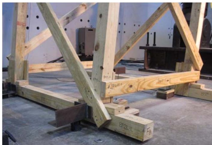
Figure 5.46 Photograph of Wedges at 15in. Displacement
