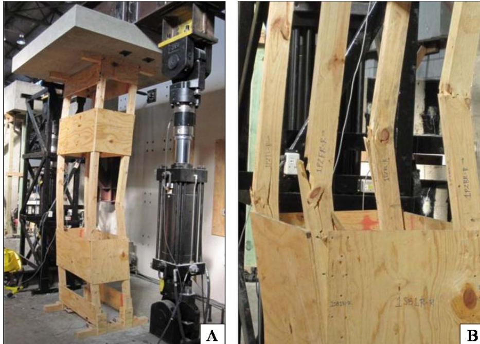
Figure 5.4 Test 1 A) First Failure and Bowing of Posts B) All Post Failures
