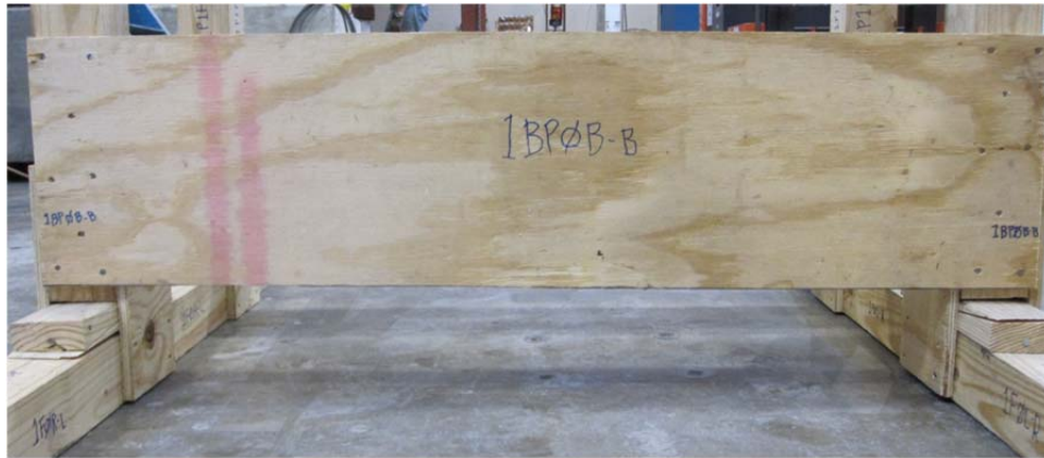
Figure 3.11 Example of a Member ID Code: Shore #1, Base Plate, Ground Level, Back Side - Facing the Back
