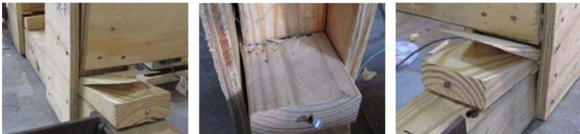
Figure 5.41 Wedge Cupping and Bearing Under Posts During Loading
