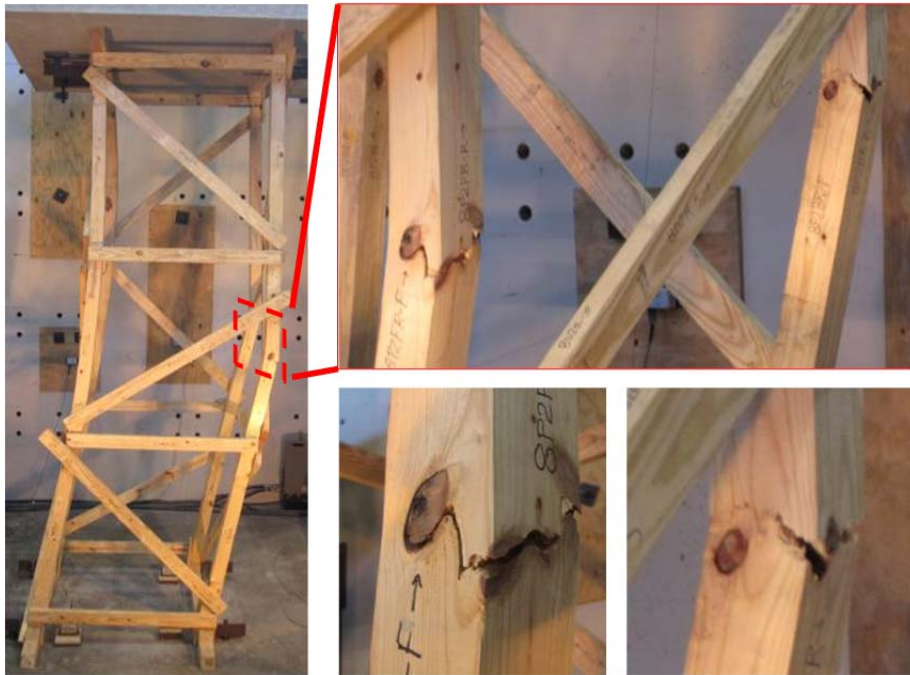
Figure 5.50 Photographs of Right Side Post Failures
