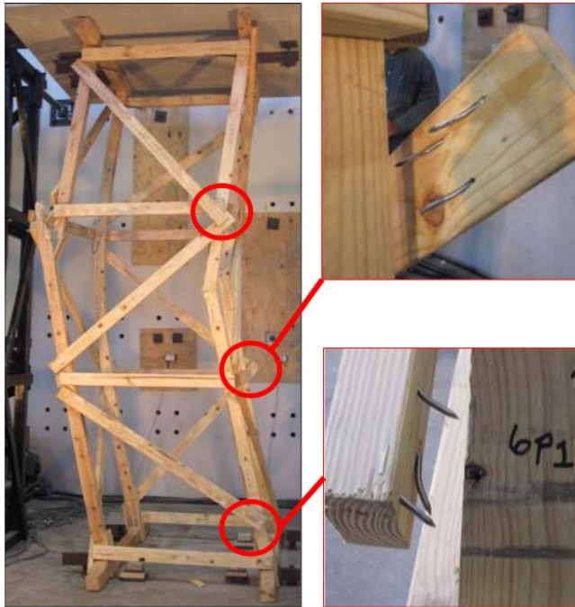
Figure 5.40 Brace Failure Locations
