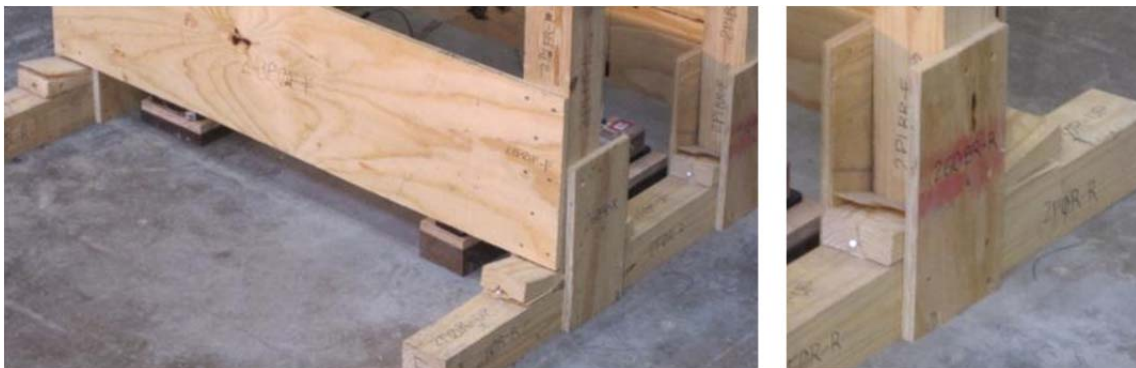
Figure 5.8 Test Specimen 2 Wedge Cupping
