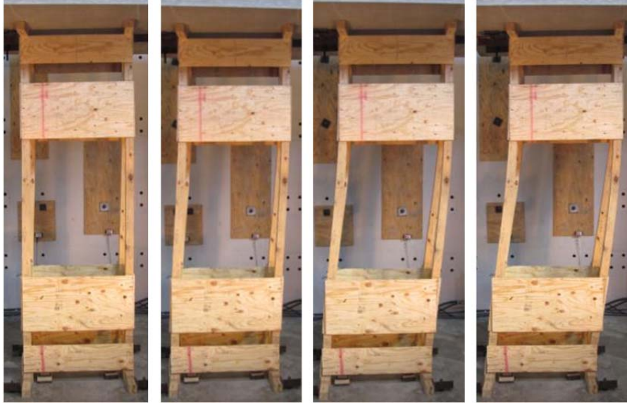
Figure 5.56 Progression of Lateral Displacement with Applied 32kip Load
