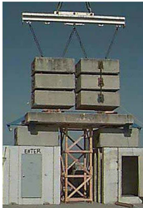
Figure 2.14 OARF Loading Apparatus ( FEMA StS2 Summary- Testing of Laced Post & Plywood Laced Posts, 2011 )
