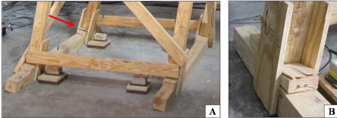
Figure 5.20 Specimen 4 Wedges A) Wedges at Failure B) Back-left Wedge Cupping
