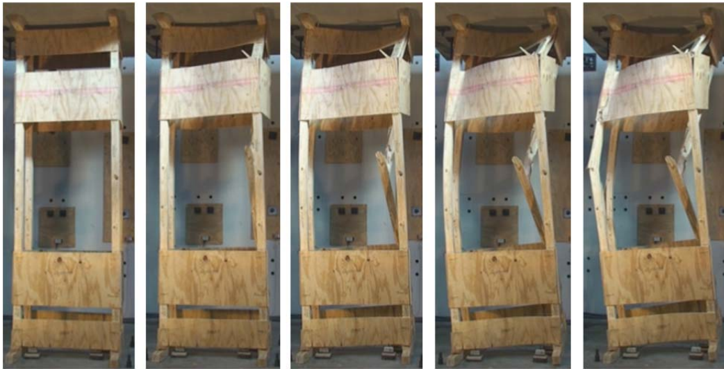
Figure 5.77 Progressive Failure of Specimen 12
