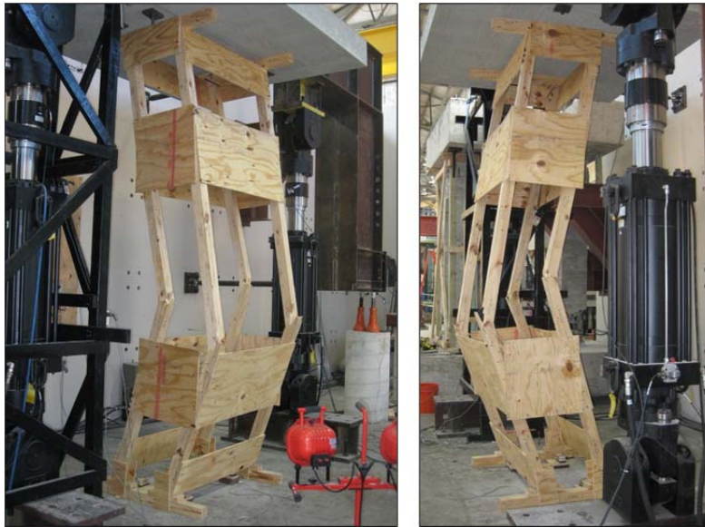
Figure 5.5 Final Failed Condition at the End of Test 1
