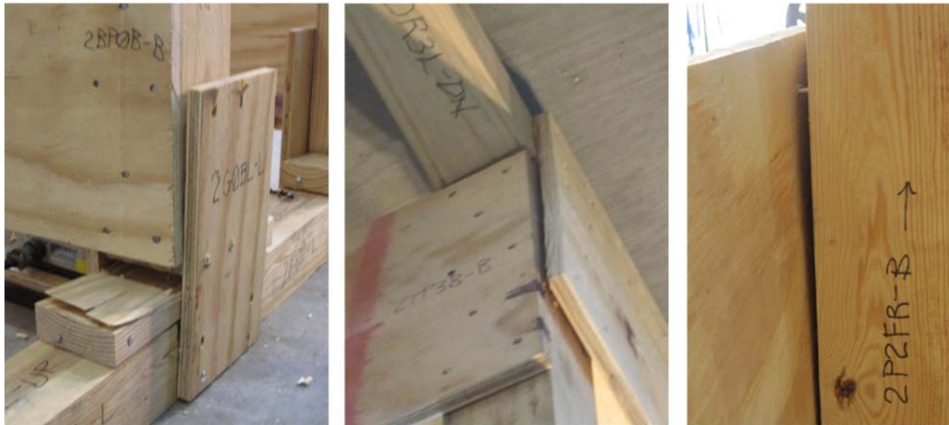
Figure 5.13 Samples of Minor Pullout from Specimen 2
