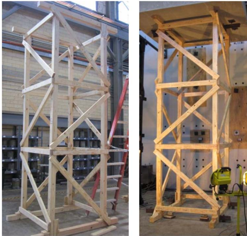
Figure 4.7 Photographs of Constructed LP Shores
