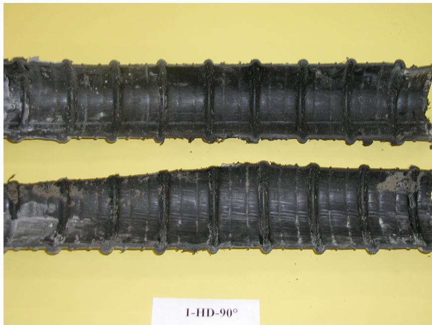
Figure 5-103 Duct from Specimen 1-HD-90° after Testing
