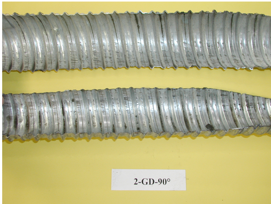
Figure 5-100 Duct from Specimen 2-GD-90° after Testing
