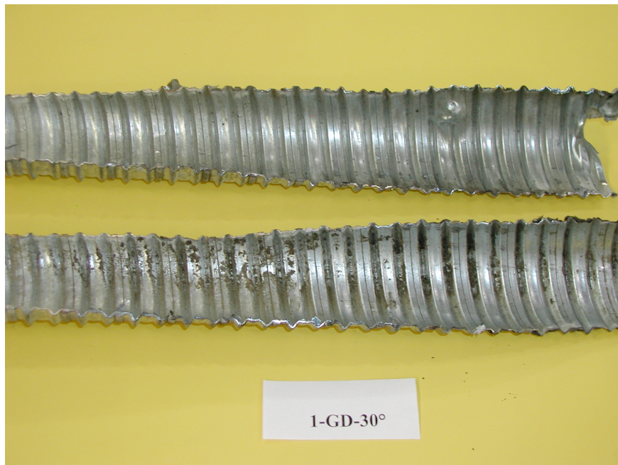
Figure 5-101 Duct from Specimen 1-GD-30° after Testing
