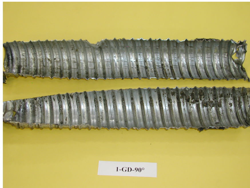
Figure 5-99 Duct from Specimen 1-GD-90° after Testing
