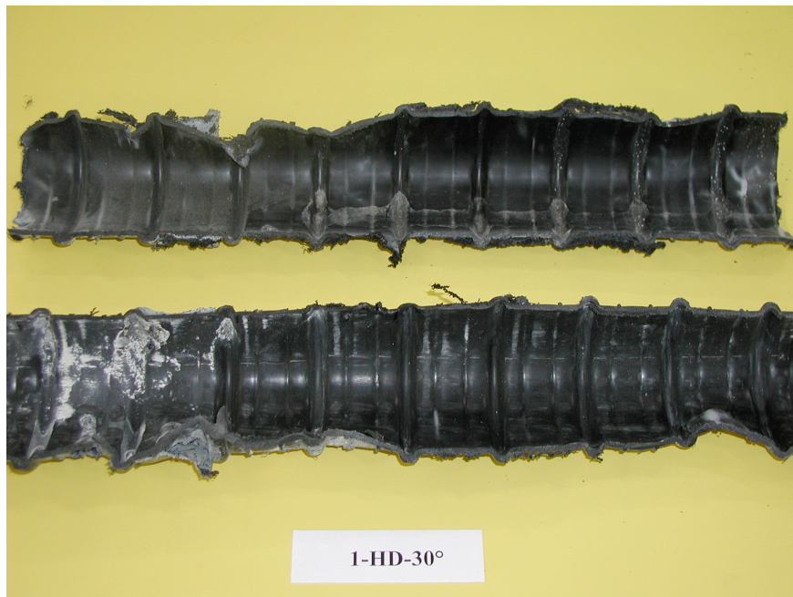
Figure 5-105 Duct from Specimen 1-HD-30° after Testing
