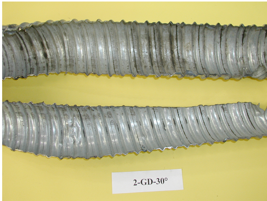
Figure 5-102 Duct from Specimen 2-GD-30° after Testing
