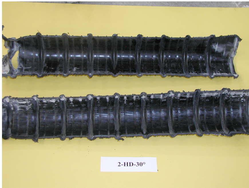
Figure 5-106 Duct from Specimen 2-HD-30° after Testing
