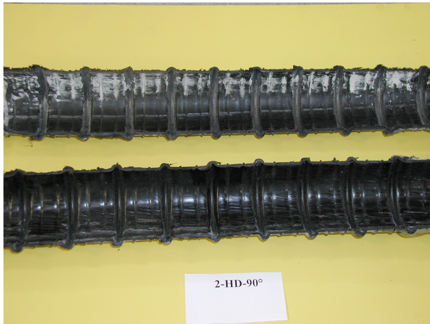
Figure 5-104 Duct from Specimen 2-HD-90° after Testing
