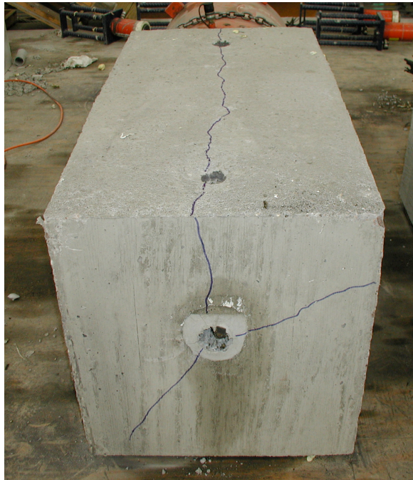
Figure 5-84 Profile of Specimen 1*-HD-7.5°-2 after Testing
