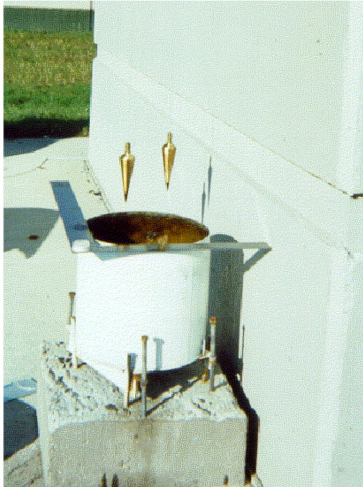
**Figure 2.8 Pier Deflection Monitoring System**
