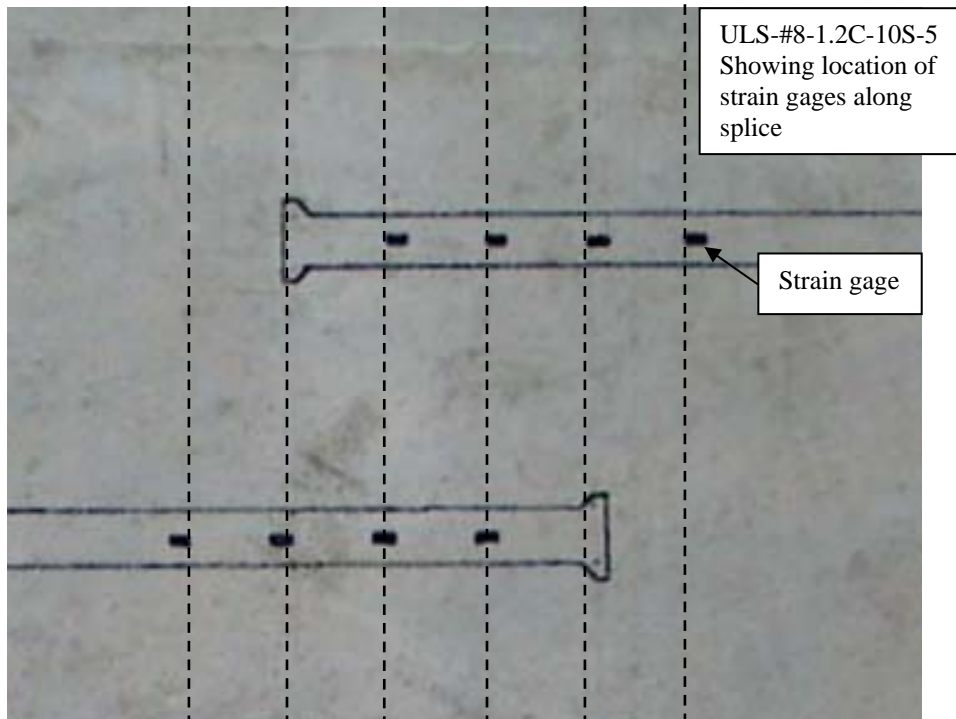
Figure 4.5 – Strain Along Splice at P = 7.2 kips b = 36 in., L_s = 5 in., s_{bar} = 10 in., Staggered Splice
