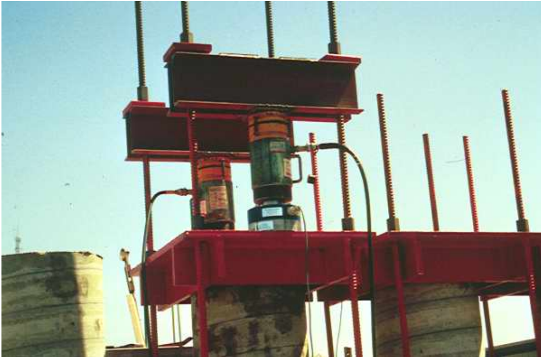
Figure 3.16: Service Load being Applied to a Column Specimen
