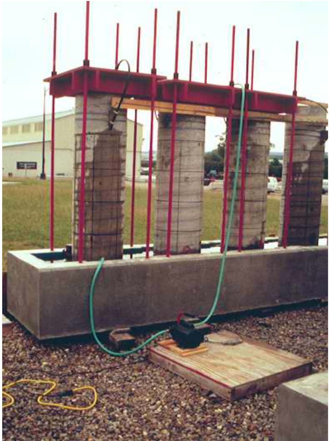
Figure 3.18: The Column Irrigation System
