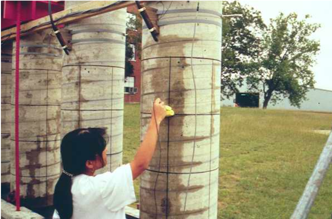
Figure 3.19: Irrigation Termination Ends and Column Gridlines
