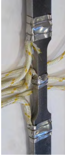
a) Shielding for middle thermocouple
