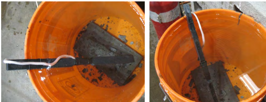
Figure 5.11 Coupons cooled in water (CIW)
