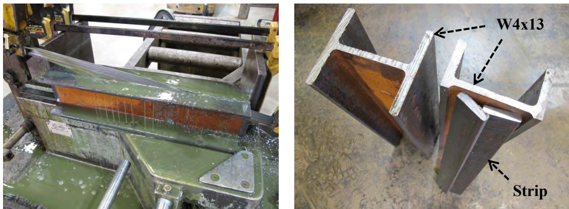
a) Flange cutting using horizontal saw
