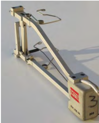
a) 2-inch extensometer for room temperature (Section 3.6.1.1)
