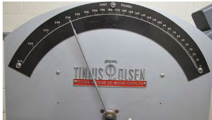
c) Reading test result off dial gauge
