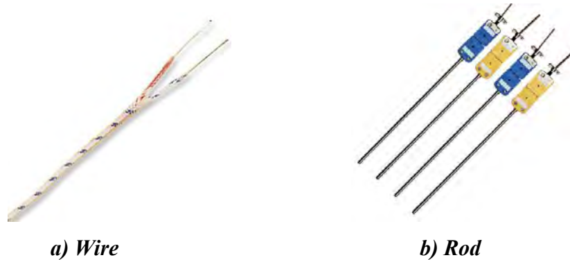
a) Wire b) Rod Figure 3.25 Forms of Type K thermocouples
