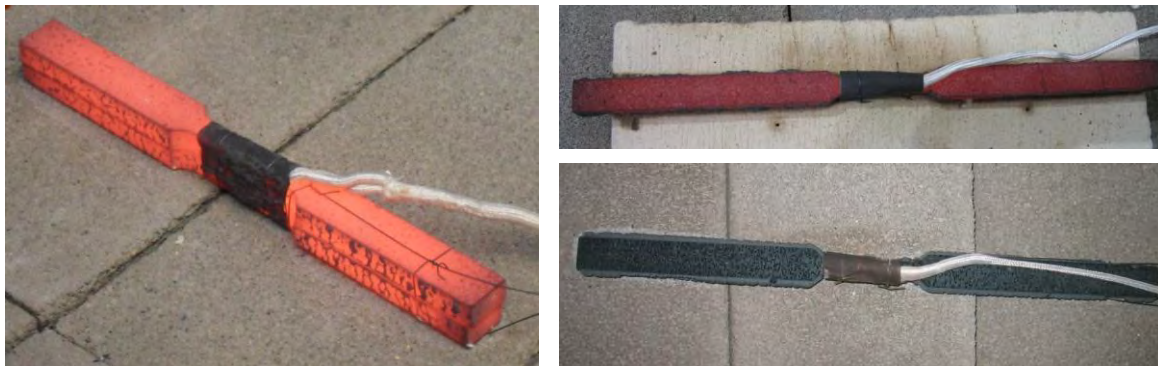
a) 14 inch coupon air-cooling
