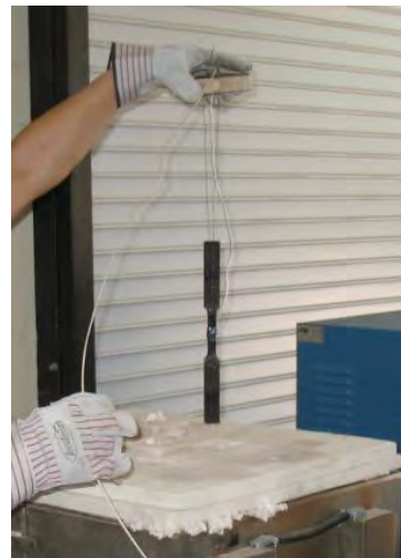
a) Coupon suspended by nickel wire b) Handled using refractory board Figure 5.3 Coupon suspension and handling scheme
