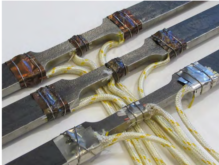
Figure 4.3 Coupon with Type K wire thermocouples
