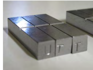
d) Completed CVN specimen
