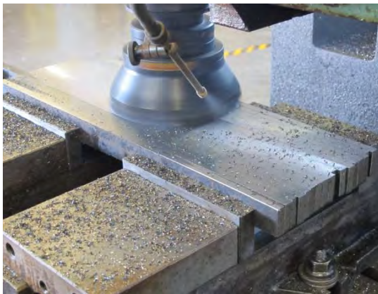
a) Strip side-milling
