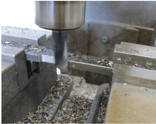
a) Cutting of specimen
