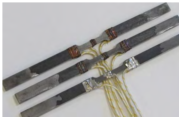
Figure 6.4 Thermocouples installed on coupons
