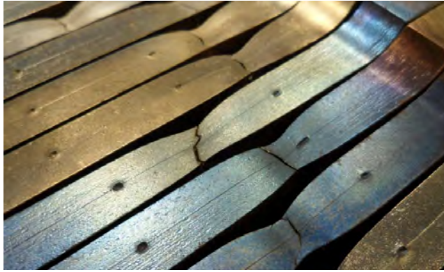
Figure 3.37 Coupons after failure requiring measurement of failure elongation
