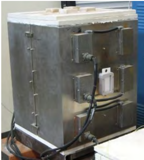
a) Exterior view b) Interior view, with three heating zones visible Figure 5.2 Furnace used for coupon heating
