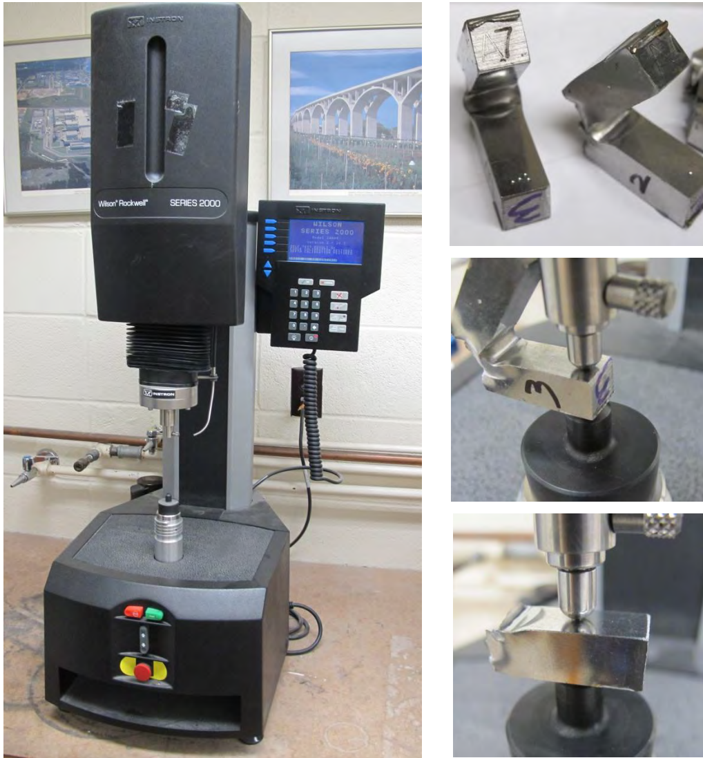
Figure 5.20 Hardness testing of previously tested CVN specimen using Wilson Rockwell machine
