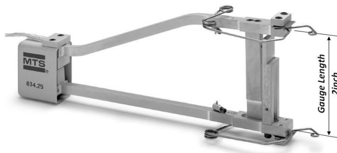
Figure 3.32 2SS extensometer (room temperature)
