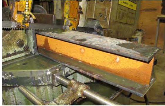
b) W4x13 rust surface
