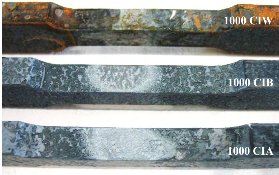
a) Coupon surface scaling, after cooling stage, for all three cases
