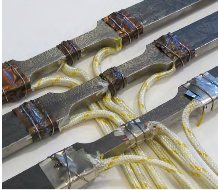
Figure 3.21 Thermocouples placement on coupon
