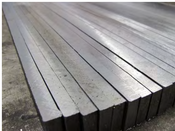
b) Completed strip side-milling
