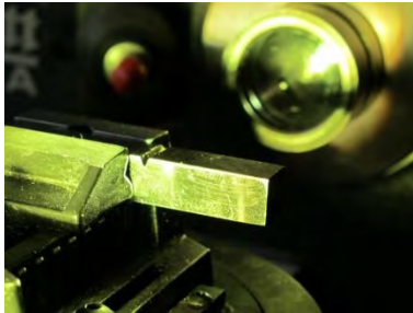
c) Examination of V-Notch dimensions
