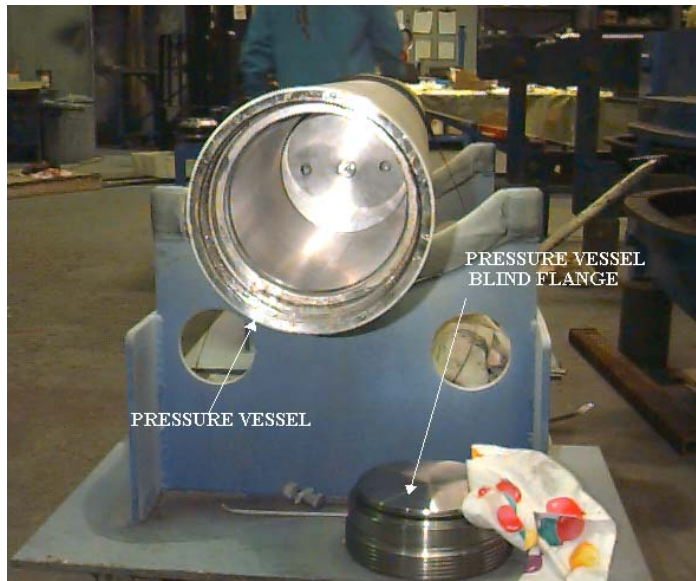
Figure 5-13: Specially Designed 90 MPa Pressure Vessel used in Explosive Decompression Testing
