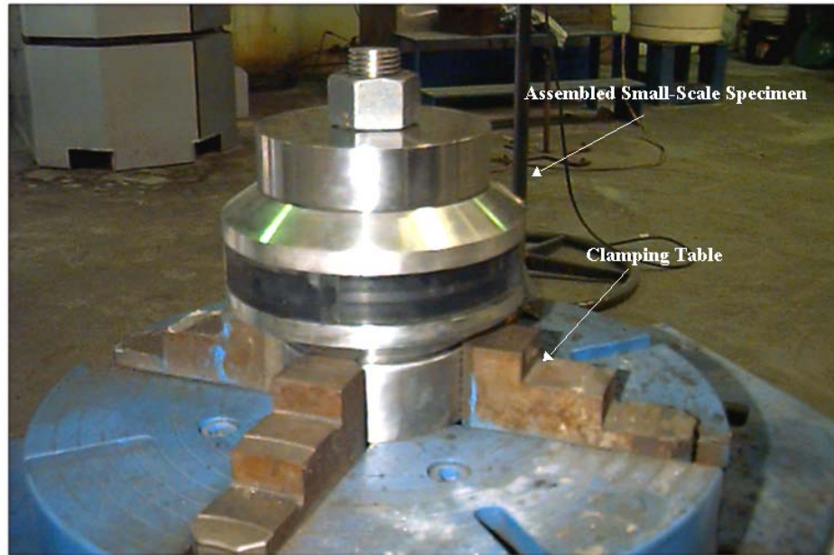
Figure 5-11: Assembled Small-Scale Test Specimen (8 mm Rubber Layer)
