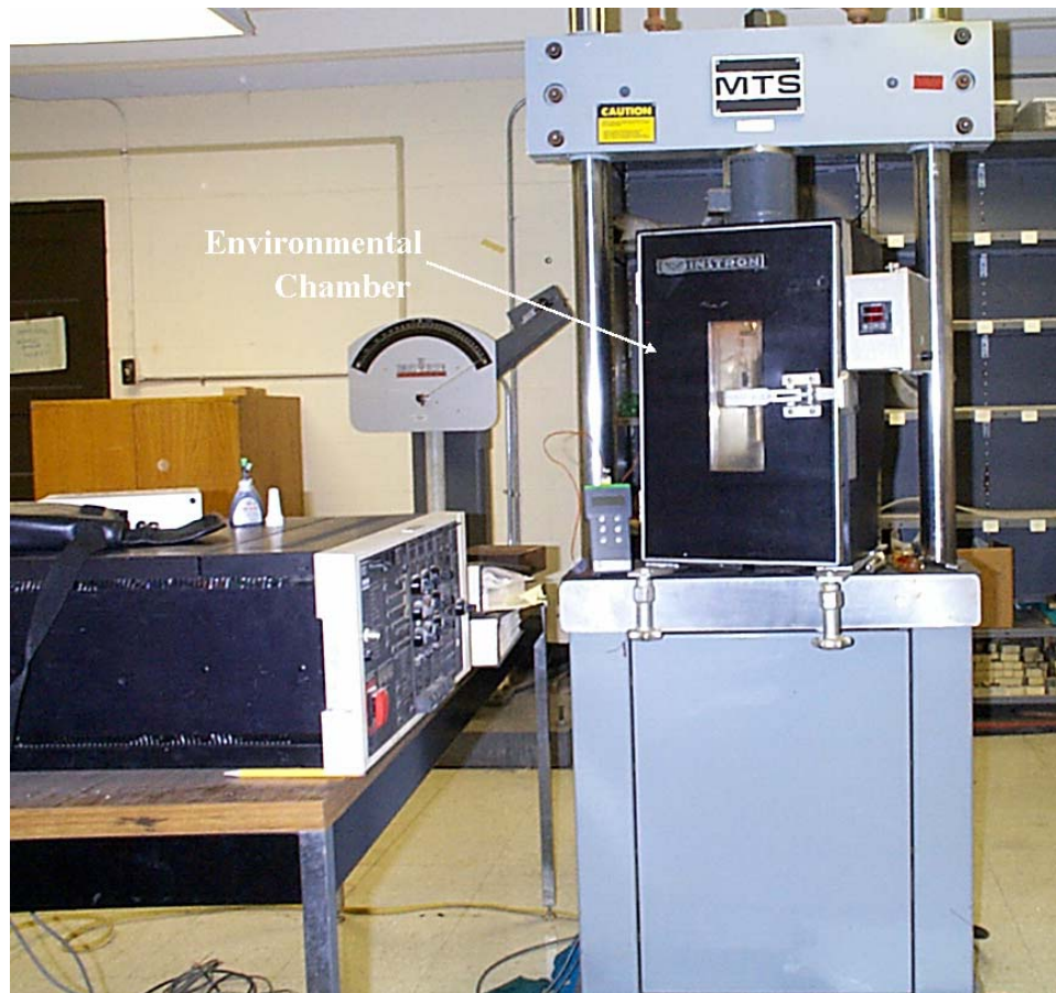
Figure 3-12: MTS System with Environmental Chamber used for Small-Scale Tests
