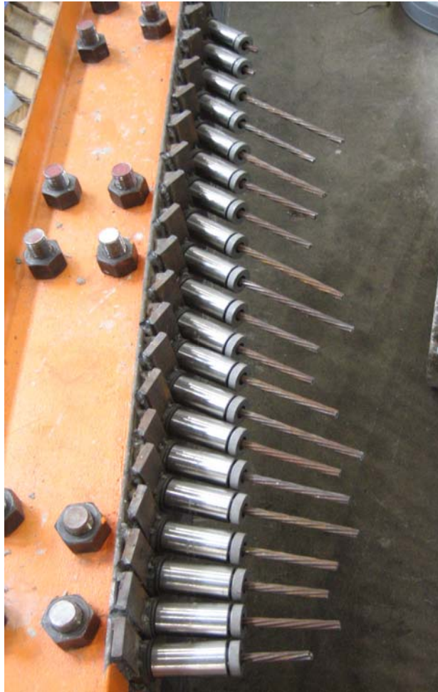
Figure 5.6: Congested dead end anchorage after stressing strands for P45F60-1
