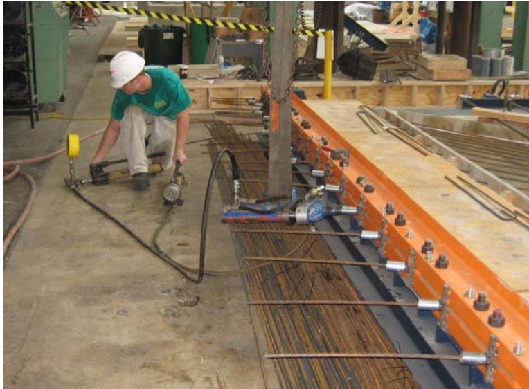
Figure 5.1: Stressing strands for panel P45F60-1
