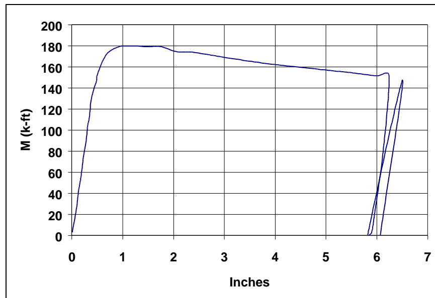
Figure 3.19 - Specimen 8.MB Load-Displacement
