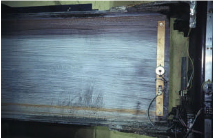
Figure 6.24 – Extent of Beam Yield at 3.5% Drift
