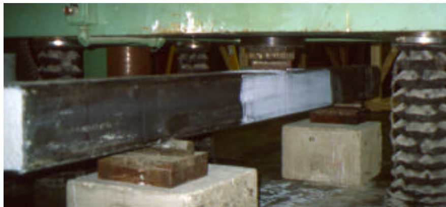
Figure 2.8 - Specimen 8.M-B Tested Under Flexure
