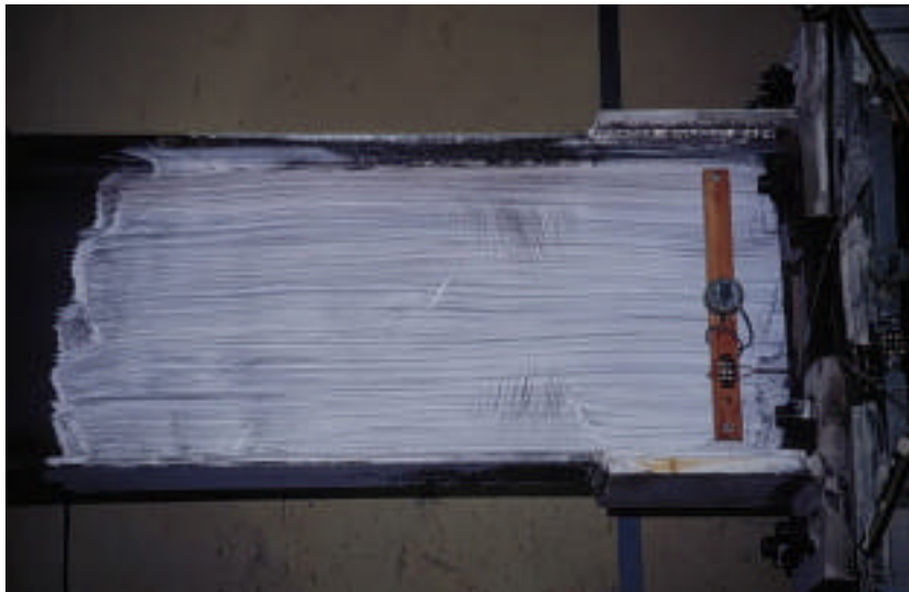
Figure 6.5 – Specimen CFT-2, Beam Web at 4.5% Drift
