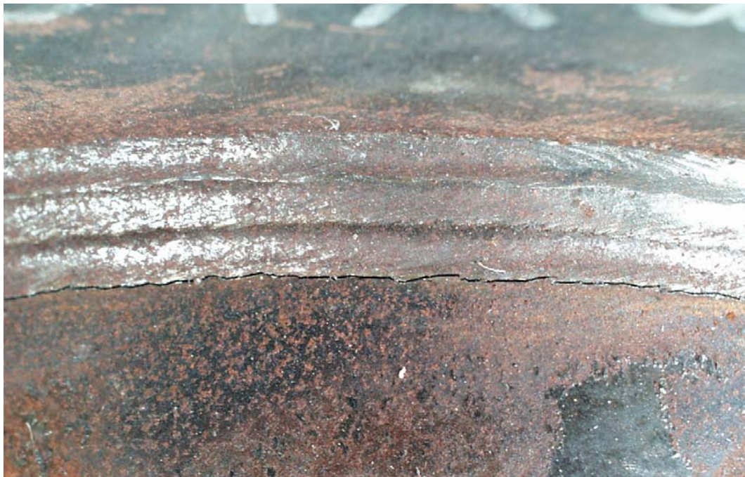
Figure 7.1 Failure of Socket Weld Connection Specimen
