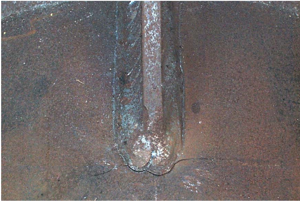
Figure 7.4 Failure of VAL 3x1/4 Specimen
