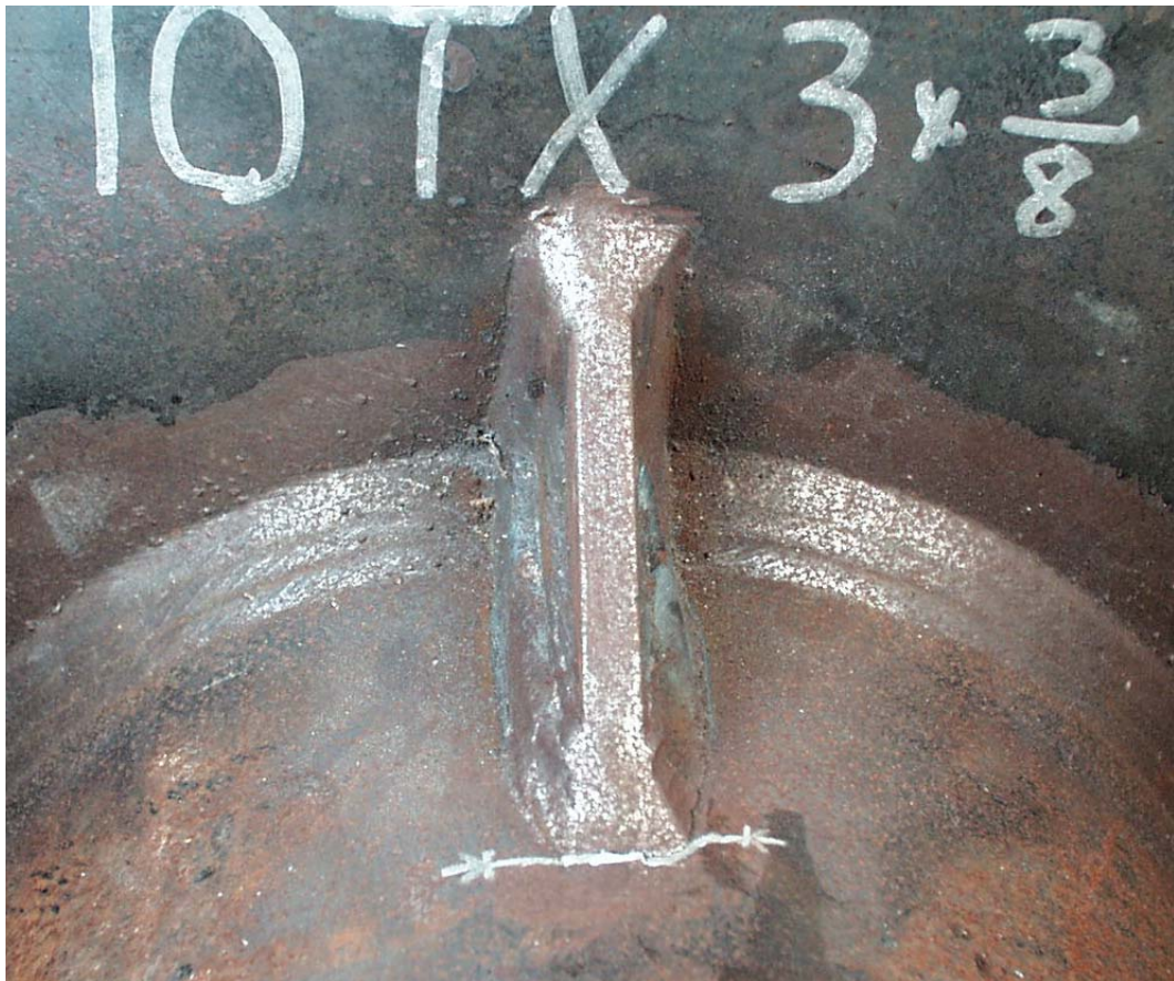
Figure 7.6 Failure of TX 3x3/8 Specimen – Note: Paint line represents extent of visible cracking.
