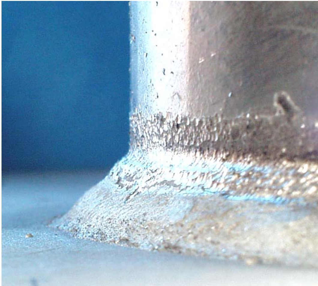
Figure 6.21 UIT Treated Region of a VALNu PR Specimen
