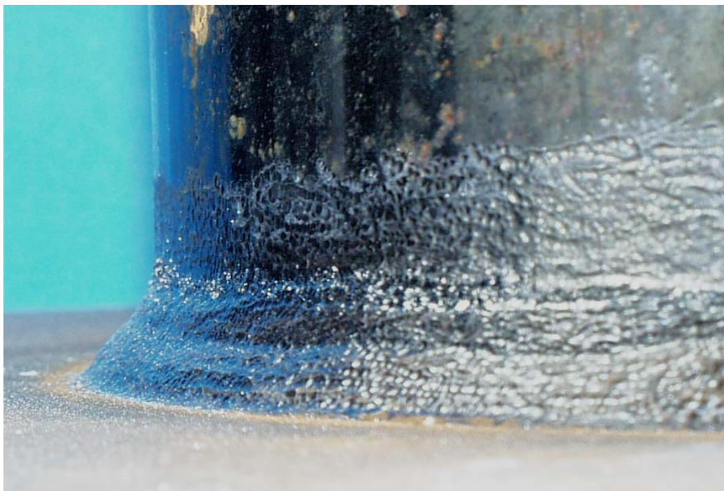
Figure 6.22 UIT Treatment of Heat Affected Region on VALNu PG Series
