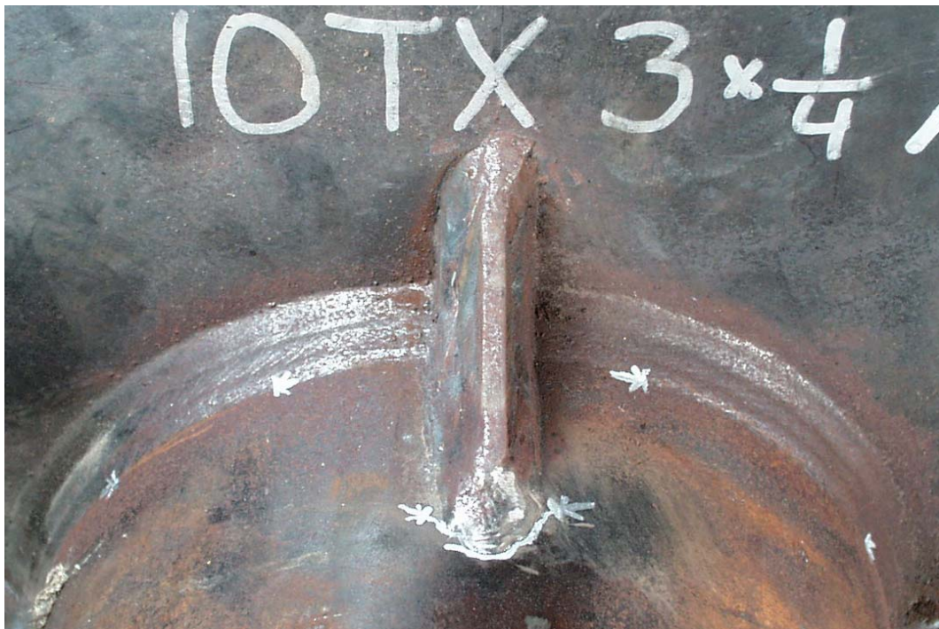
Figure 7.7 Failure of TX 3x1/4 Specimen – Note: Paint line at termination of stiffener represents extent of visible cracking, and painted arrows indicate visible crack tips in socket weld toe.
