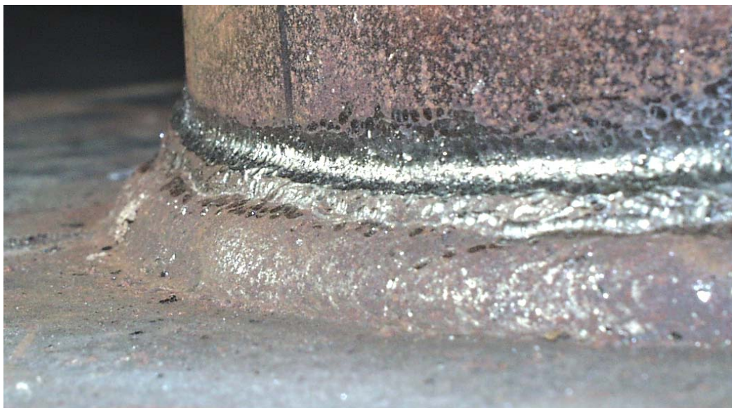
Figure 6.17 UIT Treated Socket Connection Specimen prior to testing.
