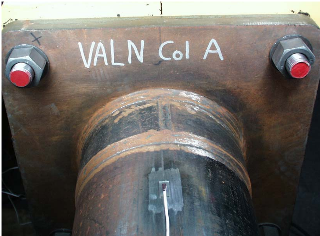
Figure 3.8 External Collar Stiffened Specimen
