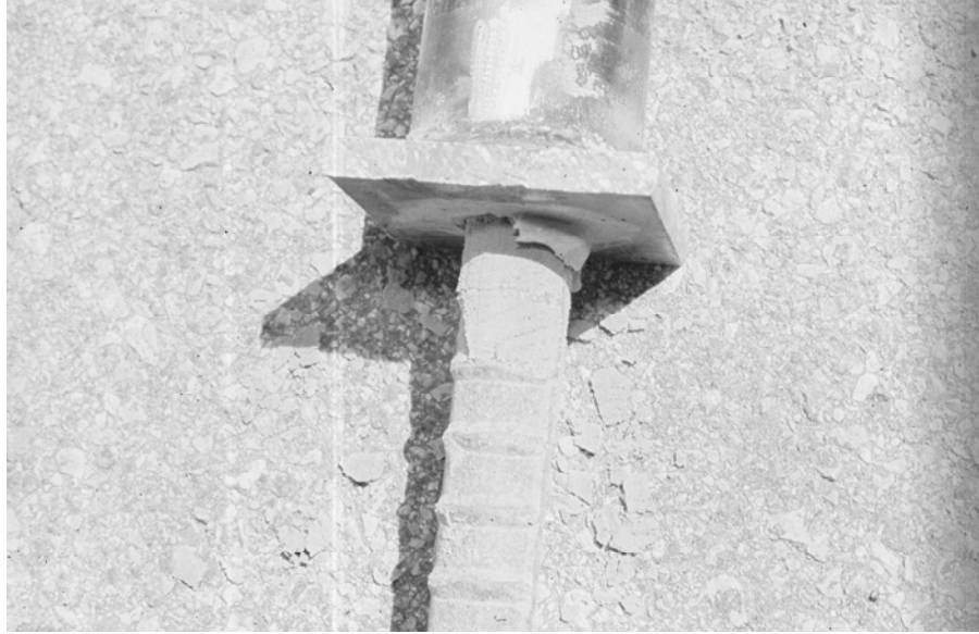
Figure 3.11: View of Spliced Bar after Testing
