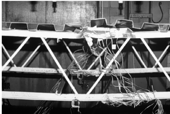
Figure 3.7 Failure Mode for 16K2-DX-1 West Joist
