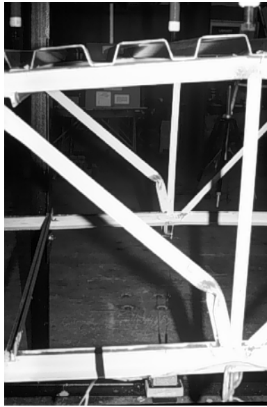
Figure 3.22 Failure Mode for 26K5-DX-2 East Joist
