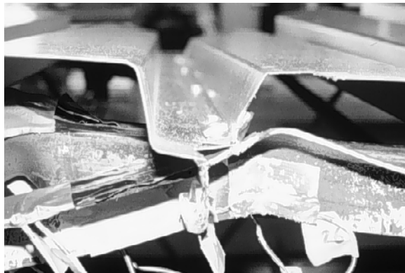
Figure 3.8 Holding Capacity of PAF through Large Deformations
