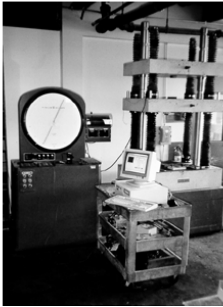
Figure 5.3 Testing Machine Used for Tension Coupons
