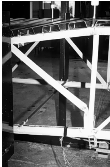
Figure 3.19 Failure Mode for 26K5-DX-1 East Joist
