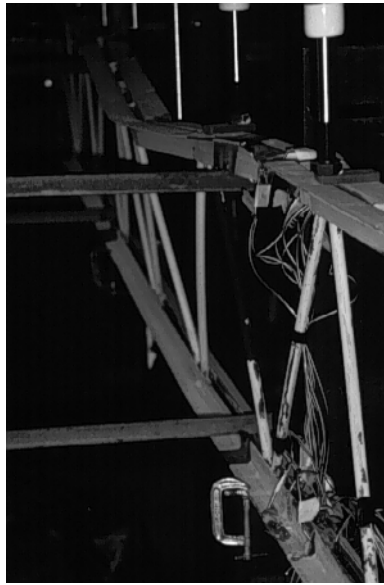
Figure 3.12 Failure Mode for 16K2-ND East Joist
