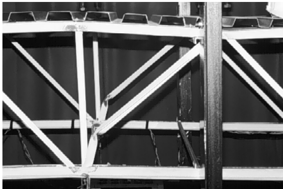
Figure 3.21 Failure Mode for 26K5-DX-2 West Joist
