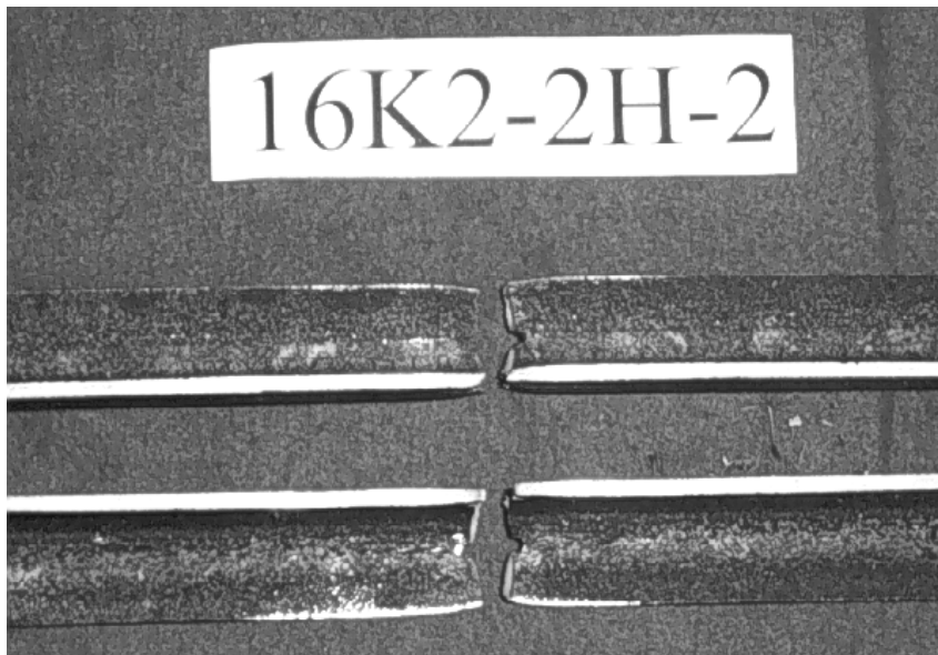
Figure 4.10 Failures in 16K2 Specimens with 2 Holes per Angle
