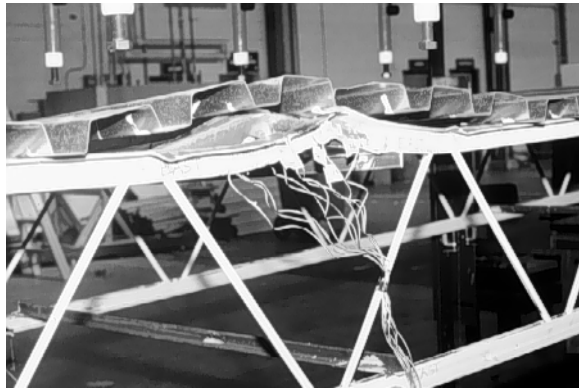
Figure 3.10 Failure Mode for 16K2-DX-2 East Joist
