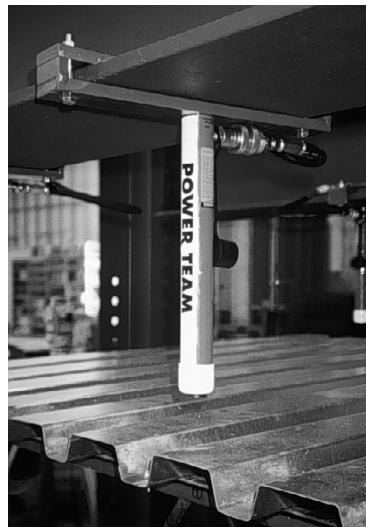
Figure 2.8 Hydraulic Ram Configuration
