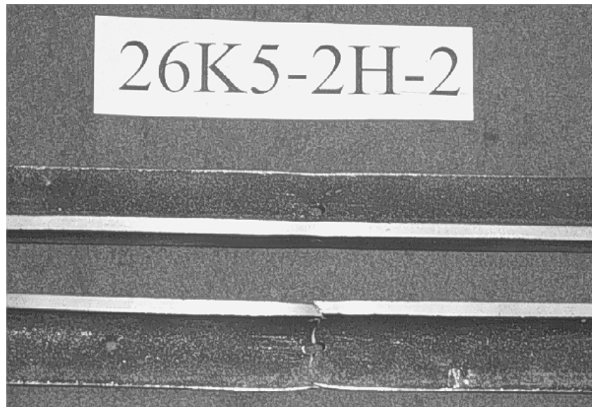
Figure 4.11 Failures in 26K5 Specimens with 2 Holes per Angle
