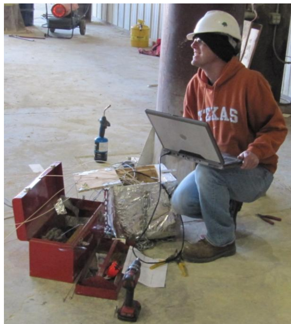
Figure 4-9: Researcher activates CompactRIO data acquisition system
