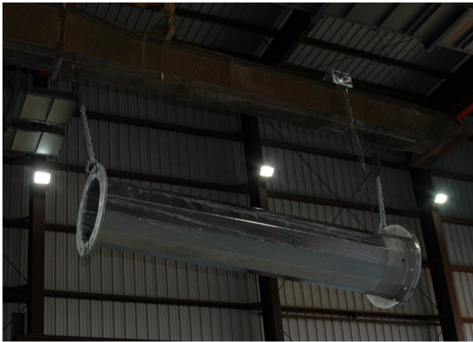
Figure 5-1: Suspended HMIP section with external collar and DAQ box after galvanizing
