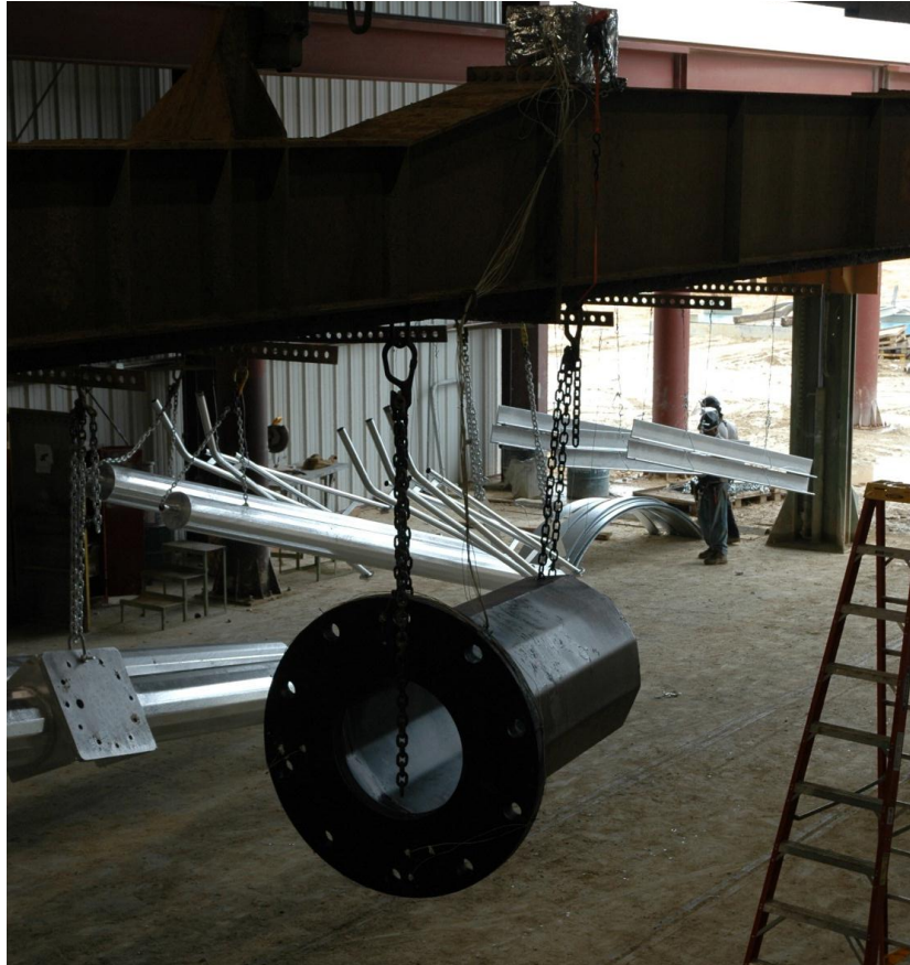
Figure 4-10: Instrumented high mast stub and DAQ box prior to galvanizing
