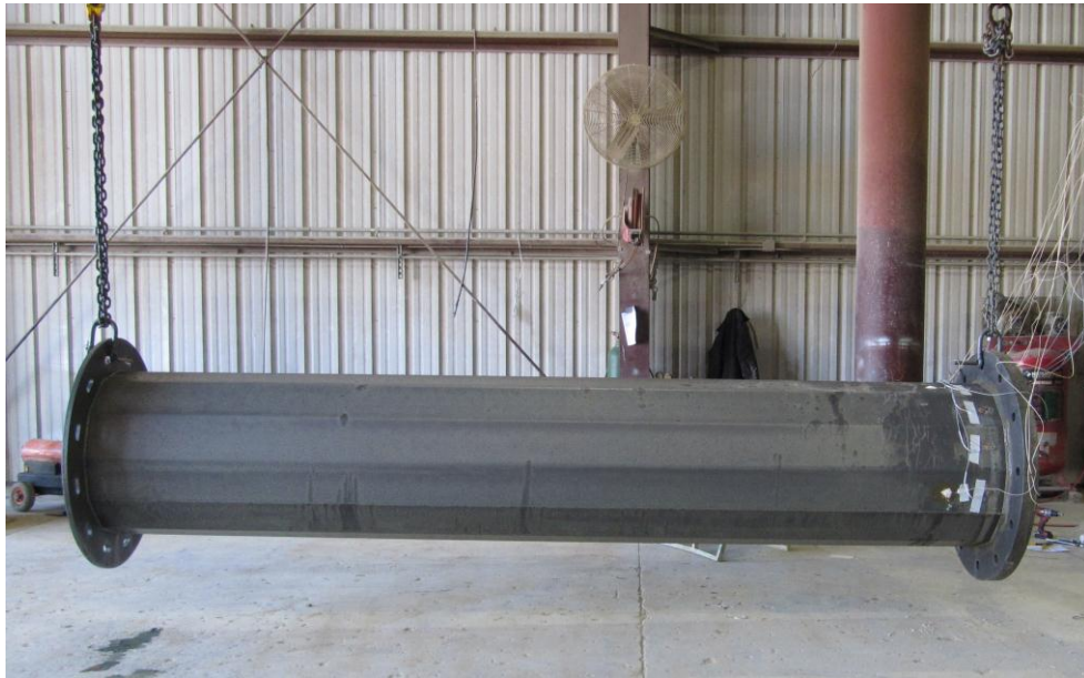
Figure 5-25: Fully instrumented HMP 33-3-12-TX-SG-C prior to galvanizing
