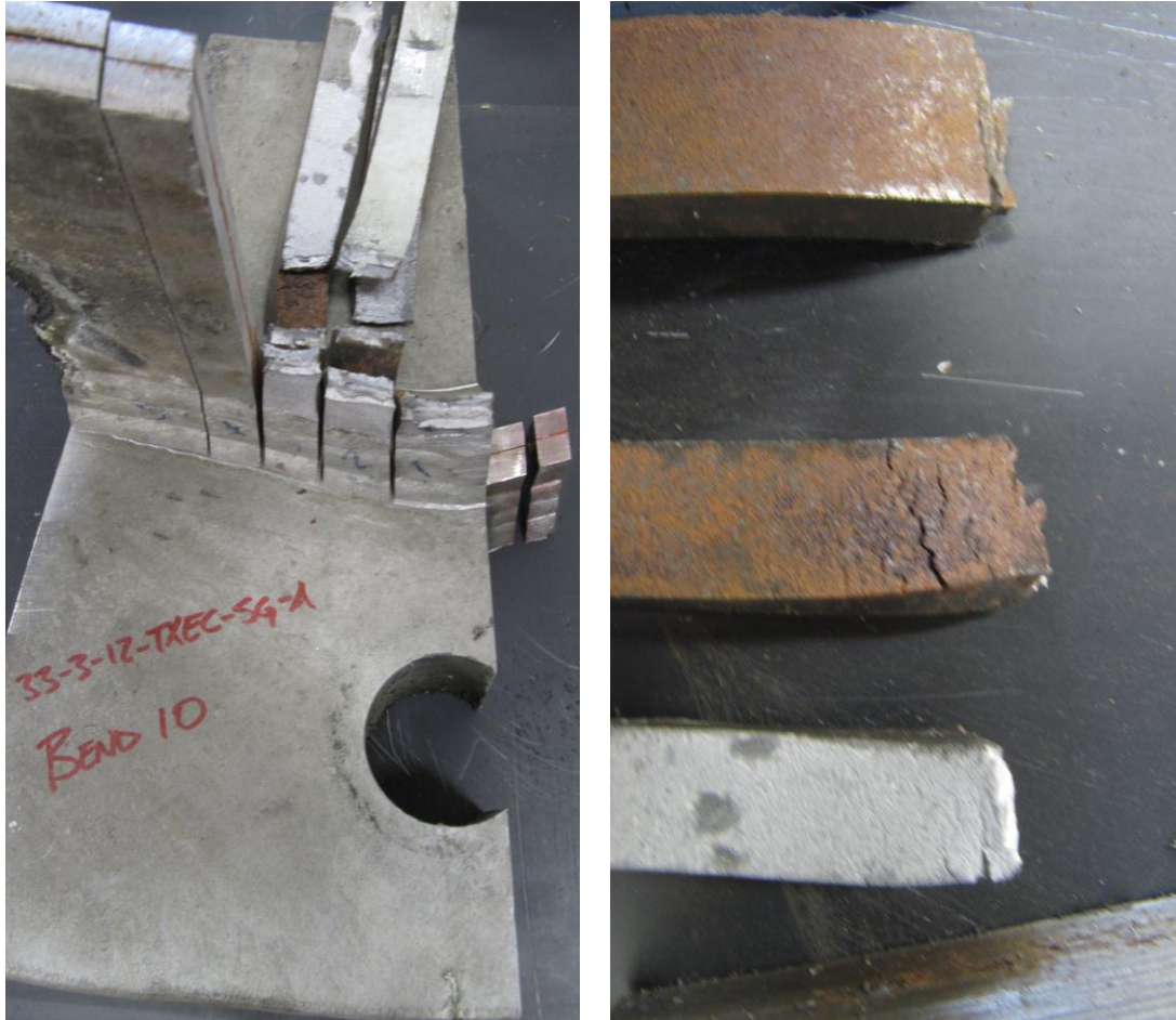
Figure 5-10: Suspected non-ductile cracks due to yielding during destructive testing
