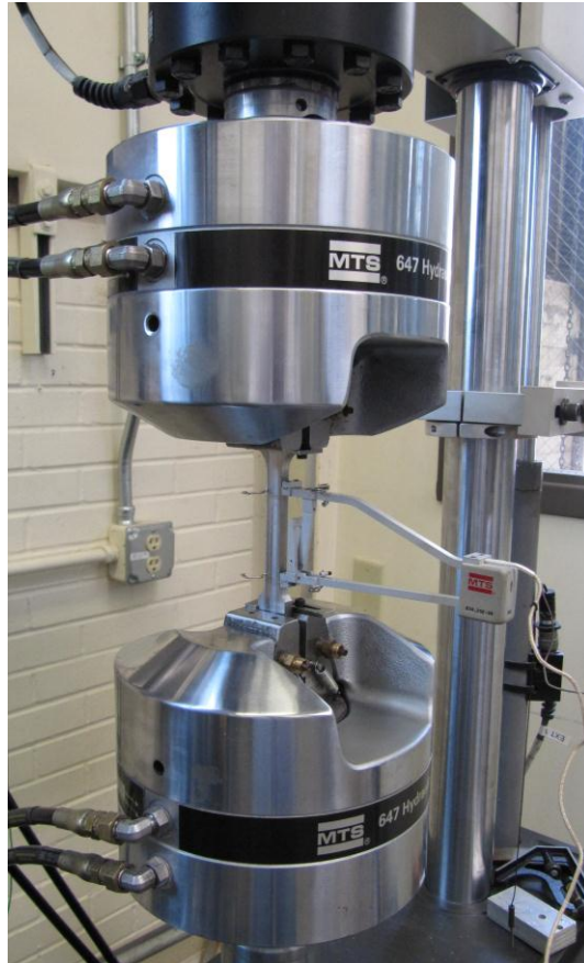
Figure 5-11: Tension coupon being tested in uniaxial tension with universal testing
