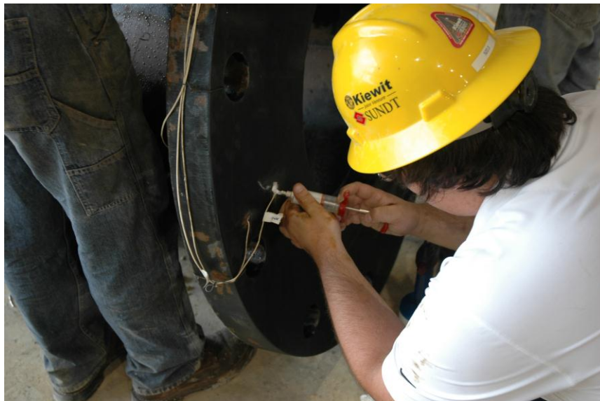
Figure 4-6: Researcher applies adhesive paste to seal thermocouple hole
