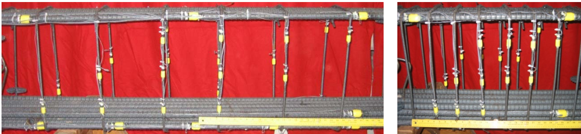
Figure A-7 Strain gage layout for a/d=3 (left) and a/d=1.5 (right)
