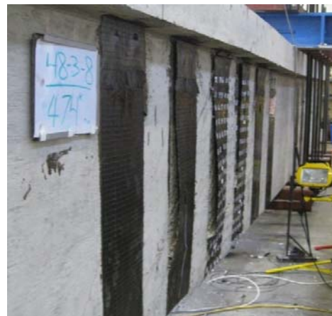
Figure 4-84 Fracture of CFRP anchors
