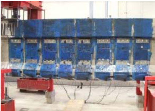
(c) Discontinuous CFRP plate
