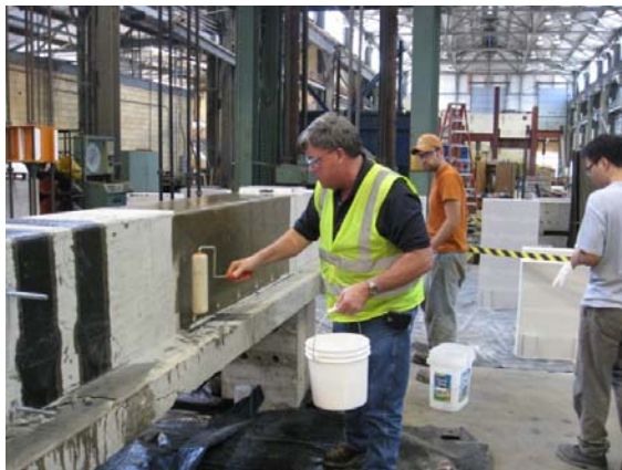
(a) Application of concrete surface primer
