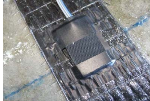
(b) Mechanical protection
