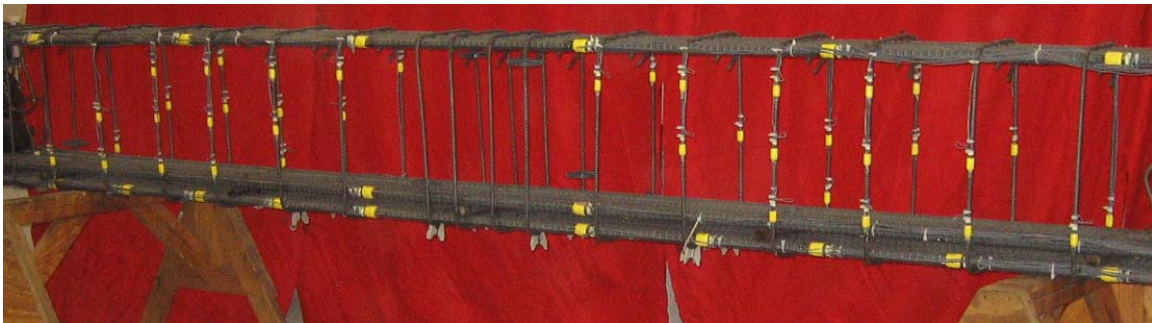
Figure A-5 16 ft. bar cage for a/d=3 (#3@10'')
