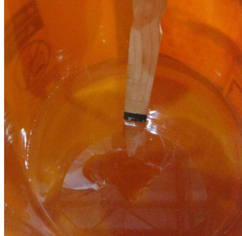
2) Measuring the epoxy resin
