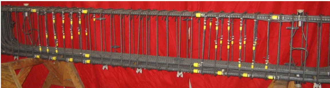
Figure A-6 12 ft. bar cage for a/d=1.5 (#3@4'')
