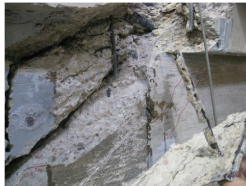
Figure 4-77 Photos of rupture of CFRP strip and anchor in test 48-3-6r
