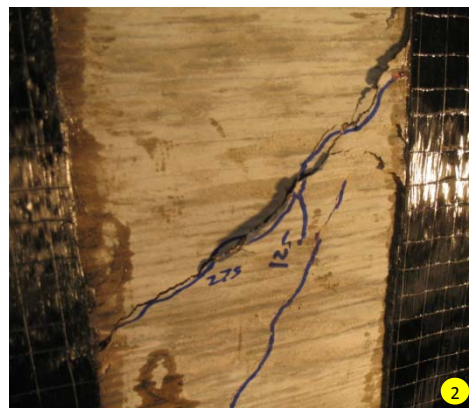
Figure 4-65 Debonding of CFRP strip of 48-3-3 at locations shown in Figure 4-64
