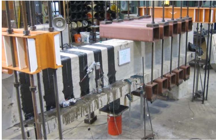
Figure 3-12 Photo of loading setup for 24 in. depth beams
