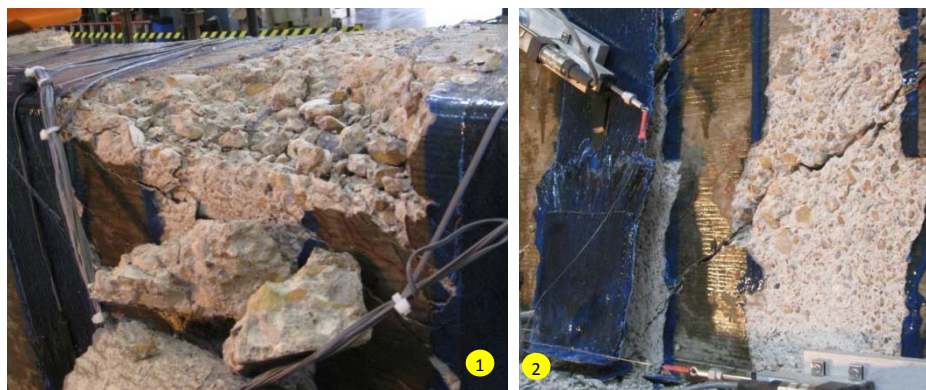
Figure 4-27 Photos of explosive rupture of strip D
