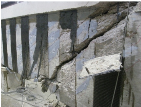
Figure 4-77 Photos of rupture of CFRP strip and anchor in test 48-3-6r
