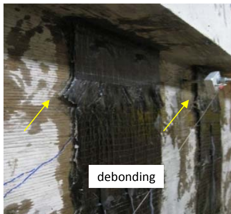
Figure 4-81 Photo of debonding of CFRP strip in test 48-3-7 when load stopped
