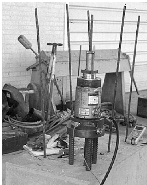
Figure 6.5- Pull-Out Block Testing Configuration
