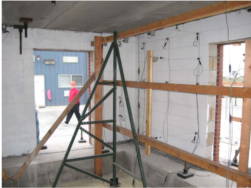
Figure 7-8 CMU wall on west side with reference frame system
