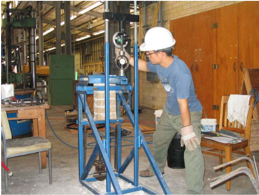
Figure 3-11 Bond-wrench testing of a typical clay masonry prism
