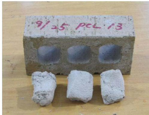
Figure 3-12 Example of loose mortar in the core-holes of clay masonry prisms laid with cement-lime mortar
