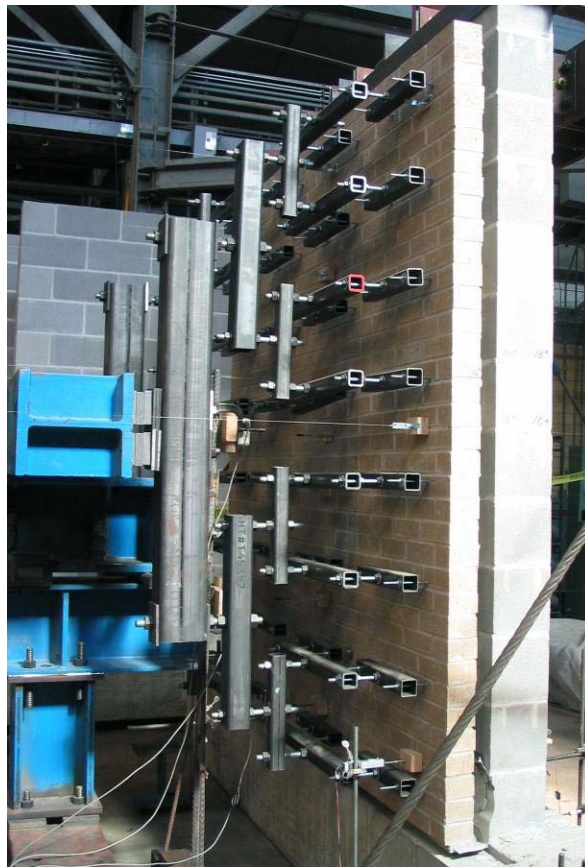
Figure 4-7 Installed "whiffle-tree" attached to CMU wall specimen
