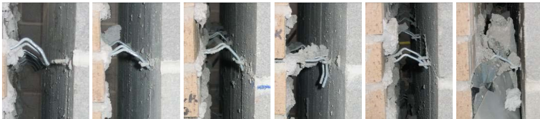
Figure 4-16 Connectors at 1-in. tensile displacement (top to bottom at west side, nearest to the viewer)
