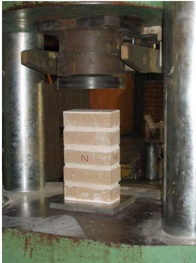
Figure 3-6 Compressive testing of a typical clay masonry prism
