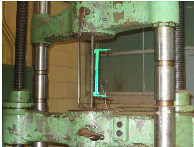
Figure 3-14 Tensile testing of a typical reinforcing bar
