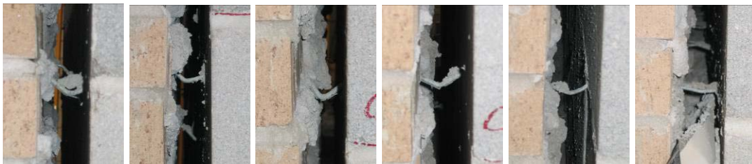
Figure 4-25 Connectors of UT CMU 2 MC at the 2 nd cycle of 0.8-in. compressive displacement (top to bottom, west side)
