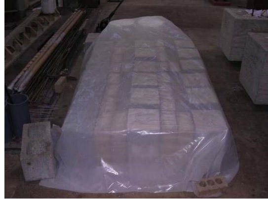
Figure 3-2 Specimens for material strength testing as cured
