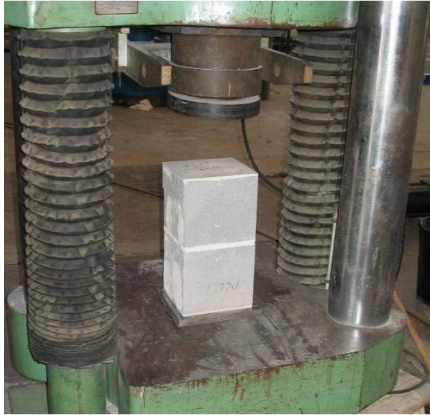
Figure 3-8 Compressive testing of a typical CMU prism
