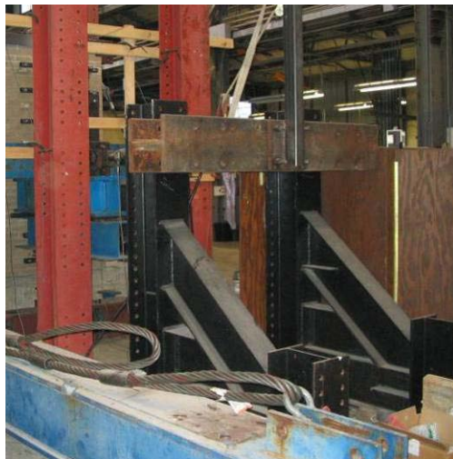
Figure 4-3 Braced loading frame of out-of-plane test setup
