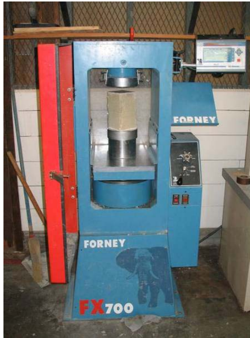
Figure 3-5 Compressive testing of a typical grout specimen
