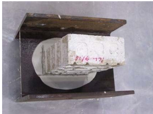
Figure 3-7 Capping of a typical clay masonry prism
