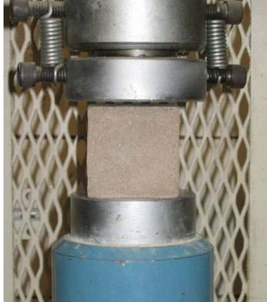
Figure 3-4 Compressive testing of a typical mortar cube
