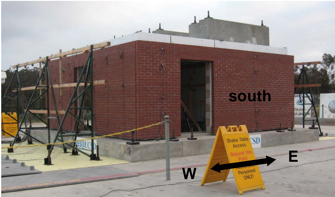
Figure 7-11 CMU building specimen on shake table
