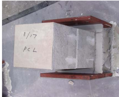
Figure 3-9 Capping of a typical CMU prism
