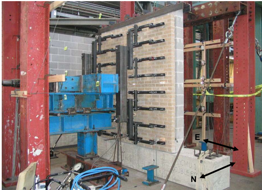
Figure 4-1 Typical quasi-static, out-of-plane CMU wall specimen (8- by 8-ft) with test setup
