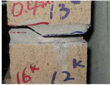
Figure 4-23 Bed joint of clay veneer at a target displacement of 0.80 in. under compressive loading of Specimen UT CMU 2 MC
