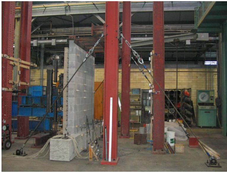
Figure 4-8 Braced reaction frame of out-of-plane test setup
