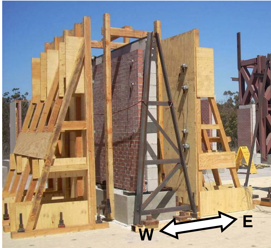
Figure 6-4 Typical shake-table, out-of-plane CMU wall specimen with test setup
