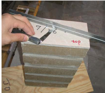
Figure 3-10 Checking the planarity of capped surfaces with a feeler gage
