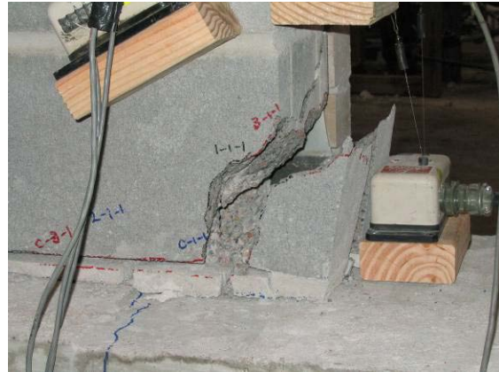
Figure 5-18 North end of CMU wall at the base under the first 1.0 in. loading to the north (Specimen UT CMU 4)
