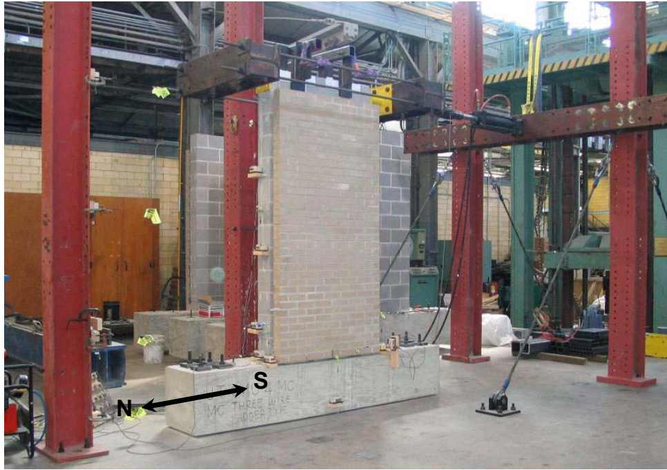
Figure 5-1 Typical quasi-static, in-plane CMU wall specimen (4- by 8-ft) with test setup
