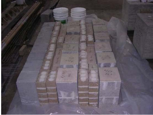
Figure 3-1 Specimens for material strength testing as constructed
