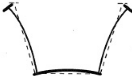
Figure 3-3: Bending distortion in unrestrained webs (Gilchrist 1997)
