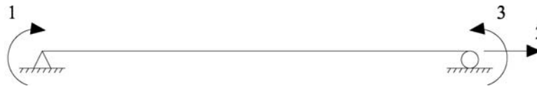
Figure A-7: Global degrees of freedom for a pin-roller simply supported beam
