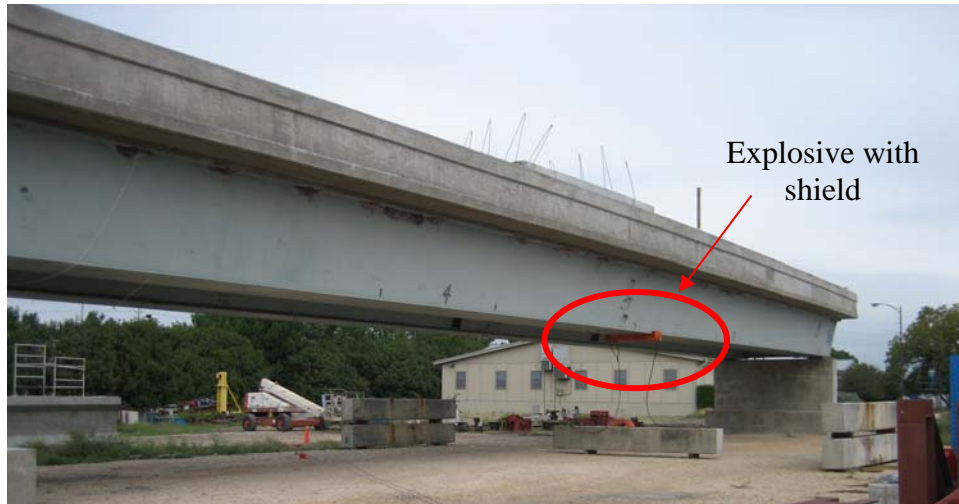
Figure 3-13: Test specimen, with containment shield in place, 21 October 2006
