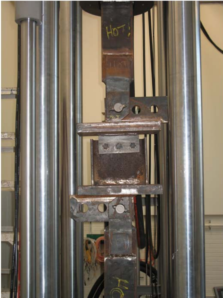
Figure 5.7 Test setup without furnace, for connections subject to tension (left) and specimens subject to inclined tension (right)
