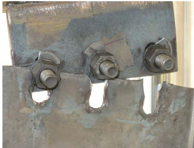
Figure 5.19 Failure shape of specimen exposed to 1000°C and subsequently cooled and tested
