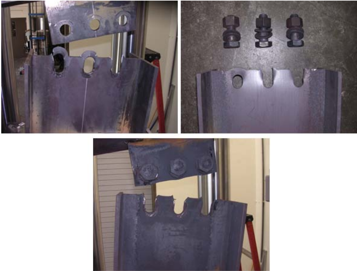
Figure 5.15 Connection failures after axial tension tests at 20° (top left), 500°C (top right) and 700°C (bottom) – W12×26 – 1 inch A325 bolts
