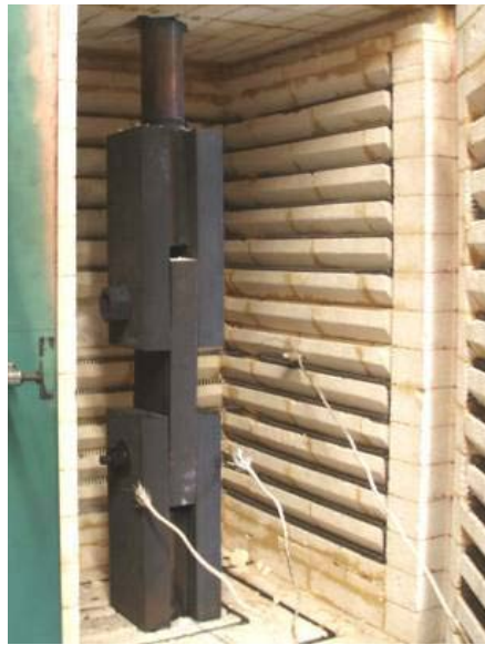
Figure 2.17 Yu's bolt shear test setup (Yu 2006)
