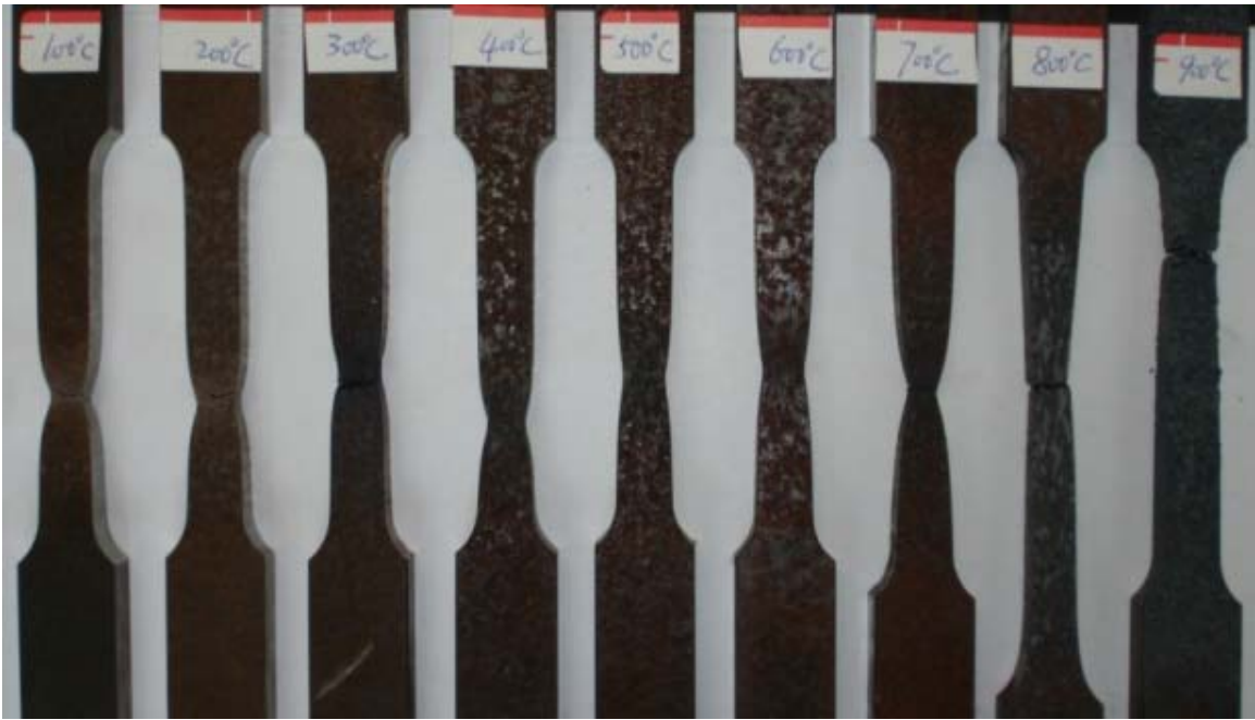
Figure 3.6 Coupons from elevated temperature tests - elongation
