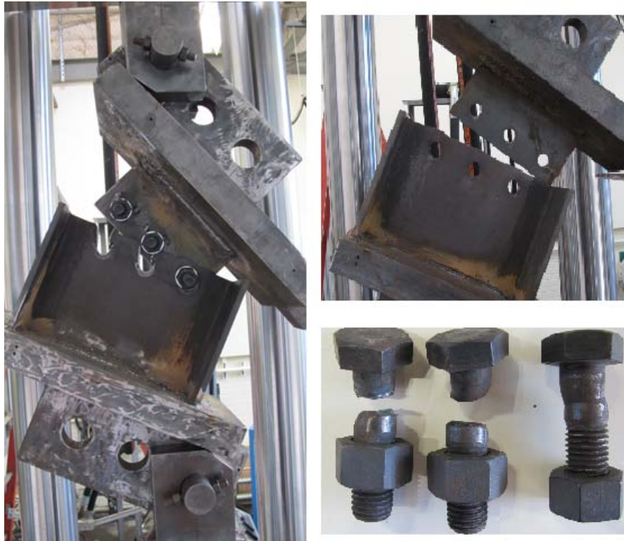
Figure 5.23 Connection failures after inclined tension tests at 20°C(left) and 400°C (right) – 3/4 inch A325 bolts
