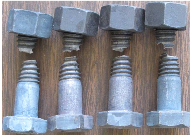
Figure 5.20 Bolts fracture in tensile test after exposure to high temperatures (900°C- left two; 1000°C-right two) and cooling
