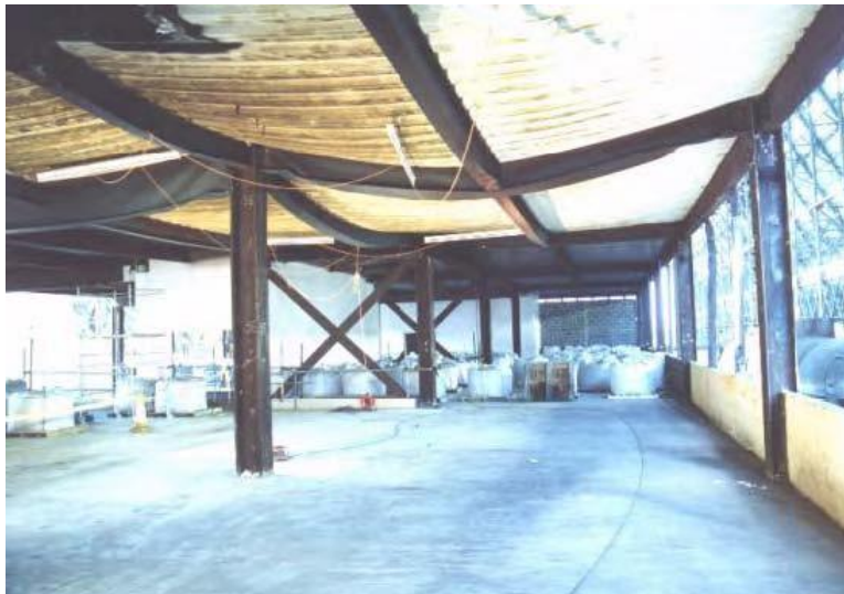
Figure 1.1 Floor system response in Cardington fire test (Cardington test report 2003)
