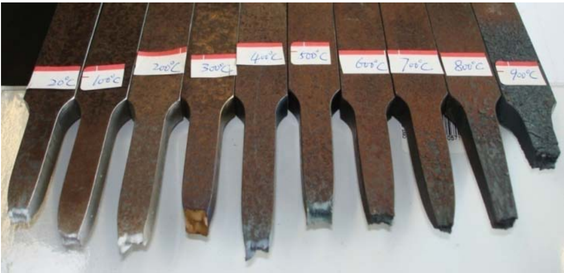
Figure 3.7 Coupons from elevated temperature tests - fracture section
