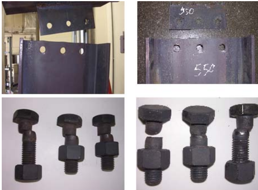
Figure 5.12 Connection failures after axial tension tests at 500°C (left) and 550°C (right) – W12×26 – 3/4 inch A325 bolts
