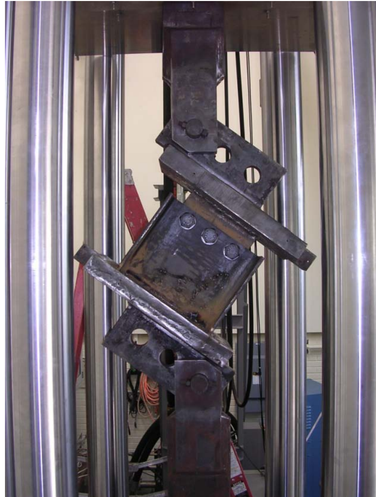
Figure 5.7 Test setup without furnace, for connections subject to tension (left) and specimens subject to inclined tension (right)
