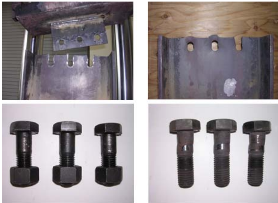
Figure 5.11 Connection failures after axial tension tests at 20°C (left) and 400°C (right) – W12×26 – 3/4 inch A325 bolts
