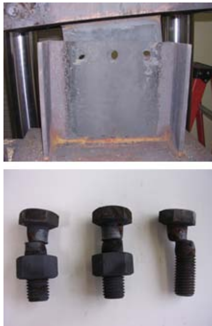
Figure 5.13 Connection failure after axial tension test at 700°C – W12×26 – 3/4 inch A325 bolts
