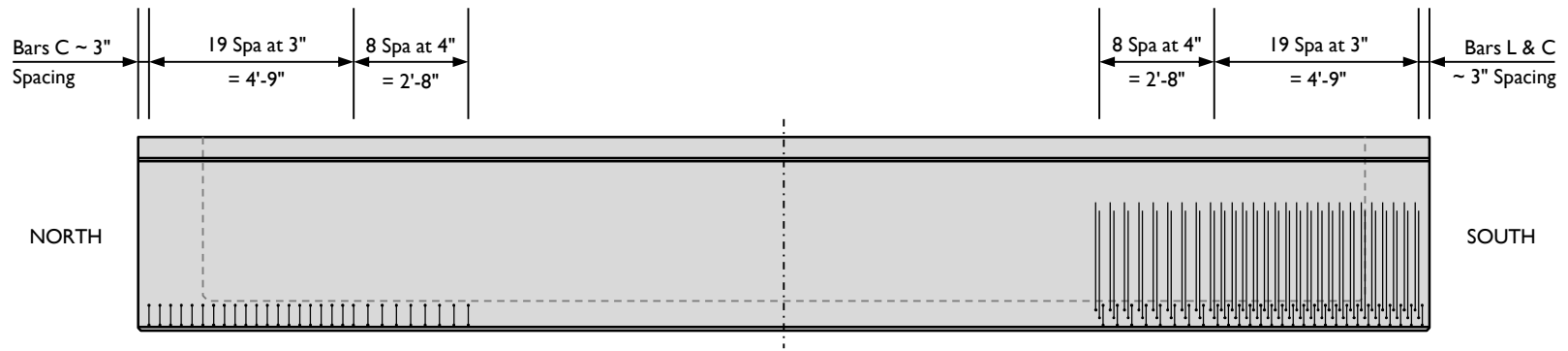
ELEVATION VIEW – Beam 4 Supplementary Reinforcement
