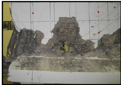
(A) Horizontal shear with web crushing in PCI BT-63 (Kuchma & Hawkins, 2007)
