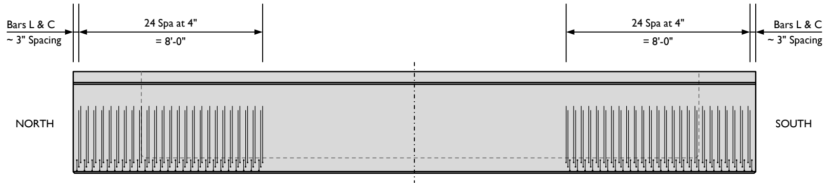
ELEVATION VIEW – Beam 6 Supplementary Reinforcement
