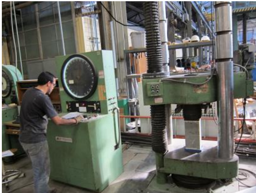
Figure 4-13 Compressive strength testing of masonry prisms
