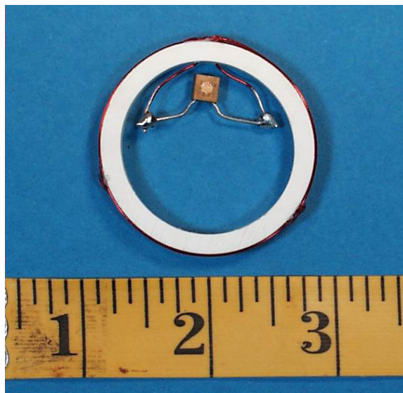
Figure C.9. Coil to Capacitor Connections
