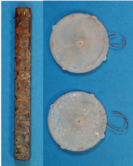
Figure D.17 Bar #25, No. 26 Gauge Wire, Exposed Loop
