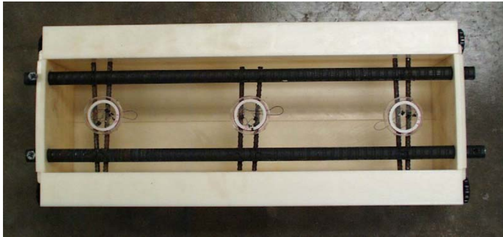
Figure 4.6 Photograph of Form, Reinforcement, and Sensors
