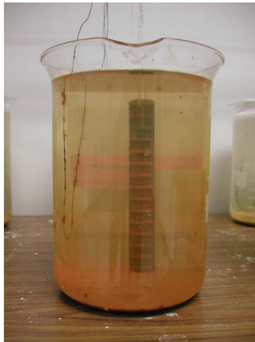
Figure 3.4 Rebar and Wire in Accelerated Corrosion Test Beaker
