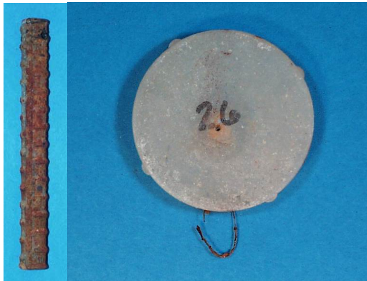
Figure D.18 Bar #26, No. 26 Gauge Wire, Exposed Loop
