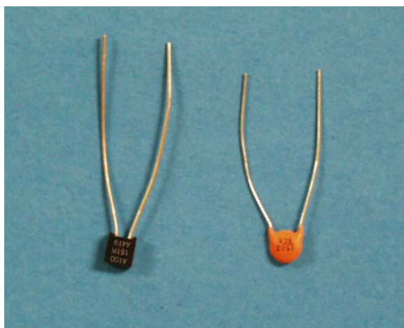
Figure C.1. Typical 151-pF Capacitors Used in Prototype Sensor
