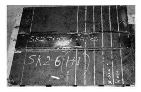
Figure 2.2: Strips marked on test plate
