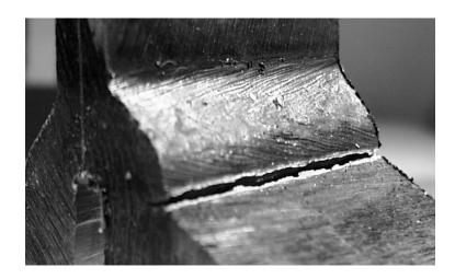
Figure 3.16. Toe crack
