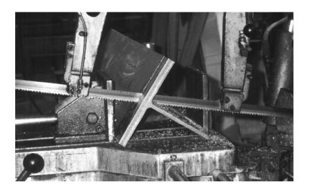
Figure 3.3. Saw-cutting T specimens
