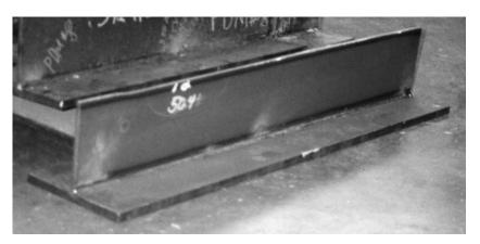
Figure 3.1. T specimens as fabricated
