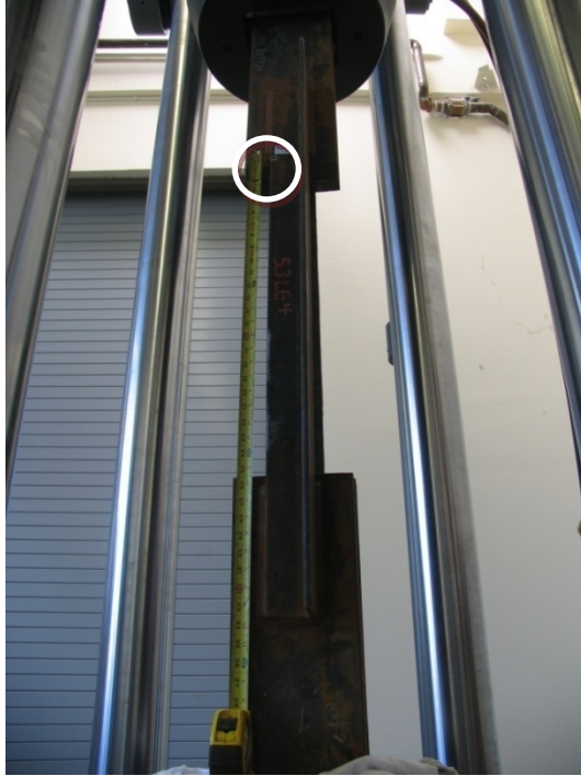
Figure 50. 53LE Angle Failure
