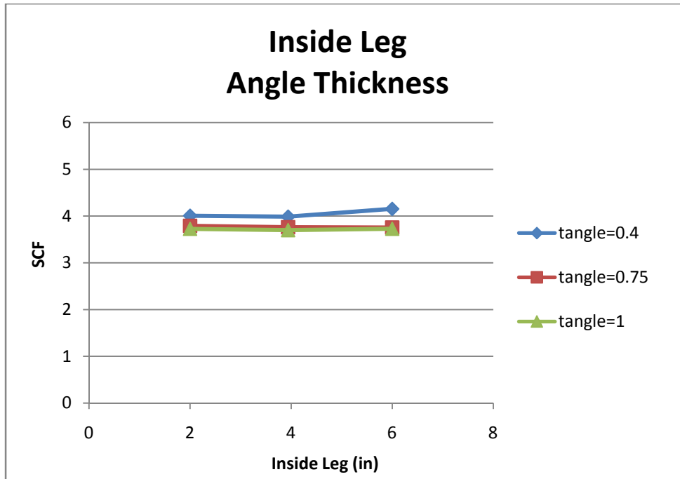
Figure 107. Inside Leg Length and Angle Thickness vs. Stress Concentration Factor
