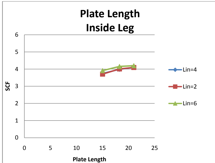
Figure 112. Plate Length and Inside Leg Length vs. Stress Concentration Factor
