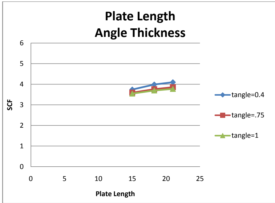
Figure 109. Plate Length and Angle Thickness vs. Stress Concentration Factor
