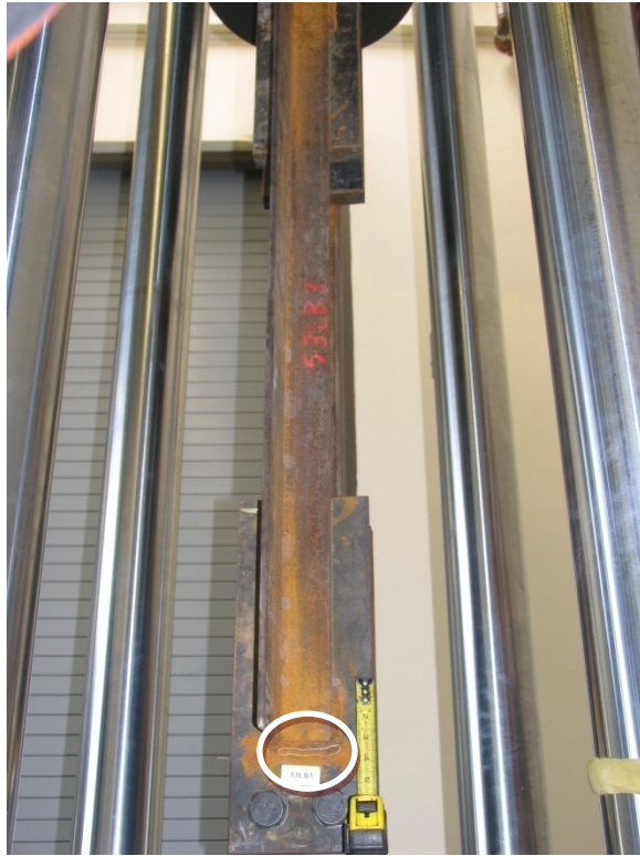
Figure 52. 53LB Angle failure
