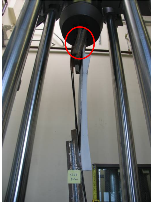
Figure 30. Failed Specimen (failure is circled)
