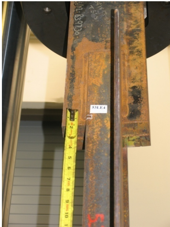
Figure 51. 53LE Angle Failure Close-Up
