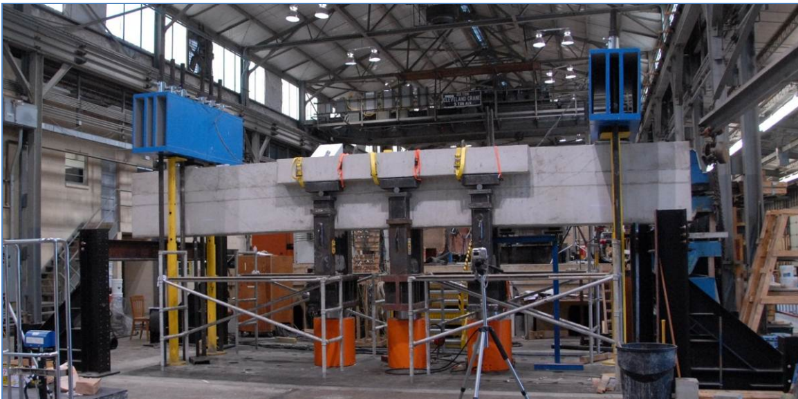
Figure 3-18: Beam specimen in test set-up with three point loads
