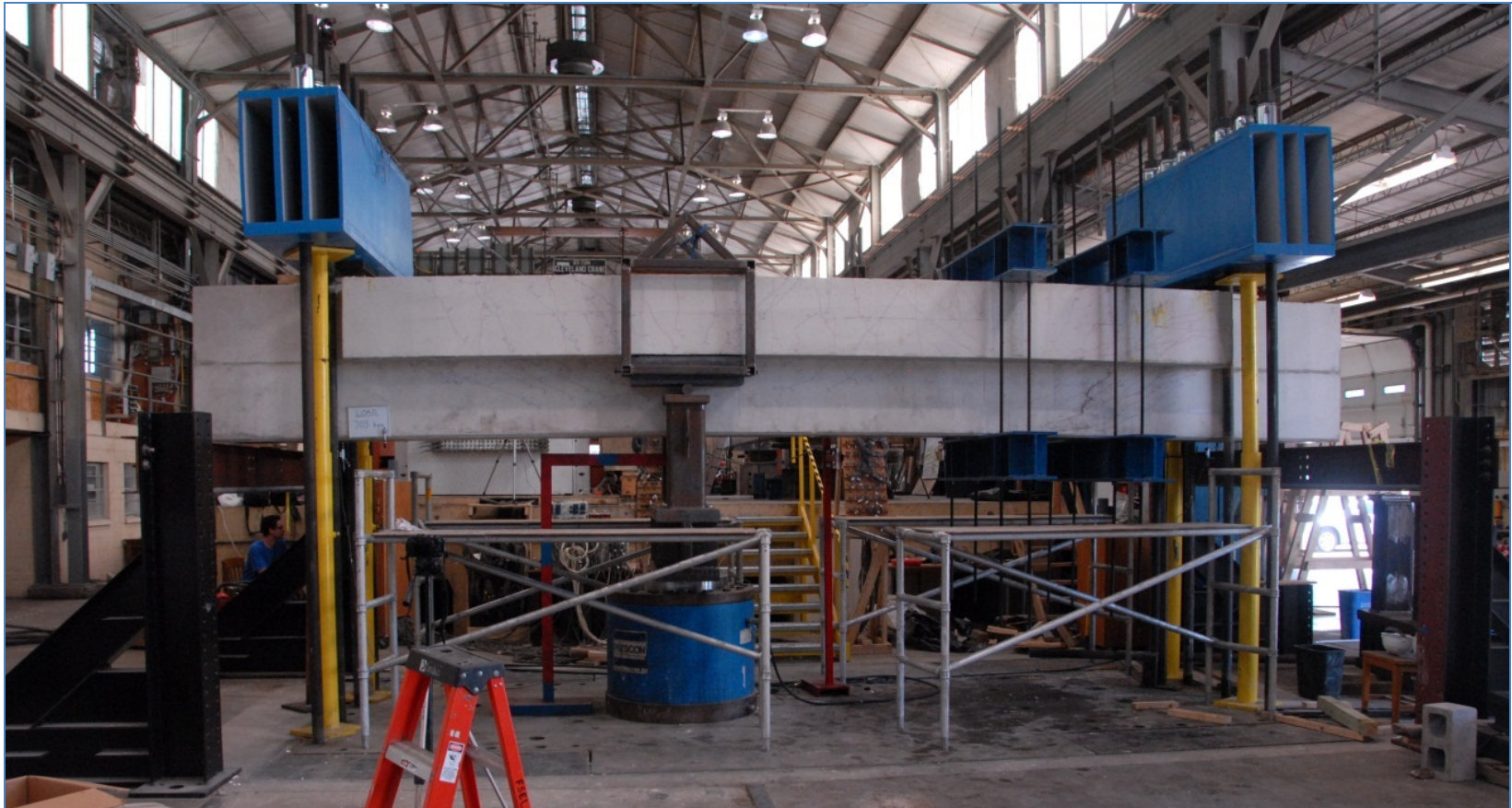
Figure 3-15: Inverted-T specimen subjected to single point load in test frame
