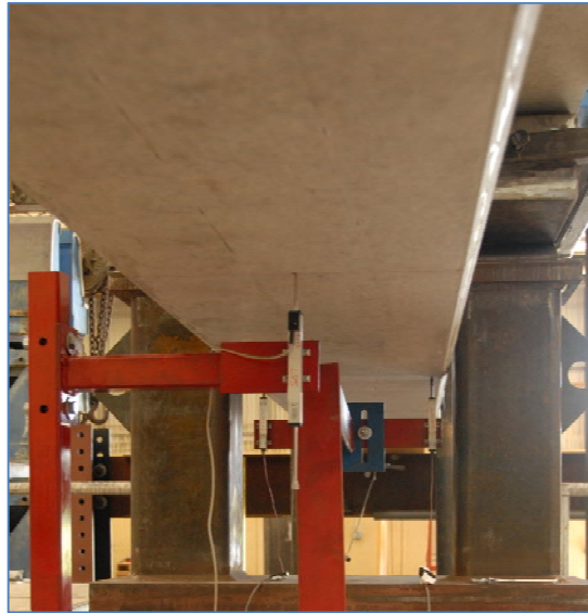
Figure 3-28: Typical placement of linear potentiometers at midspan and beneath the load point
