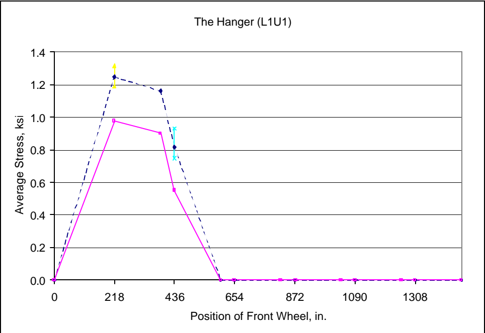
Graph F.92: Average stress: Vertical hanger (L1U1)
