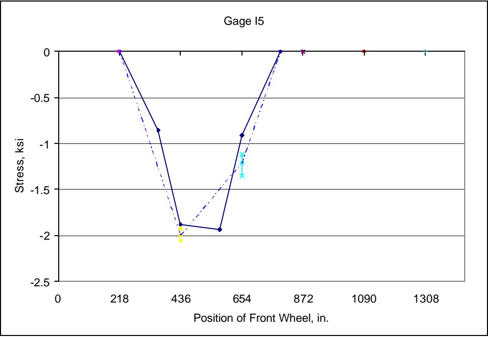
Graph F.44: Section at 23" away from the mid span of the metal floor beam
