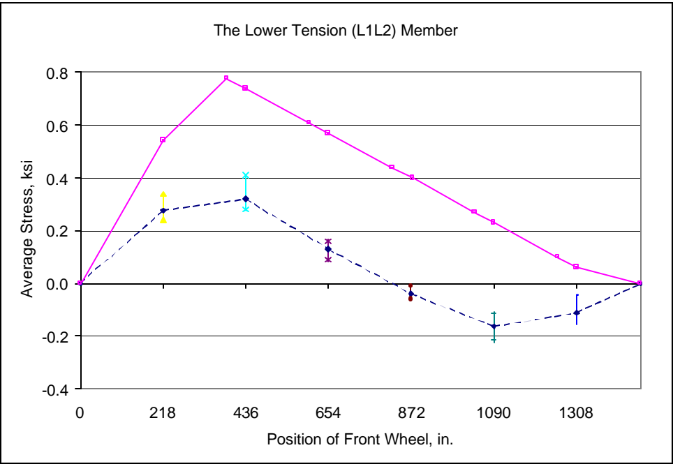
Graph F.87: Average stress: Bottom chord (L1L2)
