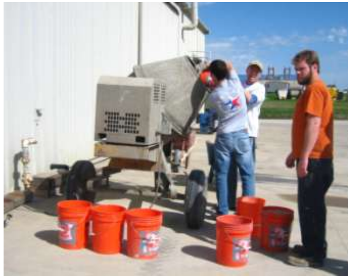
Figure 3.13 Mixing of the grout used in the splice specimens with No. 5 bars
