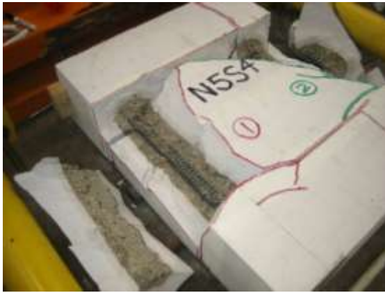
Figure A.16 Specimen N5S4 – Left and right splices
