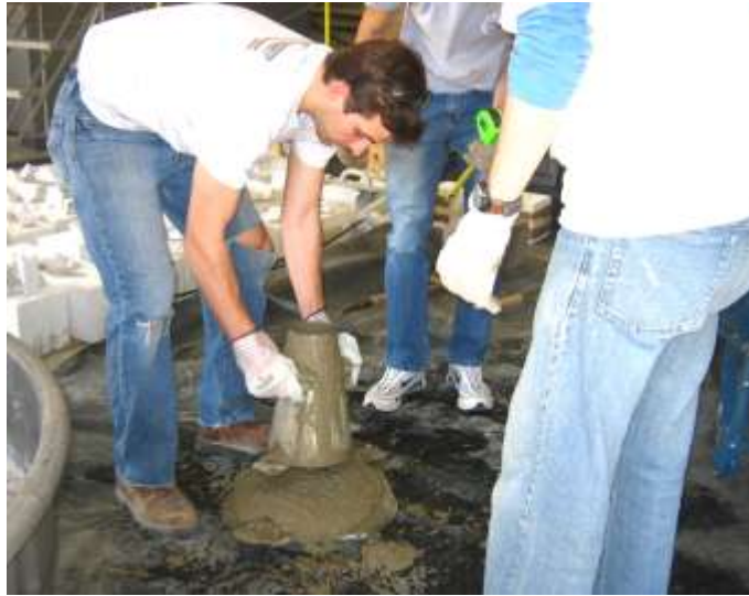
Figure 3.14 Initial slump test – Grout used in splice specimens with No. 5 bars
