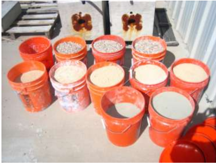
Figure 3.12 Cement, sand, and pea gravel used to grout the specimens with No. 4 bars
