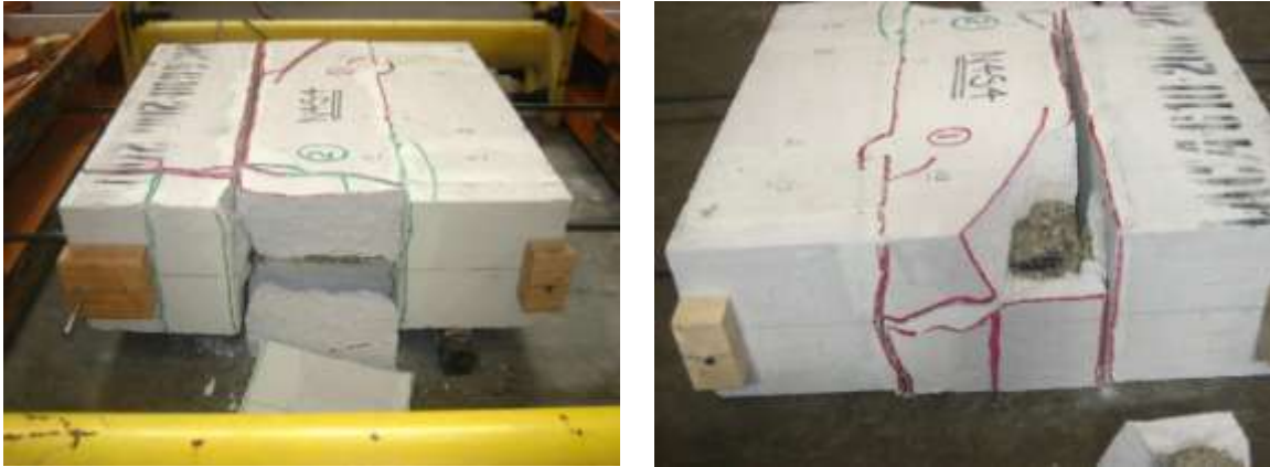
Figure 3.24 Specimen N4S4 – Left and right splices
