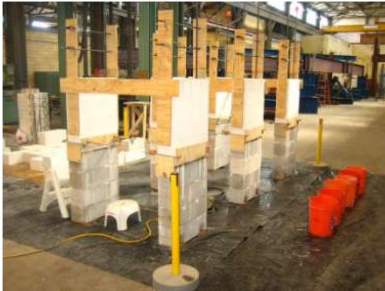
Figure 3.11 Splice specimens prior to grouting – No. 5 bars
