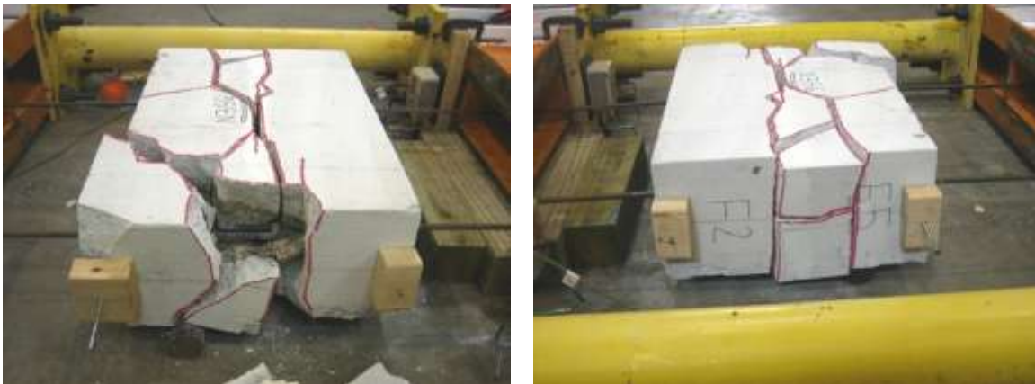
Figure 3.23 Specimen N3S6 – Left and right splices
