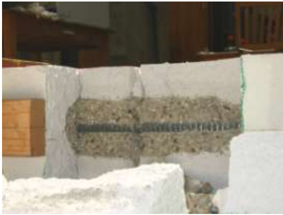
Figure A.10 Specimen N4S4 – Left and right splices
