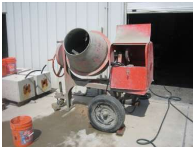
Figure 4.4 Mixer used to produce the grout
