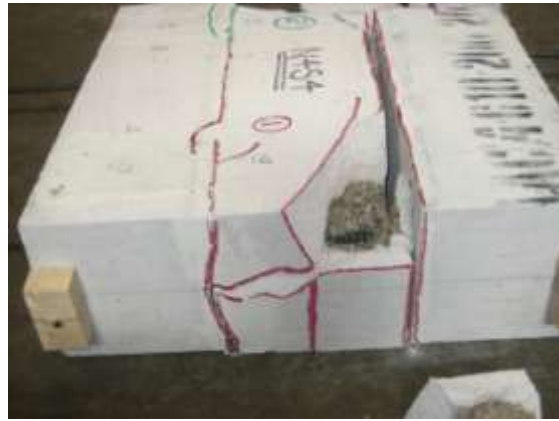
Figure A.10 Specimen N4S4 – Left and right splices
