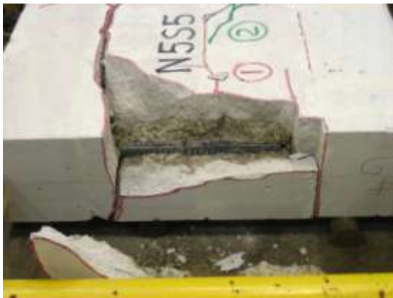
Figure A.17 Specimen N5S5 – Left and right splices
