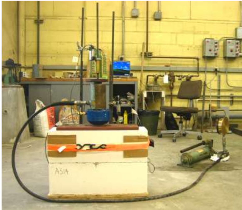
Figure 4.7 Photograph of pullout test setup
