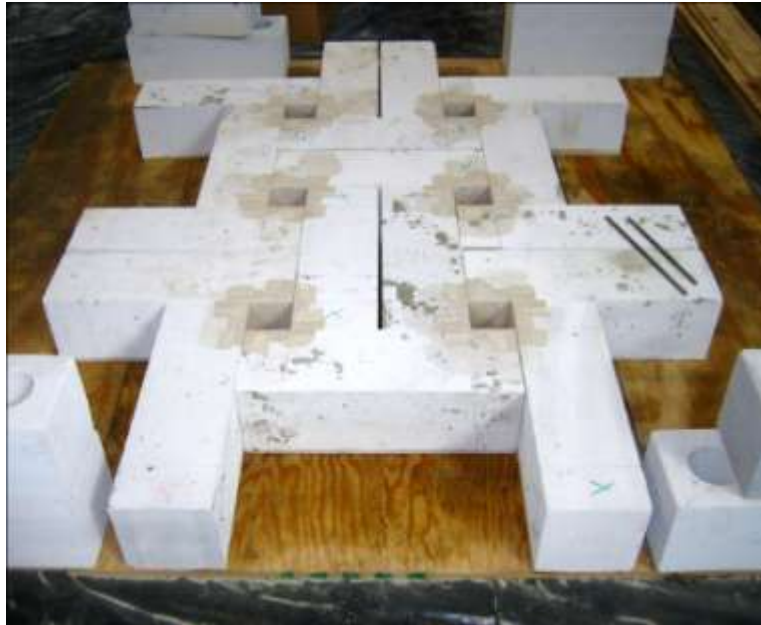
Figure 3.16 Fabrication of grout prisms
