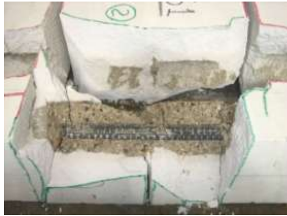
Figure A.13 Specimen N5S1 – Left and right splices
