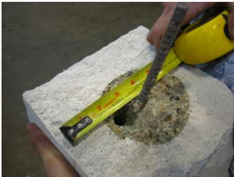
Figure 3.29 Void in grout surrounding the right splice of Specimen N3S4
