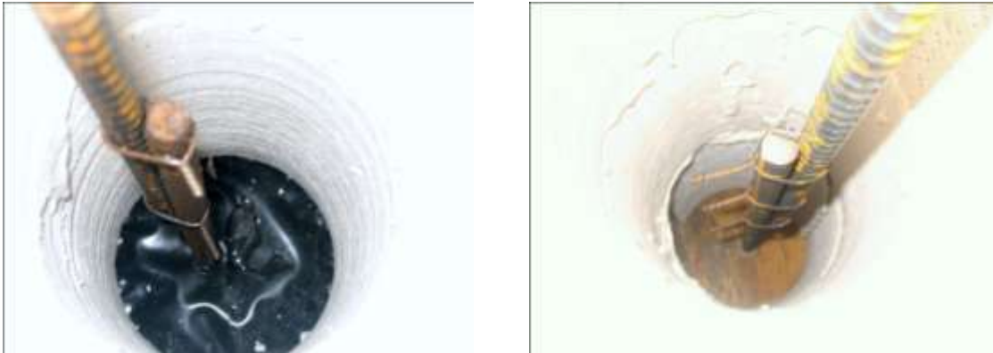
Figure 3.9 Bars spliced inside a core – No. 3 bars (left) and No. 4 bars (right)
