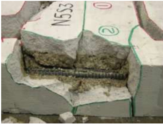
Figure A.15 Specimen N5S3 – Left and right splices
