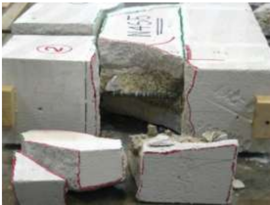
Figure A.11 Specimen N4S5 – Left and right splices
