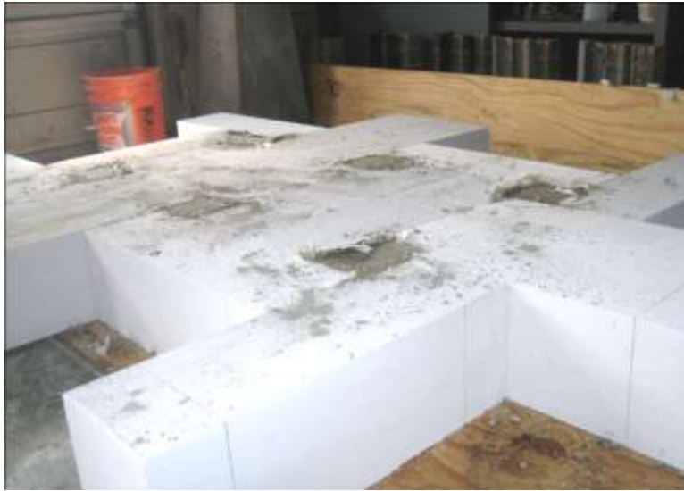
Figure 4.6 Fabrication of grout prisms
