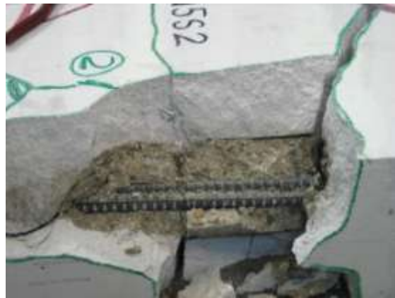
Figure A.14 Specimen N5S2 – Left and right splices
