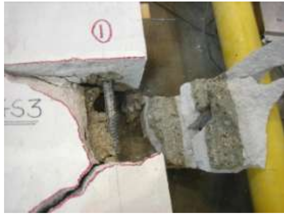
Figure A.9 Specimen N4S3 – Left and right splices
