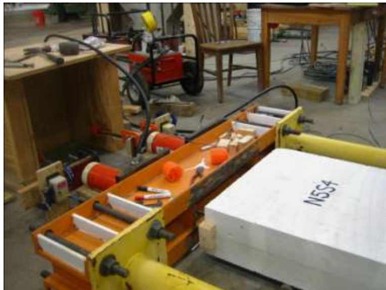
Figure 3.18 Rams and pressure gauge connected to air-driven hydraulic pump
