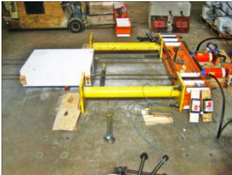
Figure 3.19 Lap-splice specimen on rollers prior to testing
