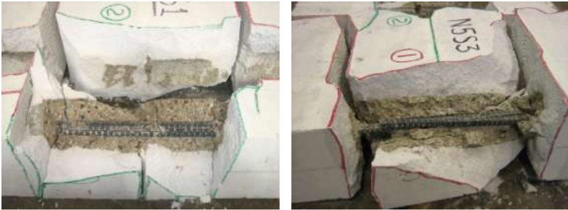
Figure 3.28 Right splice N5S1 (left) & right splice N5S3 (right)
