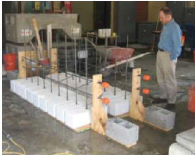
Figure 4.3 Pullout specimens prior to grouting
