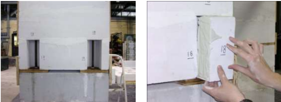
Figure 3.10 Cleanouts in a lap-splice specimen with No. 5 bars
