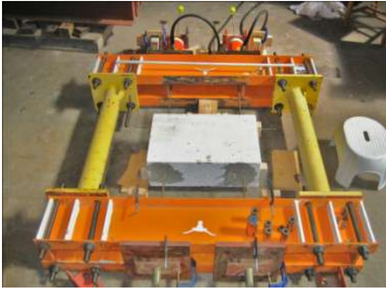
Figure 3.17 Lap-splice test setup
