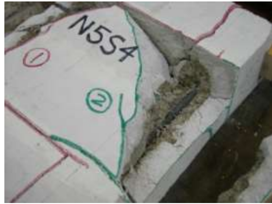
Figure A.16 Specimen N5S4 – Left and right splices
