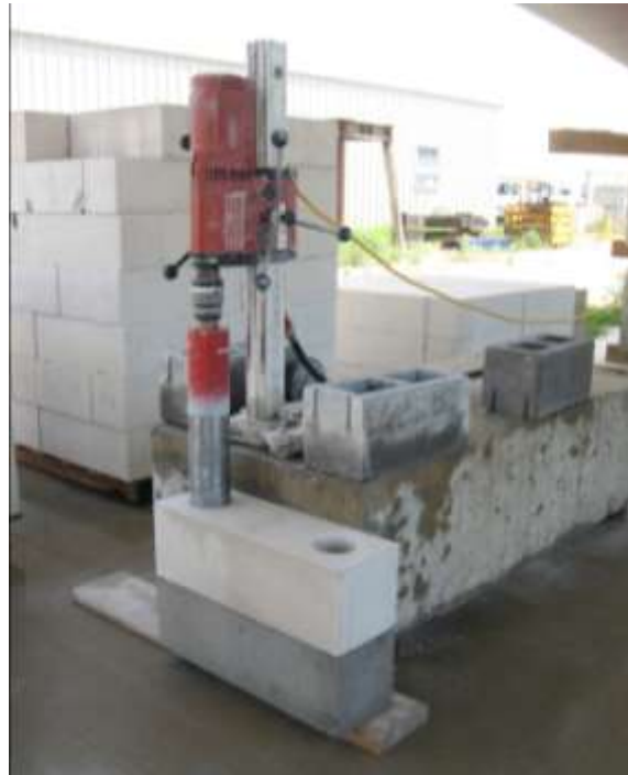
Figure 4.2 Core drilling of holes in specimens (repeated from Chapter 3)
