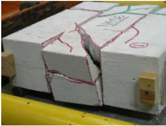
Figure A.12 Specimen N4S6 – Left and right splices
