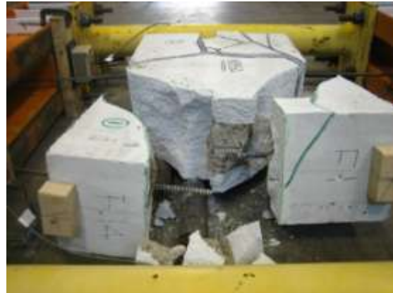
Figure A.1 Specimen N3S1 – Left and right splices
