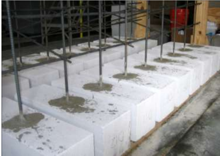
Figure 4.5 Pullout specimens after grouting
