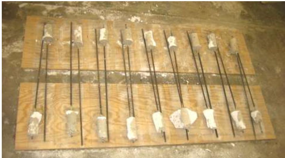
Figure 4.13 Grout cores – AS1 through AS9 (top) & AS10 through AS18 (bottom)
