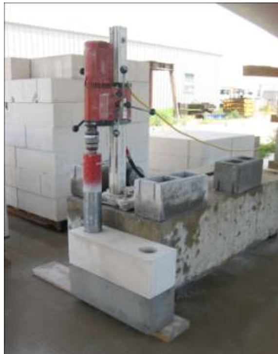
Figure 3.7 Core drilling of blocks in lap-splice specimens
