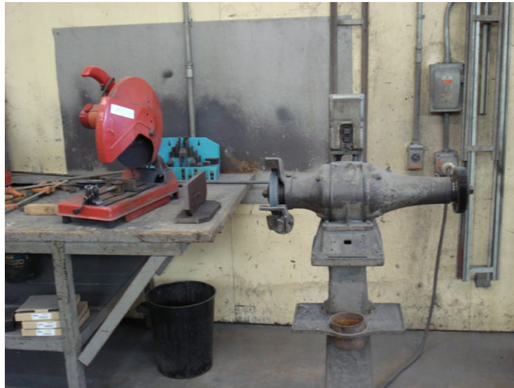
Figure 3.1: Chop Saw and Table Grinder
