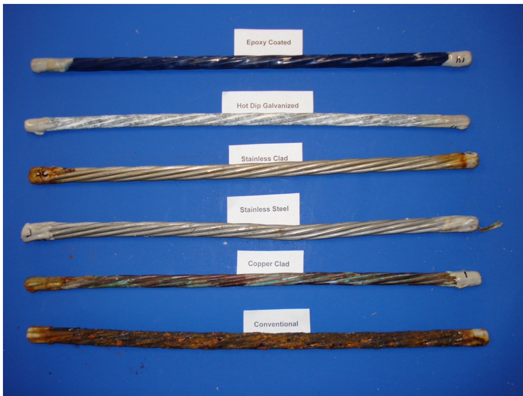
Figure 4.16: All the Strands After Six Months
