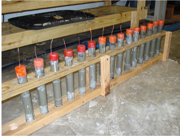
Figure 3.17: Final Configuration Before Curing
