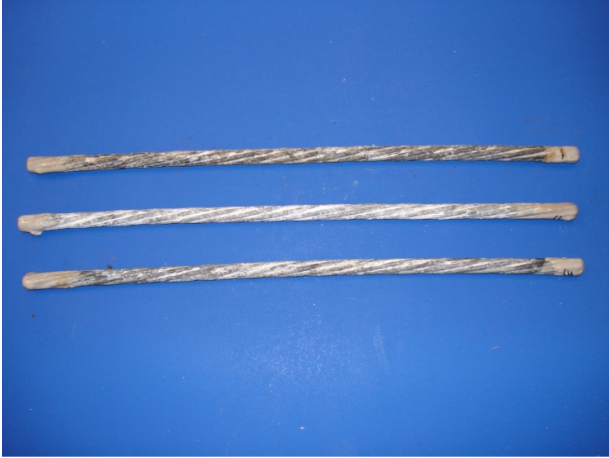
Figure 4.7: Hot Dip Galvanized Strands at Six Months
