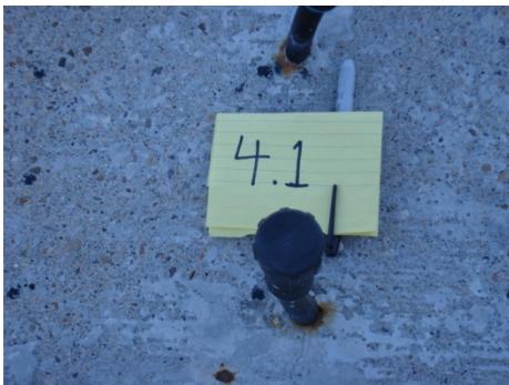
Figure 2.9: Rust Spots on Beams 4.1 and 1.4
