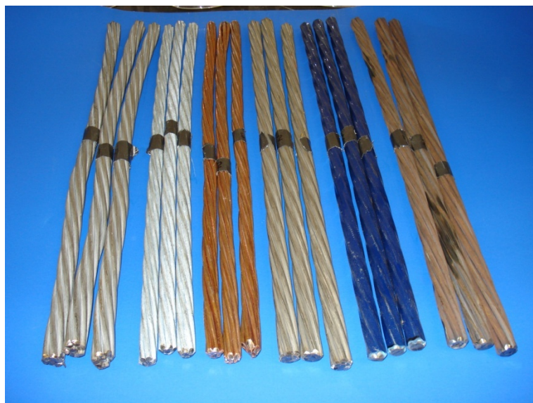
Figure 3.2: Specimens Used in Exposed Strand Test
