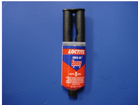
Figure 3.13: Quick Set Epoxy Used to Fill Acrylic Holes
