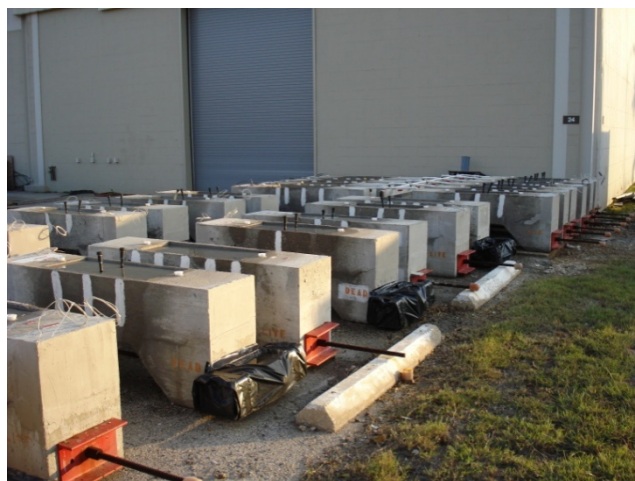
Figure 2.1: Layout of Large Scale Exposure Specimens
