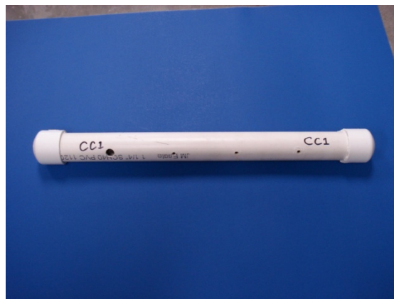
Figure 3.4: Pipe Configuration with Capped Ends and Holes Drilled
