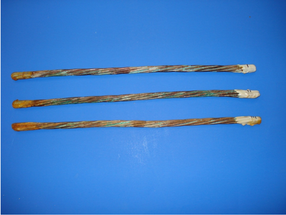
Figure 4.9: Copper Clad Strands at Six Months
