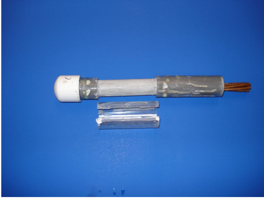
Figure 5.13: Specimen After Removal of Pipe Over Exposed Region
