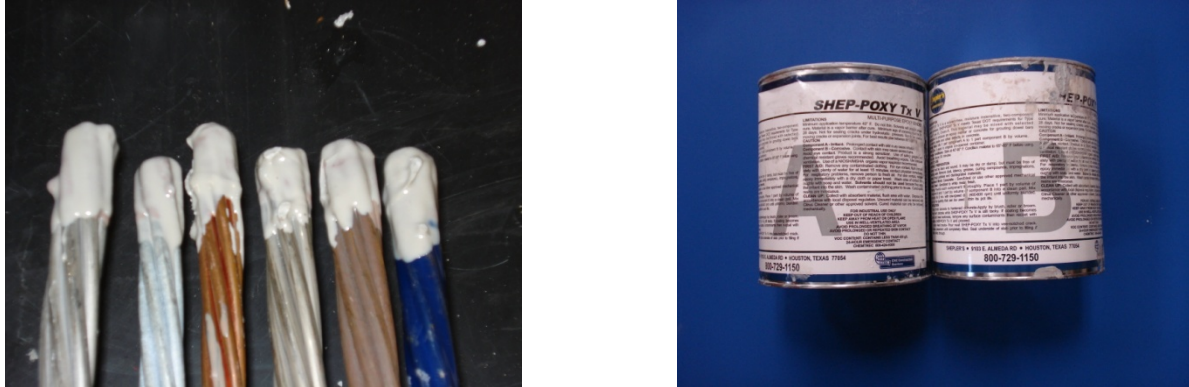
Figure 3.3: Strands with Epoxy Ends and the Epoxy Used
