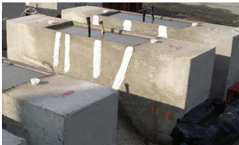
Figure 2.5: Caulked Region on Beam Specimens and Type of Caulk Used
