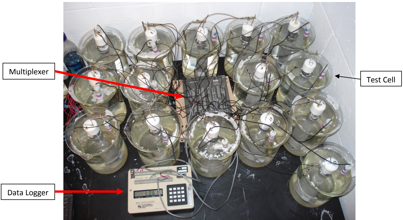
Figure 3.20: Grouted Strand Test Complete Setup
