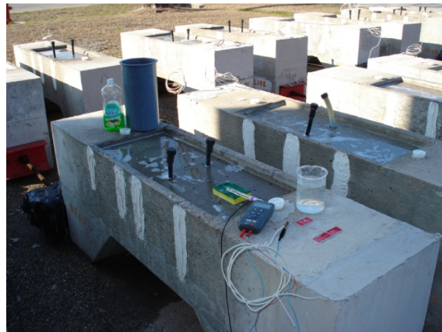
Figure 2.4: Equipment Used to Measure Half-Cell Potentials
