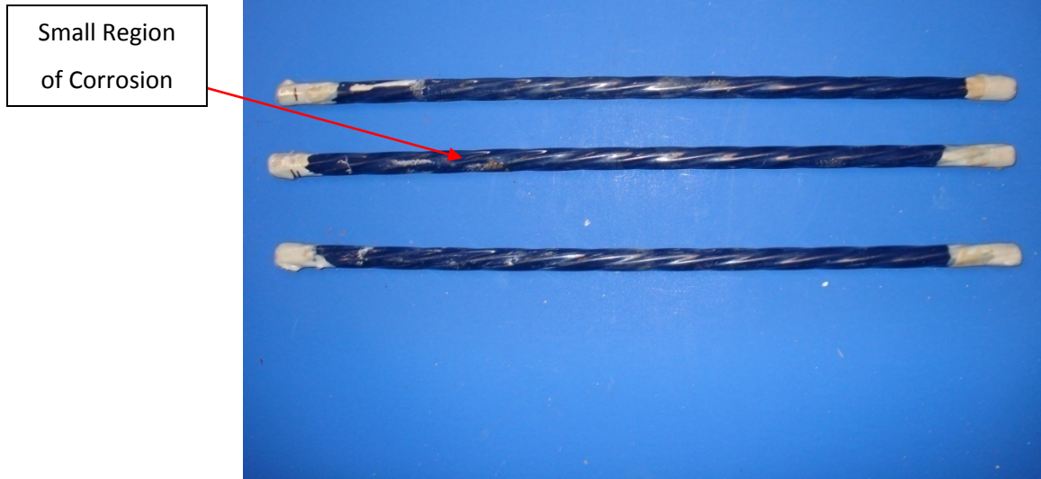
Figure 4.1: Flow Filled Epoxy Coated Strands at Six Months
