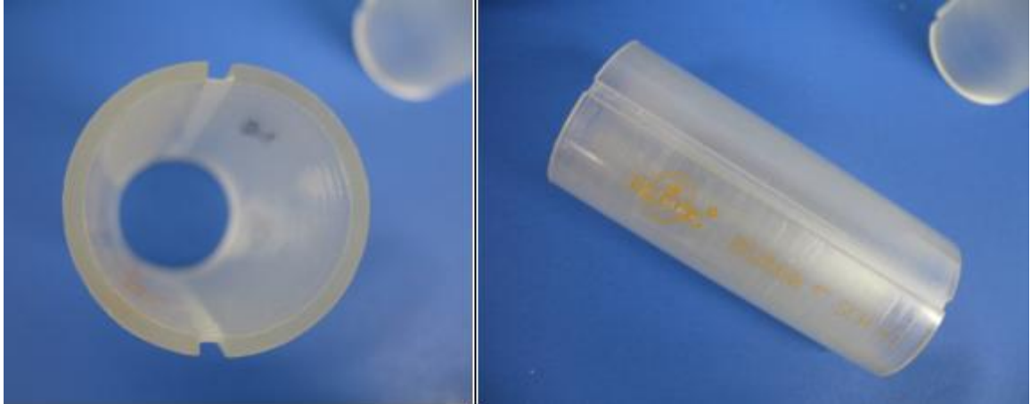
Figure 3.11: Section of Pipe Grooved and Bored Out 14
