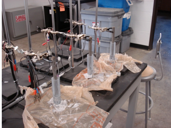
Figure 3.14: Applying Epoxy to the Bottom of the Strand
