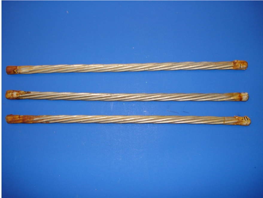
Figure 4.3: Stainless Clad Strands at Six Months
