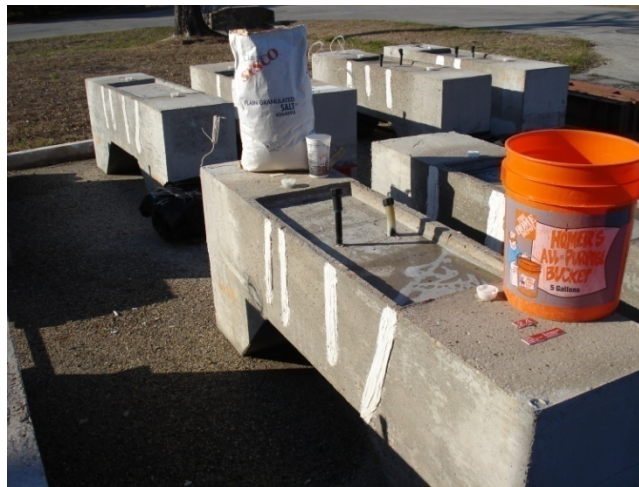
Figure 2.2: Specimen Embedment and Equipment Used to Apply Solution
