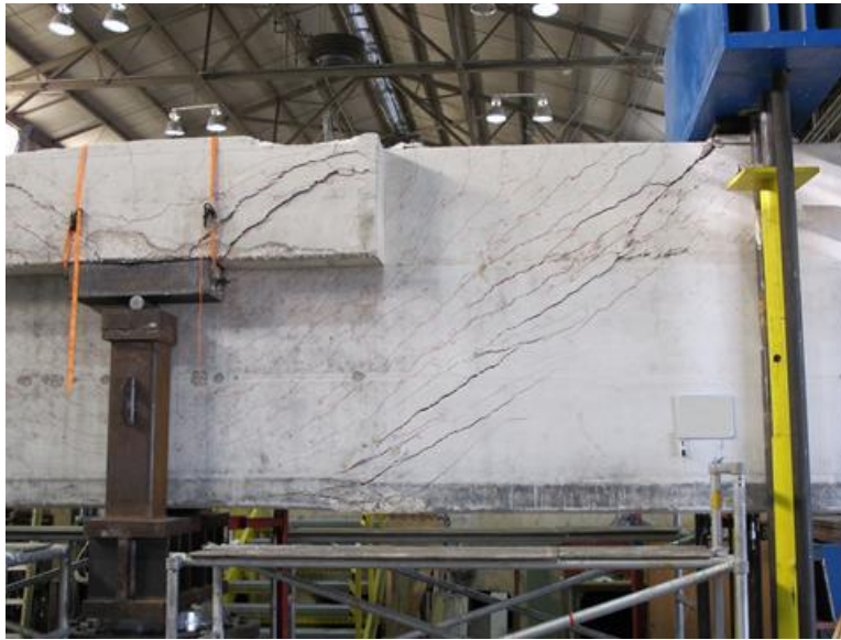
Figure D-37: Specimen after failure
