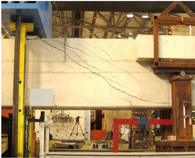
Figure D-43: Specimen after failure
