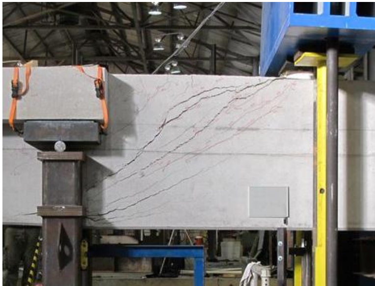
Figure D-21: Specimen after failure
