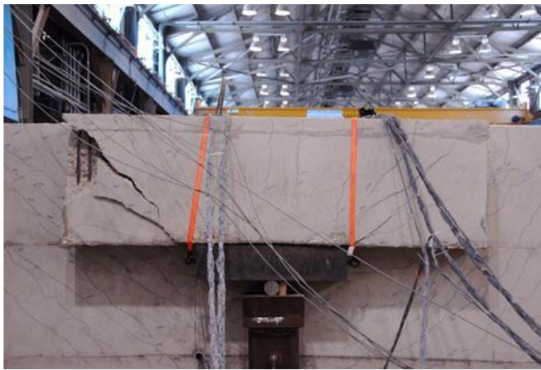
Figure D-25: Specimen after failure
