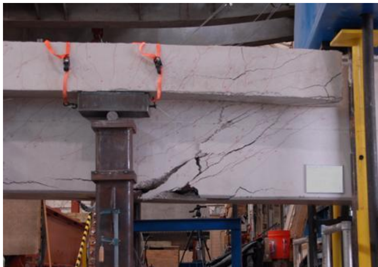
Figure D-35: Specimen after failure
