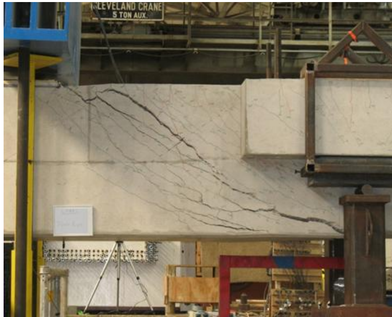
Figure D-7: Specimen after failure
