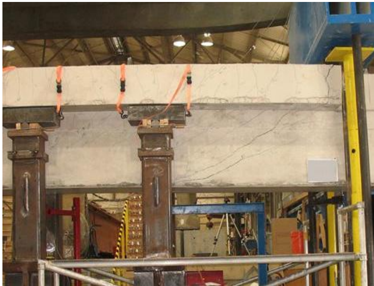
Figure D-33: Specimen after failure
