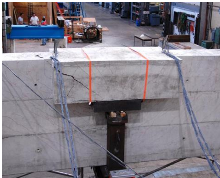
Figure D-23: Specimen after failure
