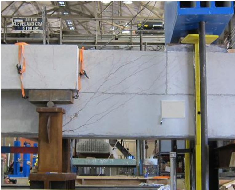
Figure D-61: Specimen after failure
