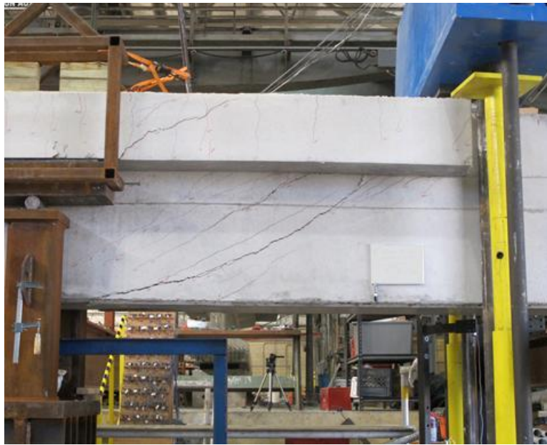
Figure D-51: Specimen after failure
