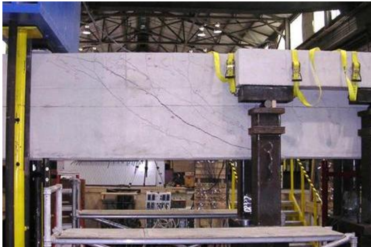
Figure D-19: Specimen after failure
