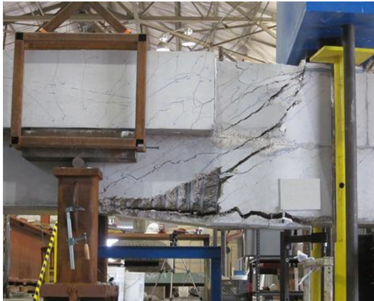
Figure D-57: Specimen after failure
