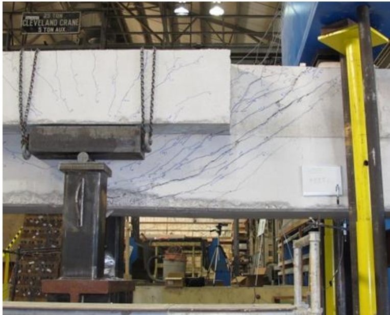
Figure D-1: Specimen after failure
