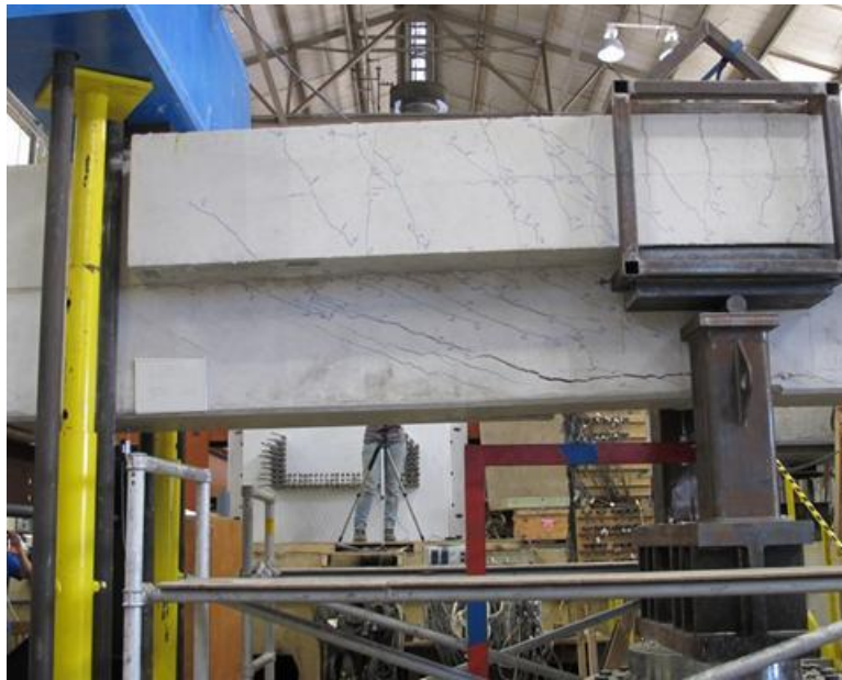
Figure D-11: Specimen after failure
