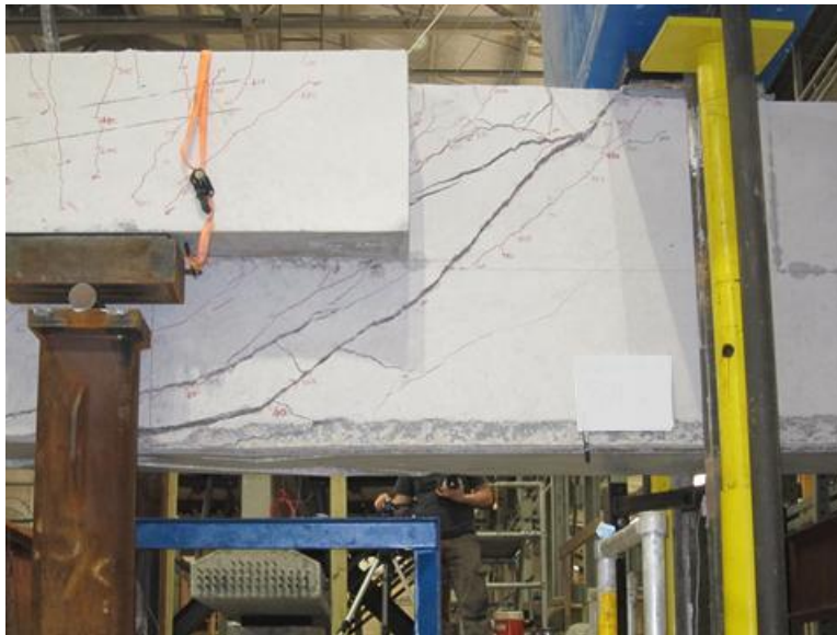
Figure D-41: Specimen after failure
