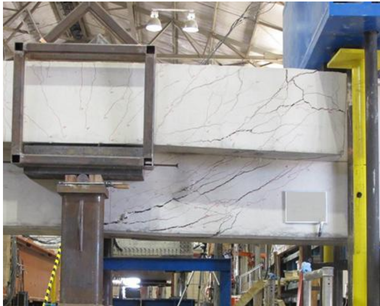
Figure D-29: Specimen after failure
