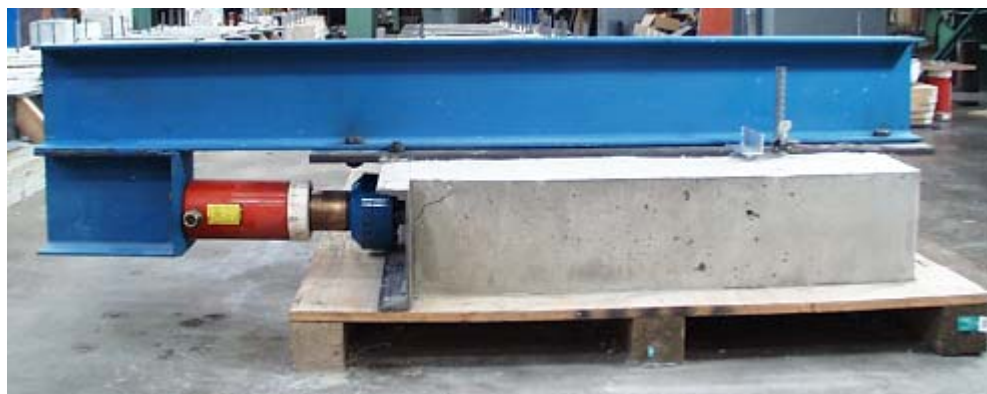
Figure 2.2: Side View of the Push-out Test Setup
