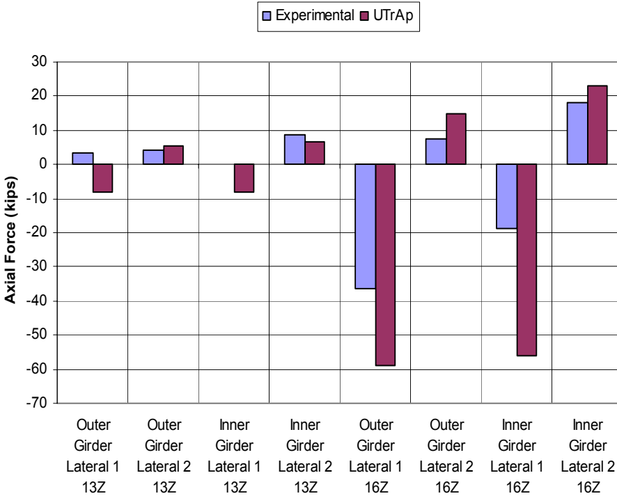
Figure 4.8: Change in Axial Force Levels Due to Pour 2
