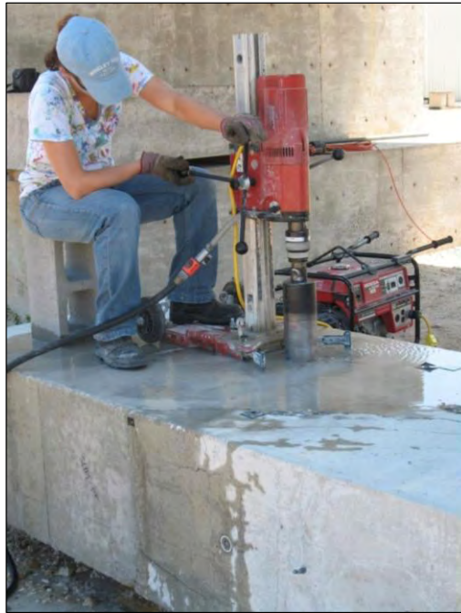
Figure 4-30: First Series Specimens - Extraction of Cores
