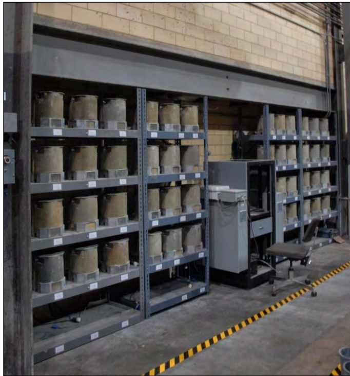
Figure 3-22: FSEL Sure Cure System – Controller and Molds
