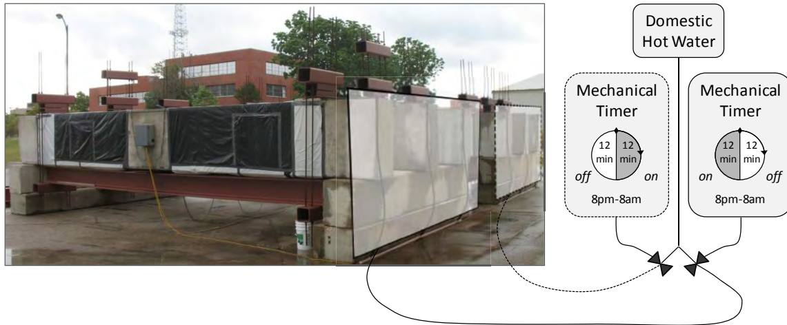
Figure 4-6: Alternating Two-Zone Watering System
