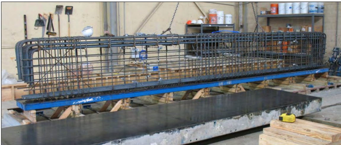
Figure 3-13: Instrumented Reinforcement Cage on Form Soffit
