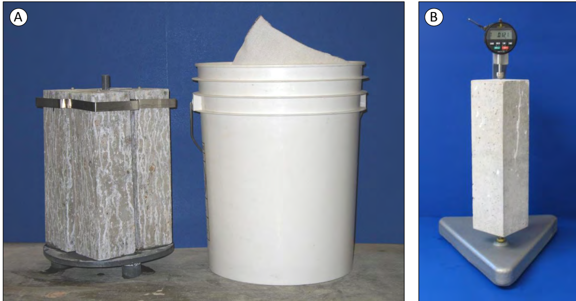
Figure 3-25: Free Expansion Potential (A) Elevated Prisms Set in Felt-Lined Bucket (B) Periodic Measurement of Length Change with Digital Comparator
