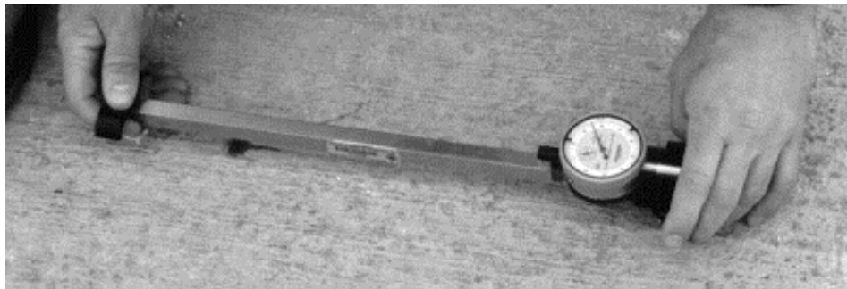
Figure 2.25 The Demec extensometer
