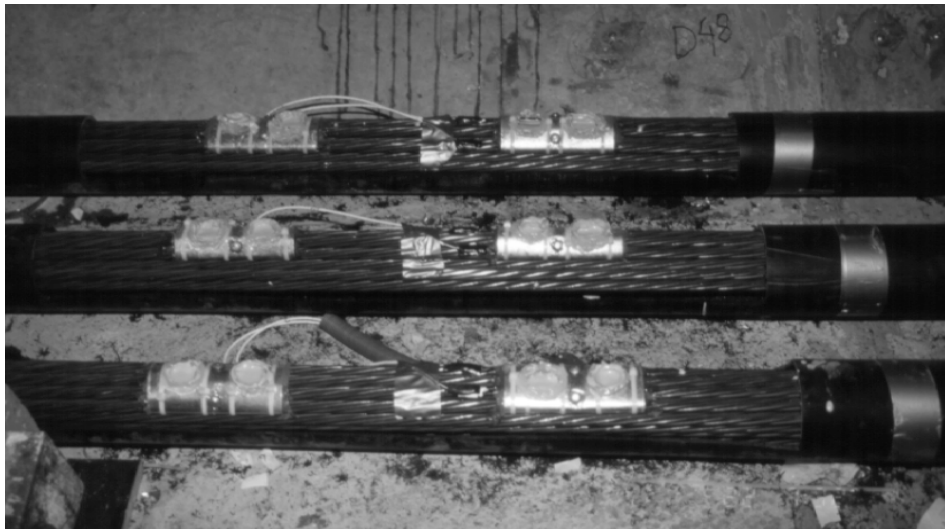
Figure 2.31 Epoxy sleeve strain measurement system
