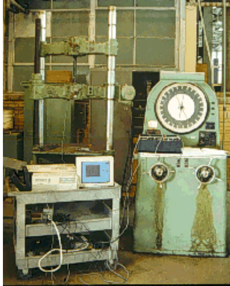
Illustration 3-3: Southwark-Emery testing machine with data acquisition system
