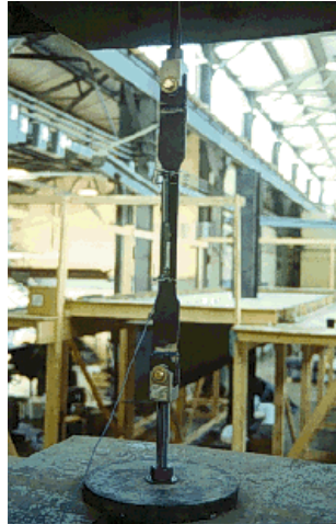
Illustration 3-5: Gripping arrangement for Riehle testing machine
