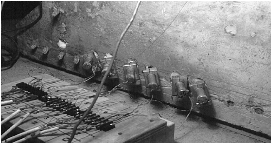
Figure 3.10: Rotation of Strand Slip Gages at Failure of Box Beam 5 - Test 2
