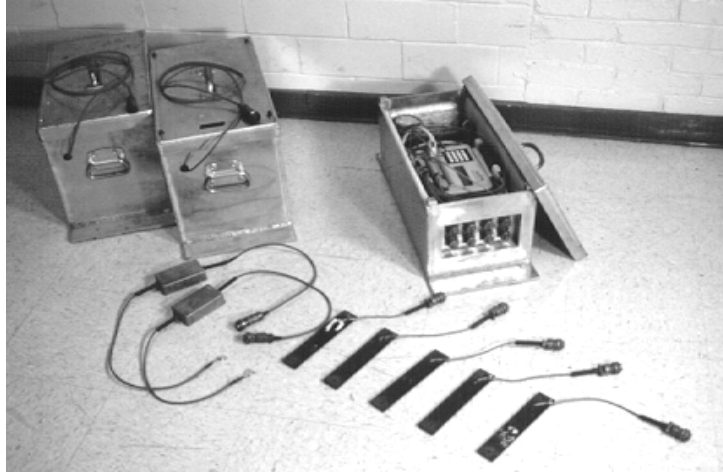
Figure 3.2 Data acquisition system and strain transducers used in test.
