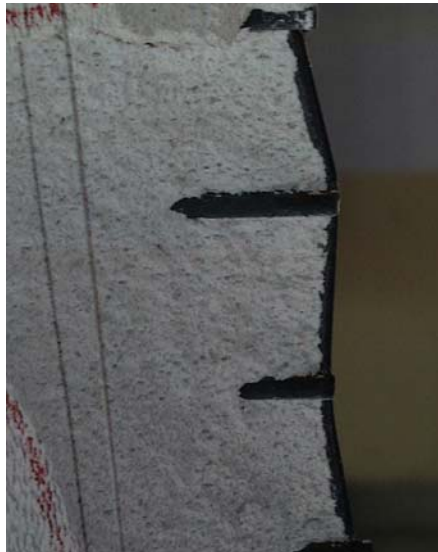
Figure 6-8: Yielding of vertical wire of reinforcement
