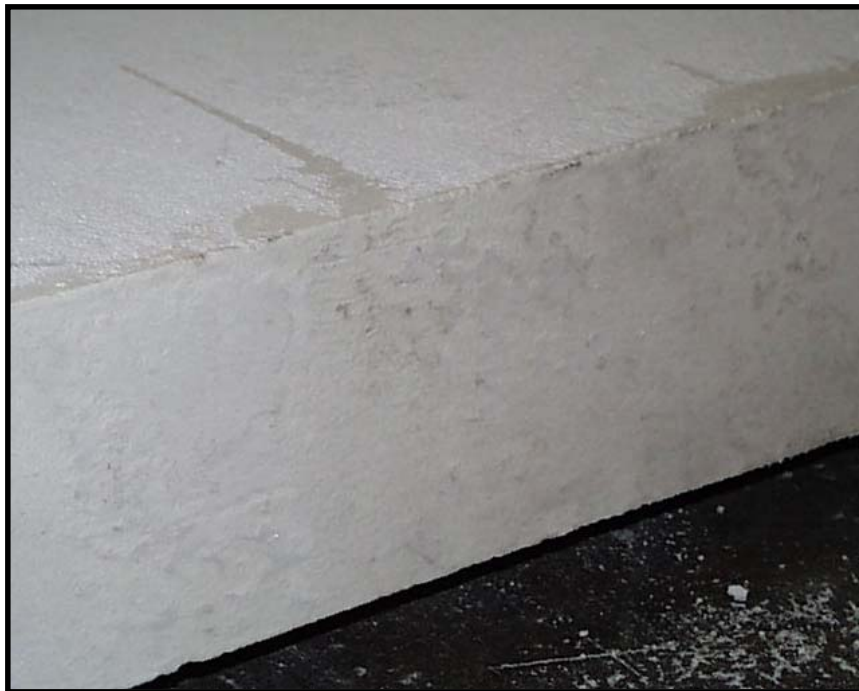
Figure 6-4: Typical thin-bed joint in Shear Wall Pilot Specimen 2
