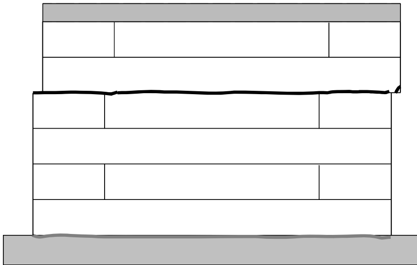
Figure 4-4: Cracking of Shear Wall Pilot Specimen 1 at Cycle 6a (horizontal crack at mortar joint under second panel from top)
