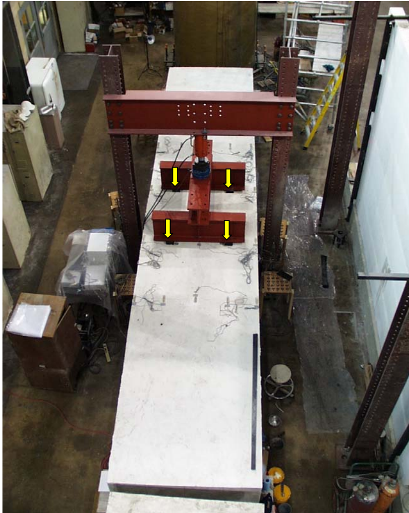
Figure 5.2 Overhead View of Pan-Joist Specimen Showing the Location of Loading Points
