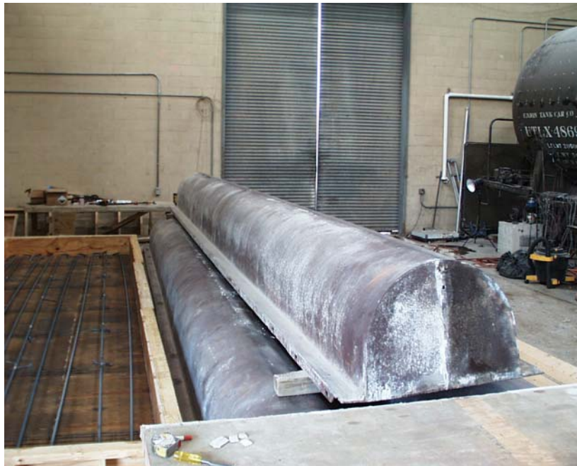
Figure 4.1 View of Metal Pan-Forms inside the Laboratory
