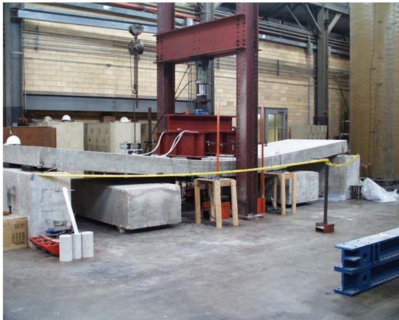
Figure 8.16 West Side View of Specimen FS-2 at Ultimate Deformation Corresponding to Initiation of Concrete Crushing
