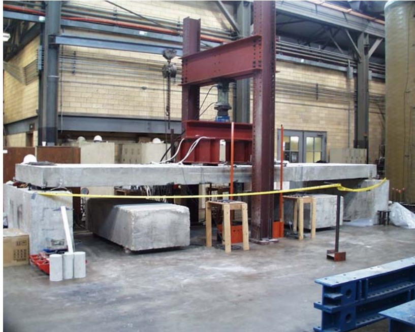
Figure 8.1 Picture Showing the Experimental Setup Used for the Laboratory Tests of the Flat-Slab Specimens
