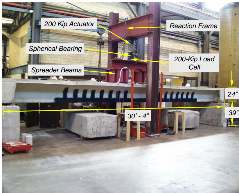
Figure 5.1 Side View of Pan-Joist Specimen in Laboratory Test Setup
