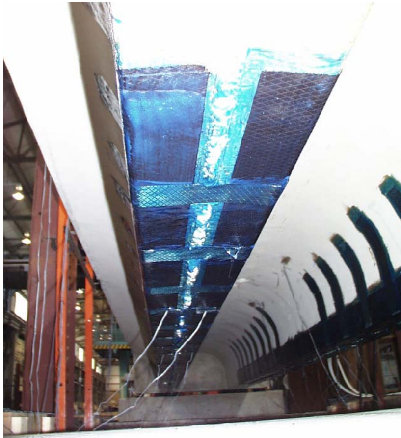
Figure 4.12 Partial Wrapping of Joists in Specimen J-2 to Avoid Concrete Surface Irregularities
