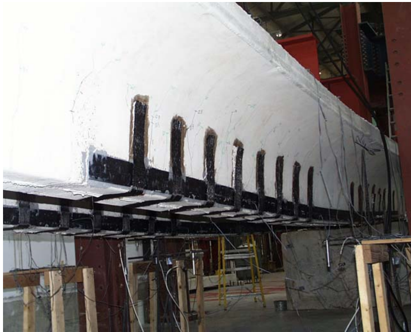
Figure 5.8 East Joist of Specimen J-1 Before CFRP Debonding
