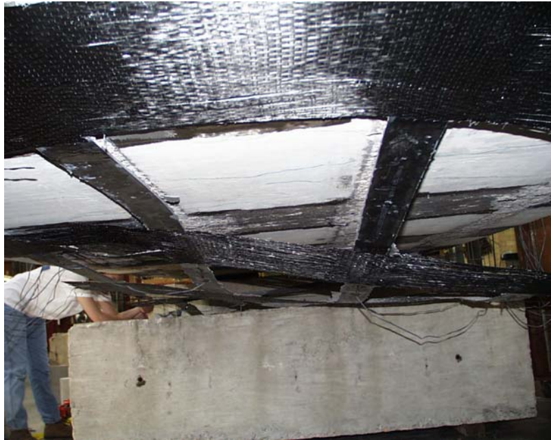
Figure 8.7 Bottom View Toward North End of Specimen FS-1 after CFRP-Plate Debonding
