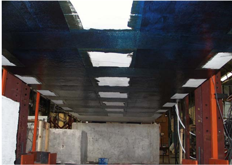
Figure 7.11 Picture of the Bottom Surface of Specimen FS-2 after Strengthening with the CFRP Wet-Layup System
