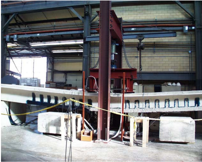
Figure 5.13 View of West Joist in Specimen J-2 at Failure
