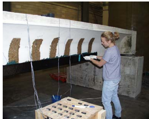
f) Coating placed sheets with epoxy
