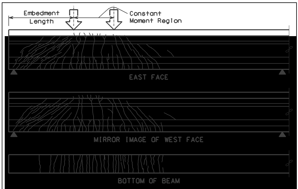
Figure 4.13 Crack pattern for test no. 7-N2S-78
