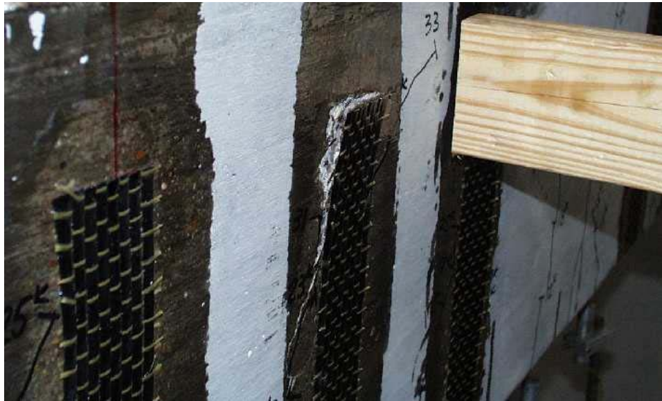
Figure 4.21: Debonding of Strap
