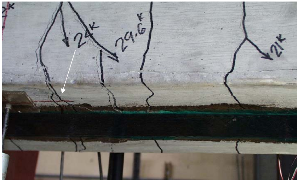
Figure 4.8: Photograph of Debonding Initiated by Prying Action
