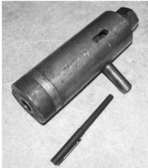
Figure 5.22: Setting tool for undercut anchor
