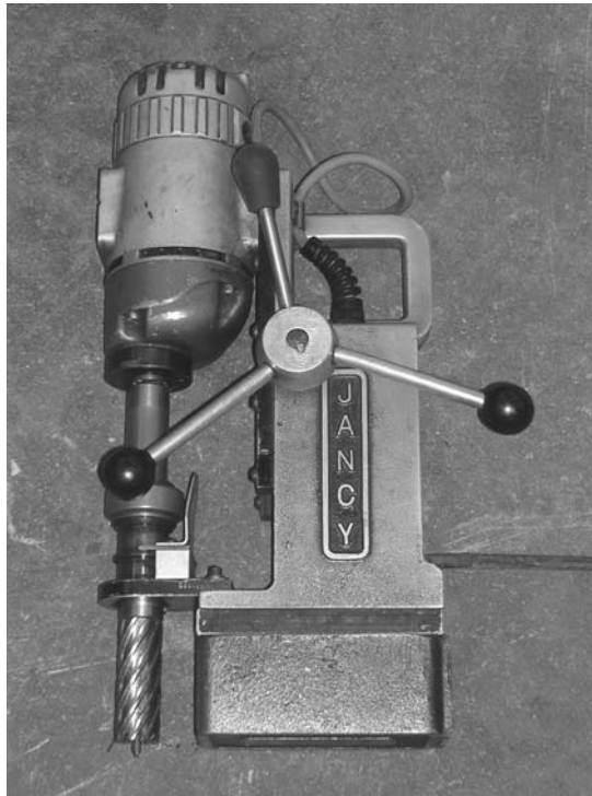
Figure 3.6: Slugger™ drill with 1/4-in. Slugger™ bit
