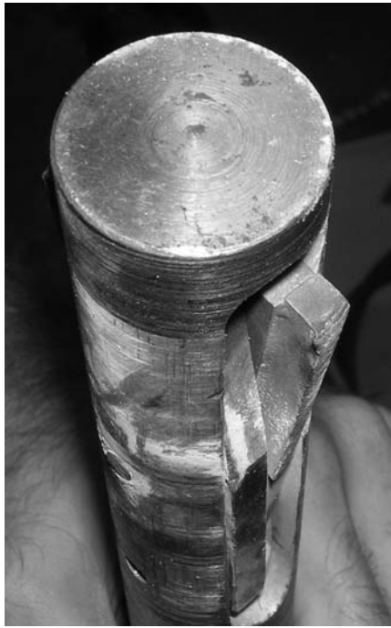
Figure 5.21: Diamond insert blades on undercutting tool
