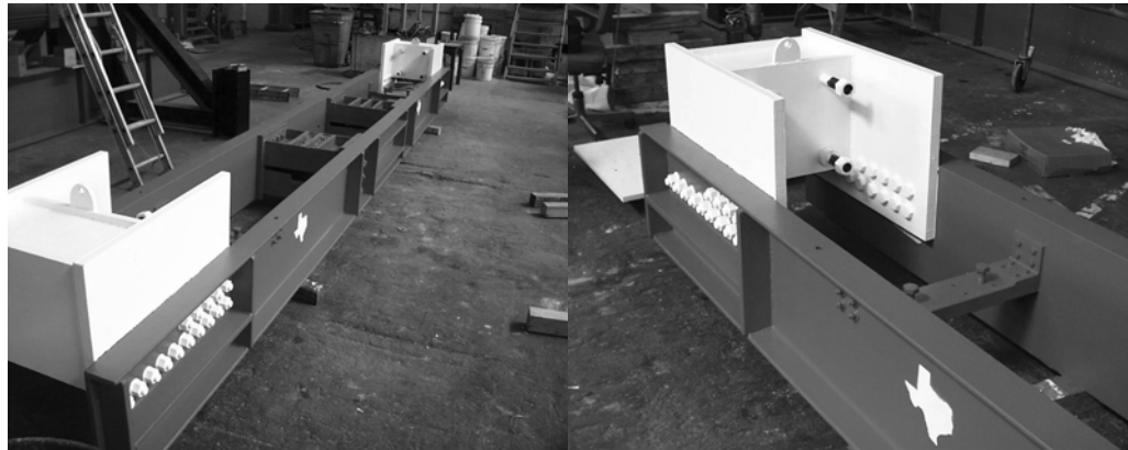
Figure 5.25: (a) Self-contained test frame; (b) Bulkhead used as reaction wall
