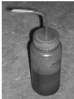
Figure 3.7: Squeeze bottle with machine oil for cooling Slugger™ bit
