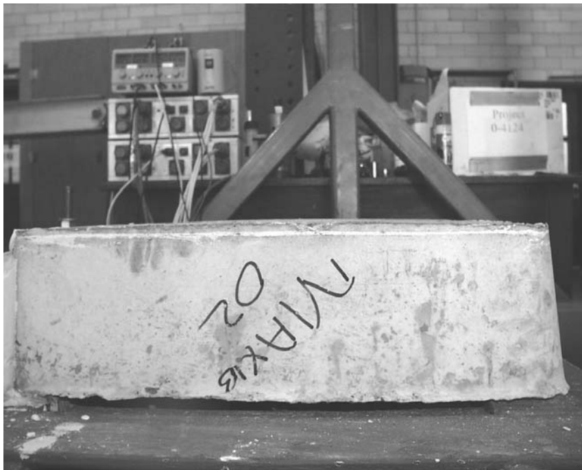
Figure 6.31: No cracks in side of slab for MAXIB02
