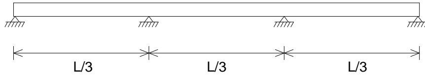
Example Three-Span Structure
