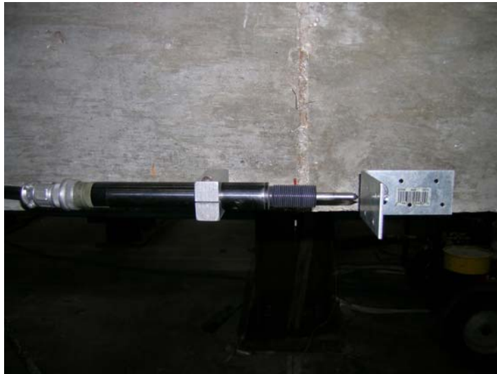
Figure 4-7: DCDT used to measure bottom strain during the static test
