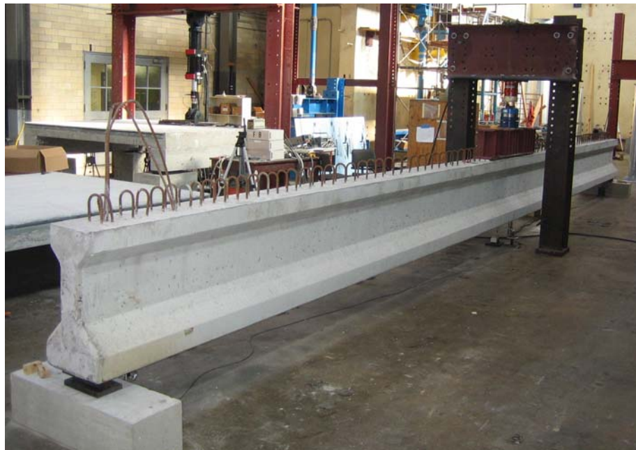
Figure 4-12: Picture of test setup for static testing of full-scale girders
