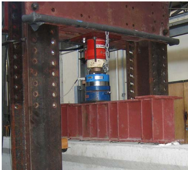
Figure 4-9: Midspan region of test-setup for full-scale beams
