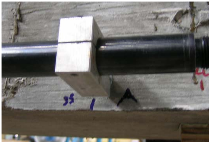
Figure 5-7: Documentation of first crack for IT1-73-2-T19 (picture was taken at P_{app} = 75 -kips)
