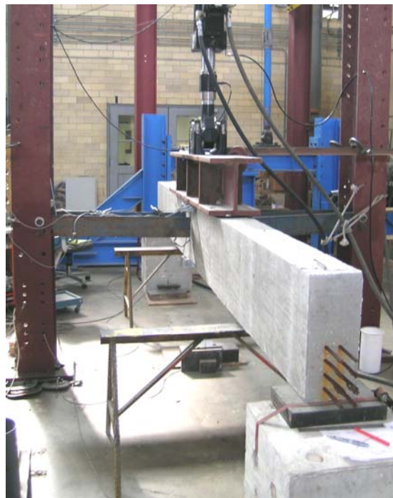
Figure 4-17: Picture of test setup for fatigue testing
