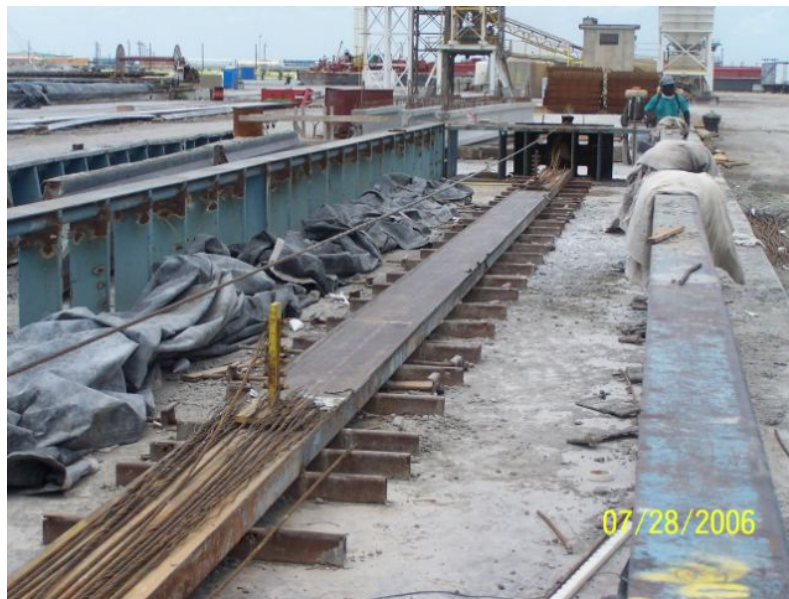
Figure 6-6: Small bed at HEI Corpus Christi plant used to cast Type-A beams (photograph courtesy of Chris Leonard)
