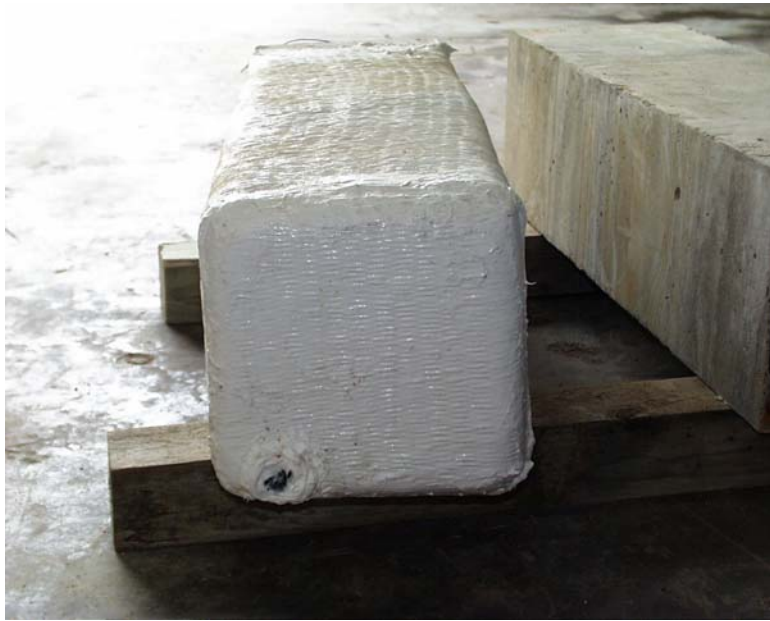
Figure 5.7 Wrapped rectangular block specimen.
