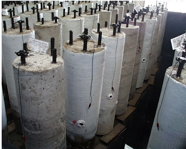
Figure 6.1 Cylinder specimens in the exposure tank.
