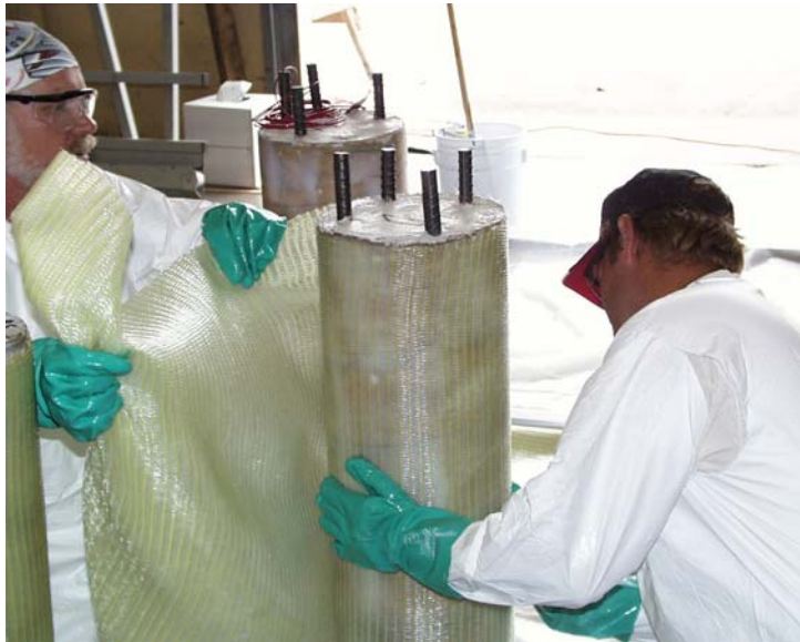
Figure 8.4 Applying FRP wrap to the concrete specimen.
