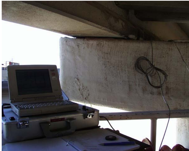
Figure 7.2 PR-Monitor test setup for Structure #12.
