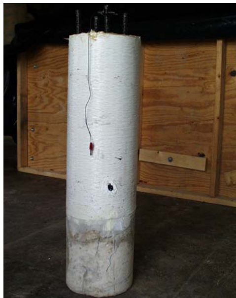
Figure 5.6 Wrapped cylinder specimen.
