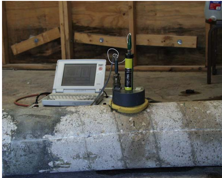
Figure 6.8 PR-Monitor test setup on specimen CC5.
