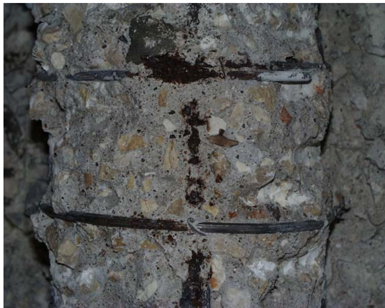
Figure 6.15 Macrocell formation in the top portion of specimen CC5.
