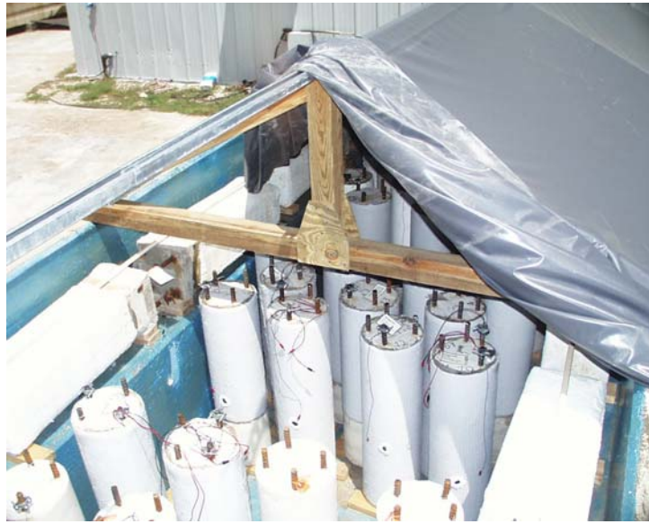
Figure 8.8 Specimens in the exposure tank.
