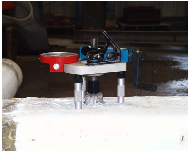
Figure 6.11 Test setup for DYNA Z16 Pull-Off Tester.
