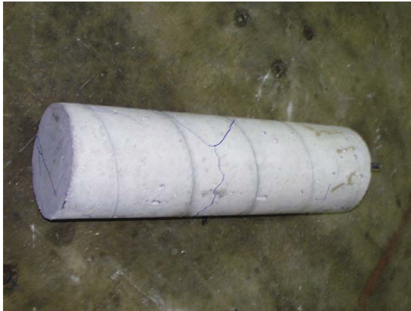
Figure 5.5 Cracked cylinder specimen.
