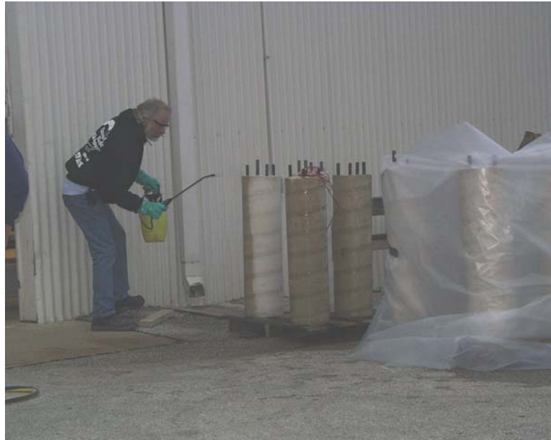
Figure 8.1 Application of a surface applied corrosion inhibitor to the specimens.
