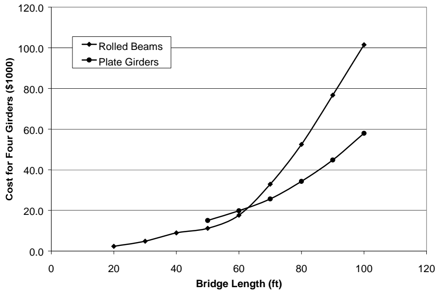
Figure 7.4 Comparison of Girder Costs for Bridges with Steel Grid Decks
