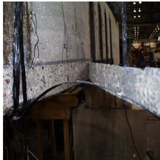
Figure 5.29.d: Plate-concrete interface: delamination of concrete (SK-e6-1/17)
