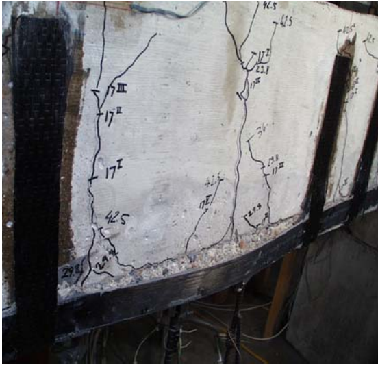
Figure 5.29.a: Debonding at midspan (SK-e6-1/17) Figure 5.29.b: Debonding at midspan (SK-e6-1/12)
