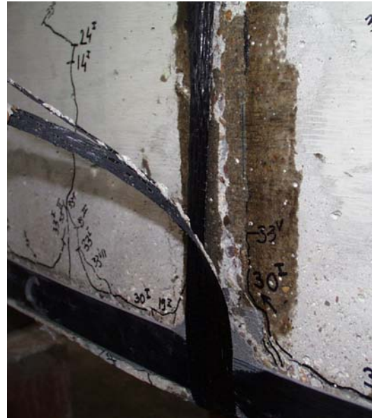
Figure 5.15.b: Debonding propagation and progression of cracking under transverse strap
