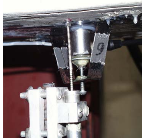
Figure 4.12.d: Linear potentiometer at the bottom face of the beam and acoustic emission sensor.
