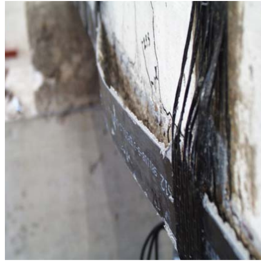
Figure 5.29.a: Debonding at midspan (SK-e6-1/17) Figure 5.29.b: Debonding at midspan (SK-e6-1/12)
