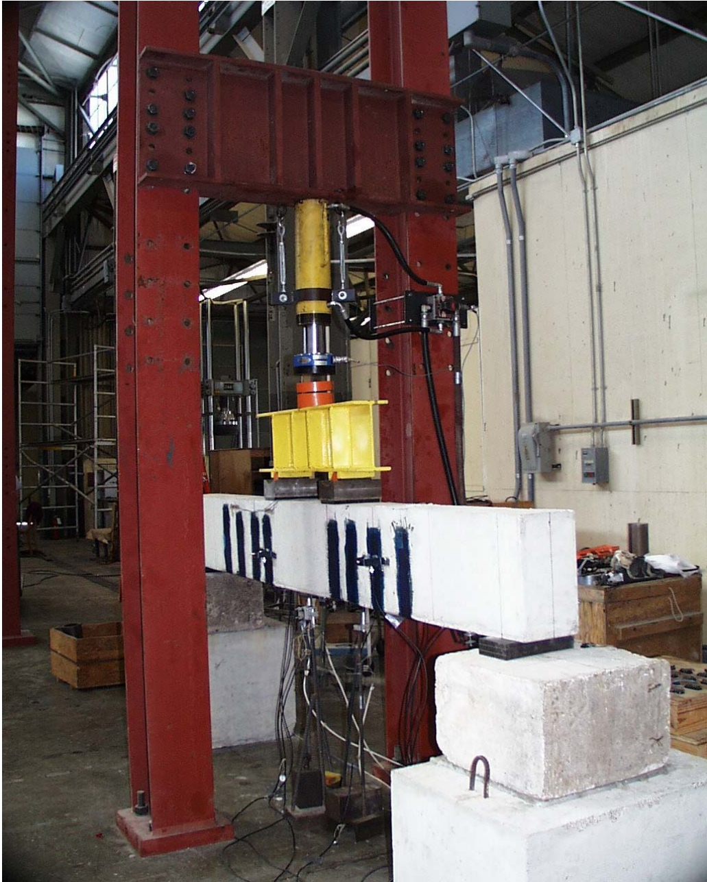
Figure 4.9: Test set-up, beam strengthened with the wet lay-up system.
