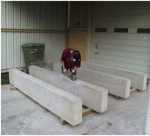
Figure 4.6.a: Beams are turned upside down to prepare the bonding surface.
