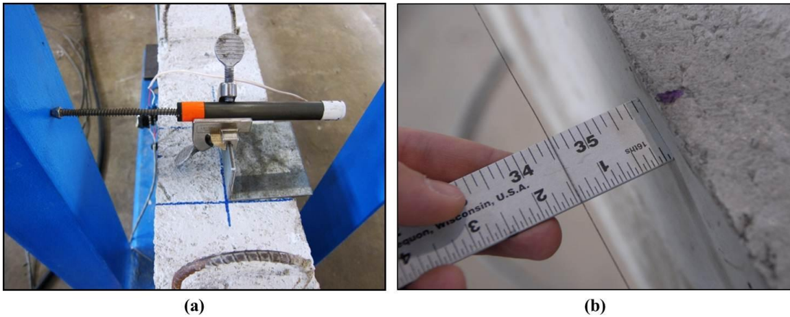
Figure 3-25: Deflection Measurements; (a) Linear potentiometer for measuring lateral deflection at midspan; (b) Deflected shape measurement
