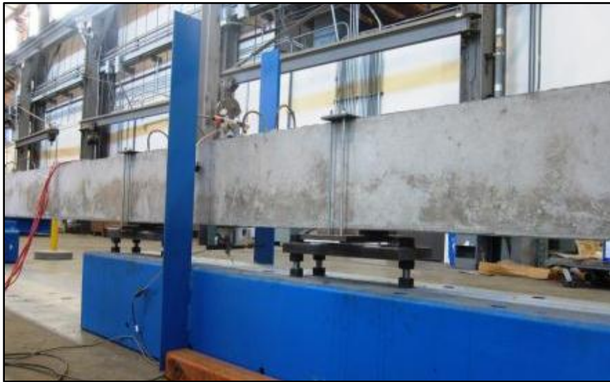
Figure 3-15: Lateral Stays at Midspan
