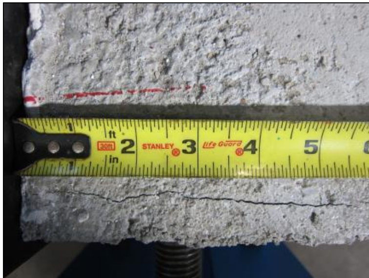
Figure 3-7: End Cracking in First Specimen
