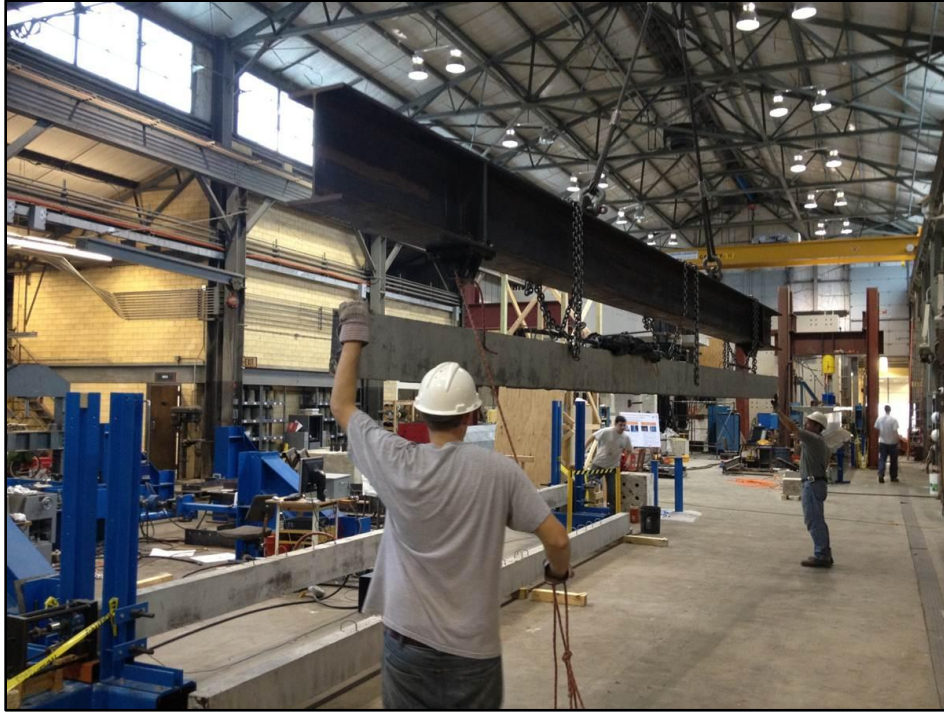
Figure 3-9: Specimen Lifting Technique
