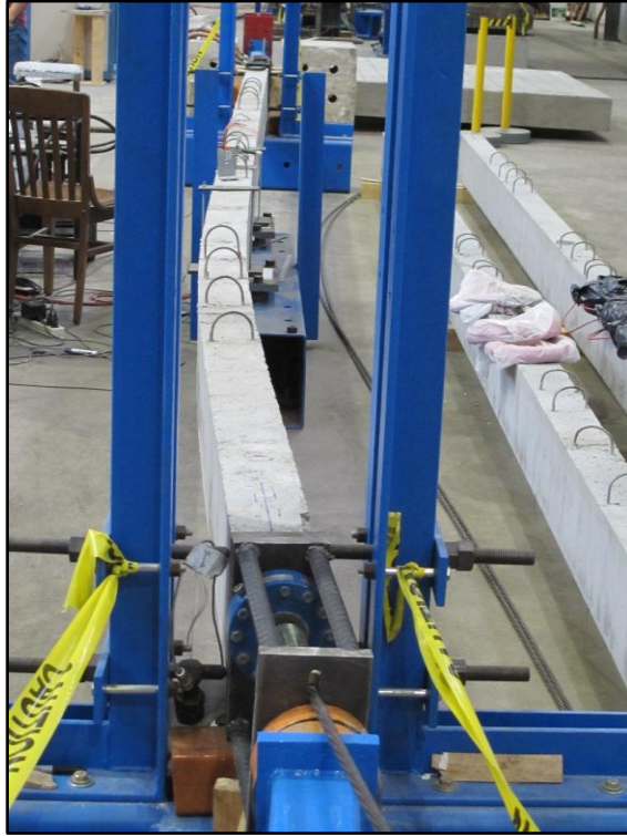
Figure 5-18: SP1 after Buckling Failure (Test SP1-PT0-EX-2)
