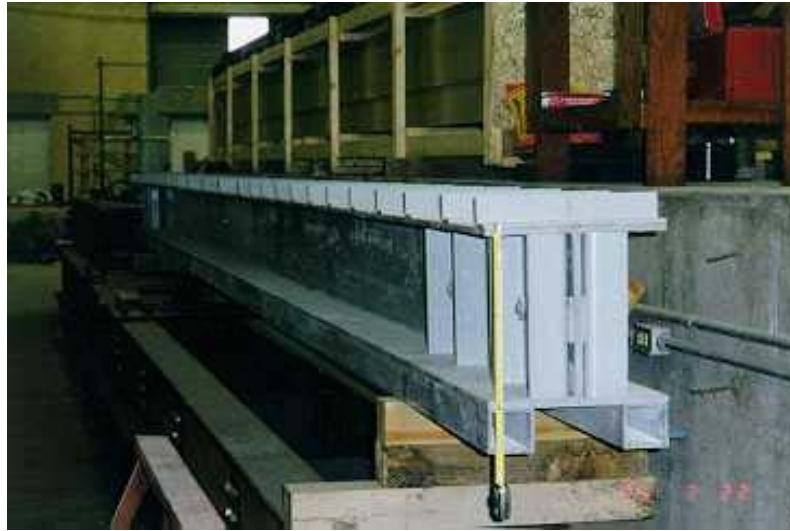
Figure 3.1: Glass Fiber Reinforced Isophthalic Polyester Pultruded Beam (FG)
