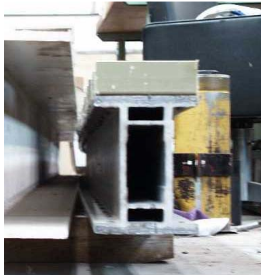
Figure 3.4: Carbon and Glass Fiber Reinforced Vinyl Ester Pultruded Beam (SW)
