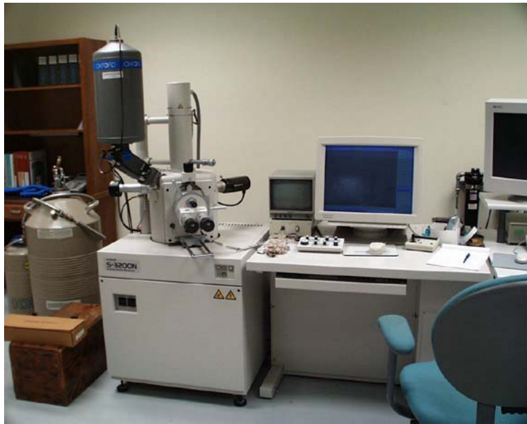
Figure 3.12: Scanning Electron Microscope, Hitachi S-3200N
