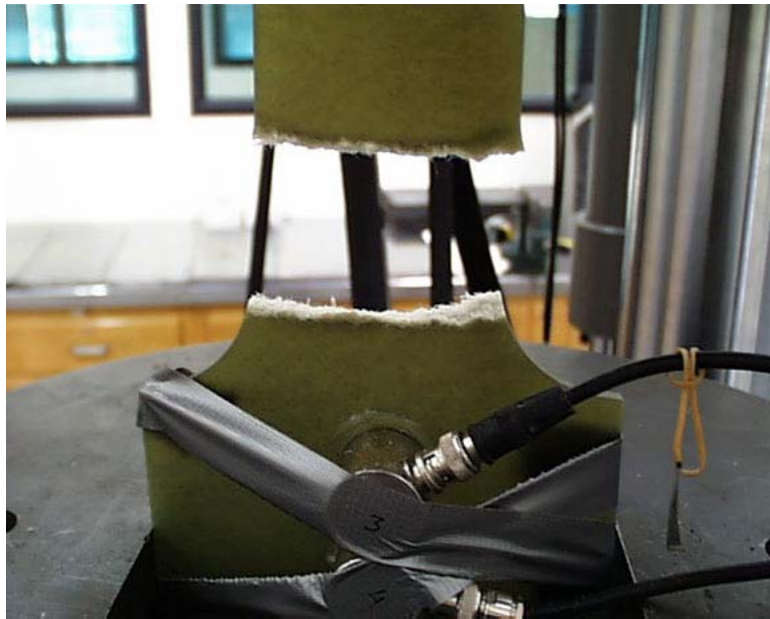
Figure 6.43: Tensile Failure of Specimen Chop
