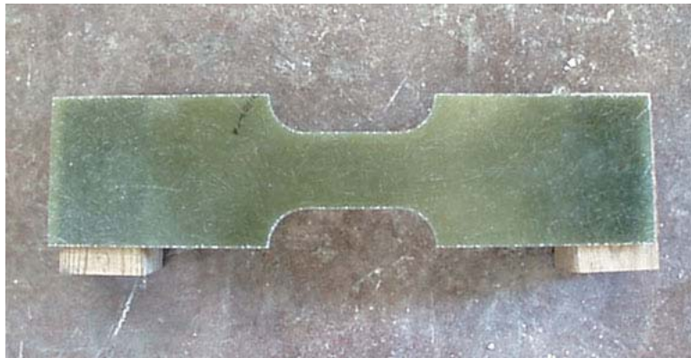
Figure 6.39: Specimen Chop (Chopped Strand Fiber Structure)
