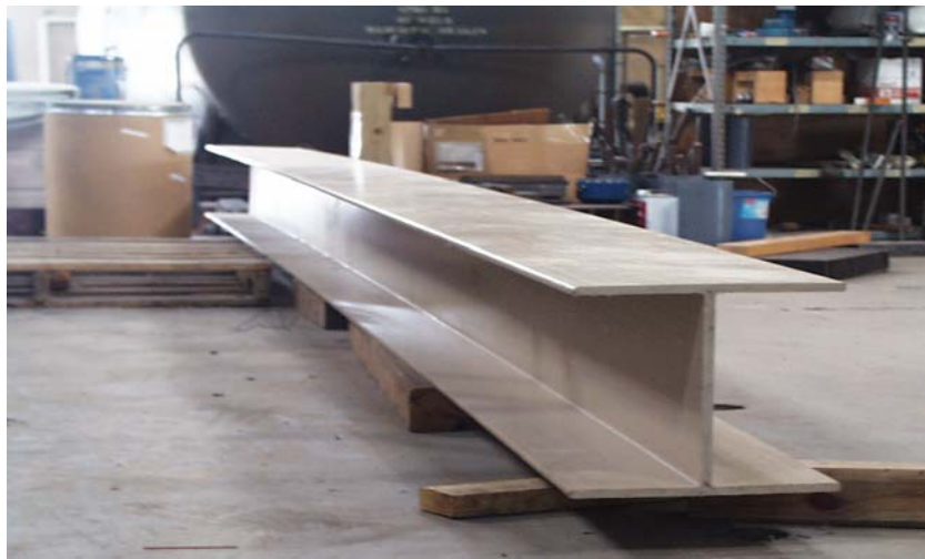
Figure 3.3: Glass Fiber Reinforced Vinyl Ester Pultruded Beam (IKG)
