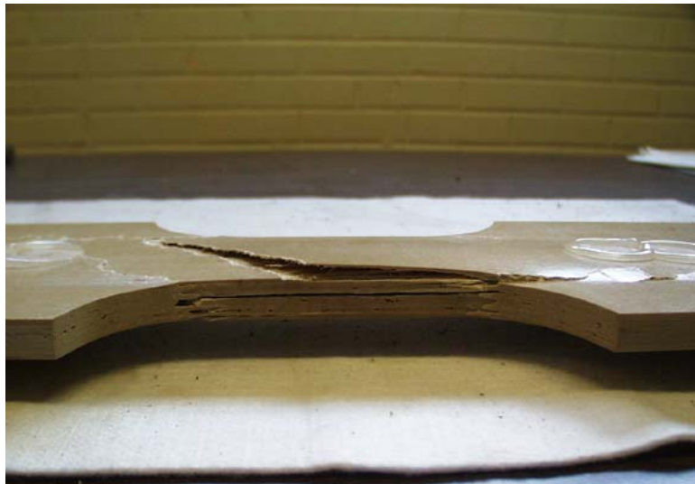
Figure 4.35: Tensile Failure and Delamination on the Side of Specimen LGVI
