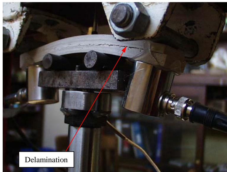
Figure 6.5: Glass/Vinyl Ester Specimen at Failure
