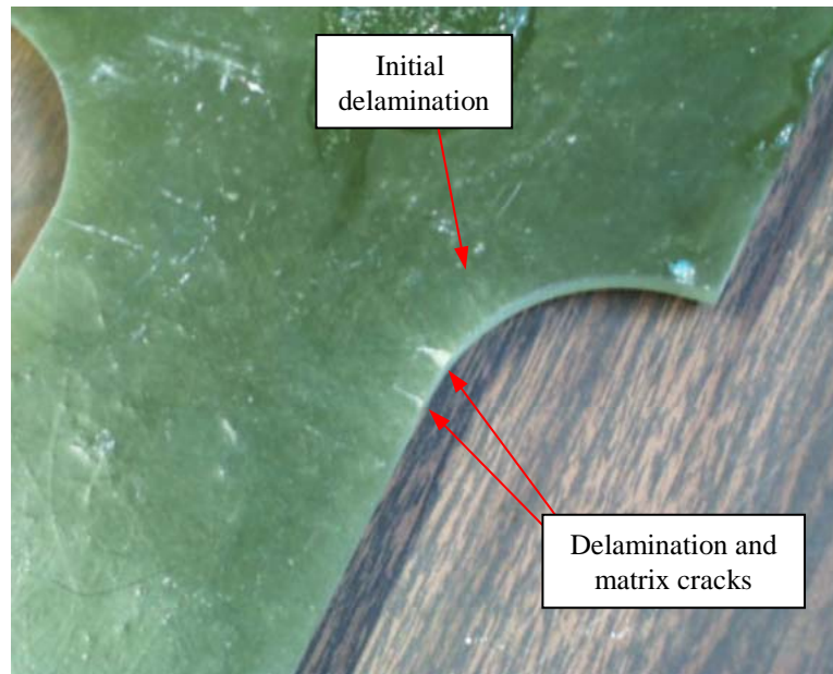
Figure 6.45: Delamination at Other End of Narrowed Section of Specimen Chop
