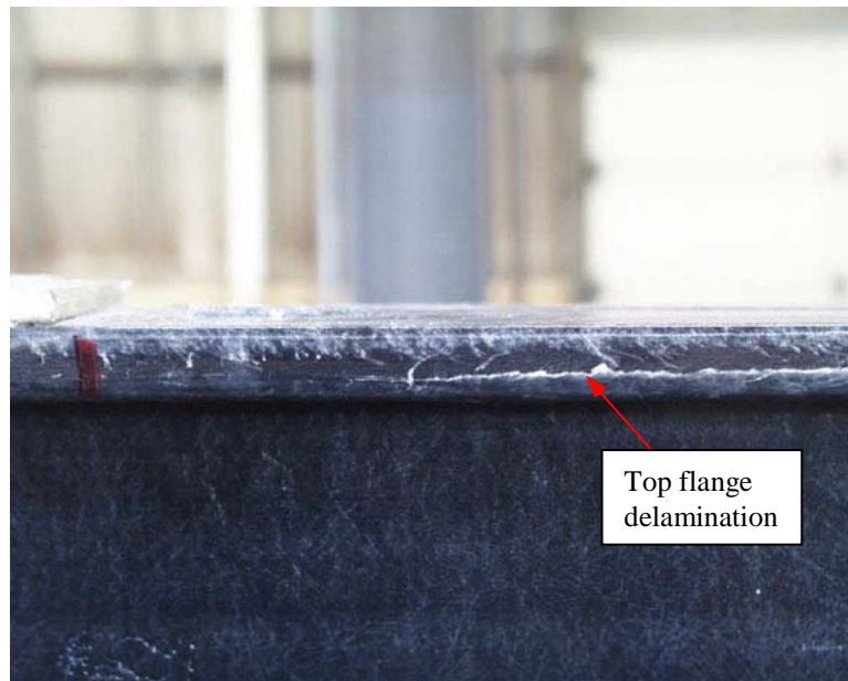
Figure 6.34: Specimen SW2 Top Flange Early Delamination (Ulloa, 2002)
