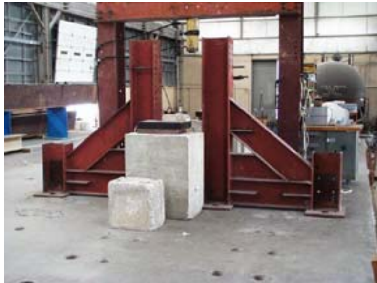
Figure 3.10: Full-Scale Loading Frame
