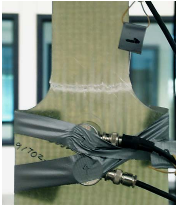
Figure 6.46: Tensile Failure of Specimen Wov
