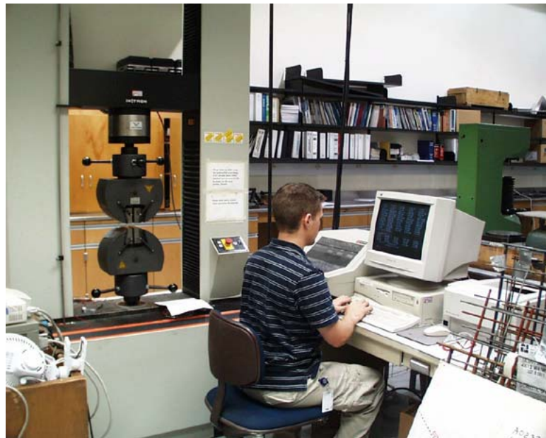
Figure 3.11: Universal Testing Machine, Instron 4208
