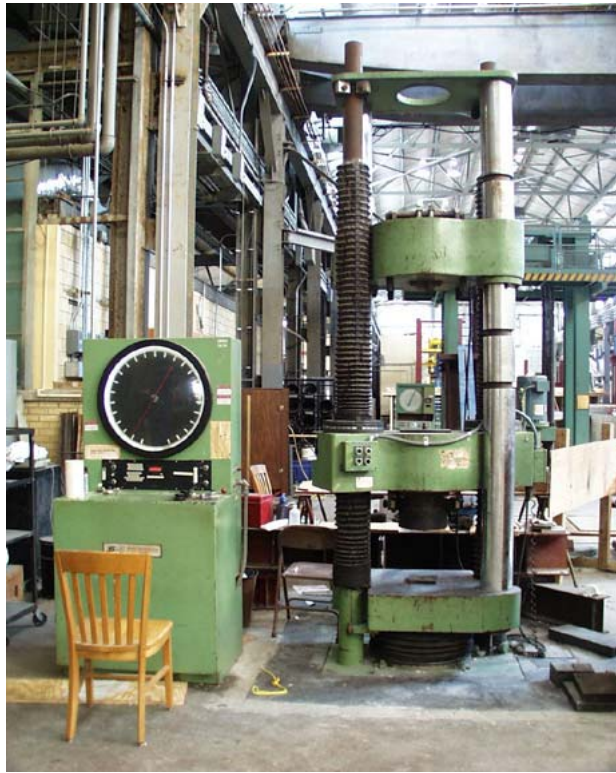
Figure 3.8: Universal Testing Machine 600HVL
