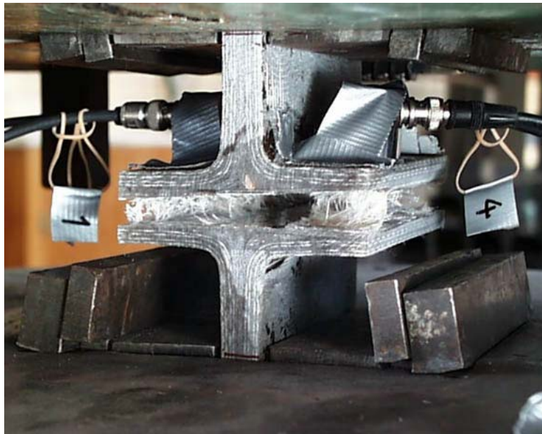
Figure 6.22: Wide Opening of the Interface Showing Fiber Bridging from Upper Portion to Lower Portion of Specimen Tee1
