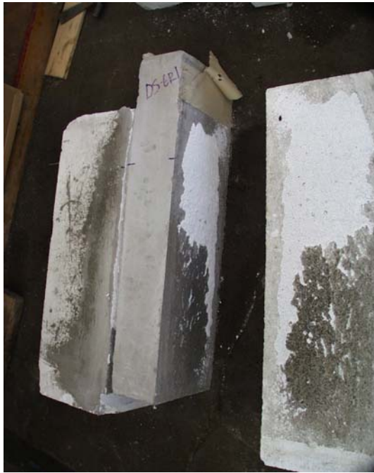
Figure D.10 Failure surface of Direct Shear Specimen DS-GR-1
