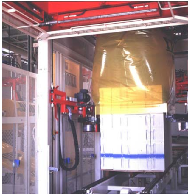
Figure B.7 Packaging of finished AAC units
