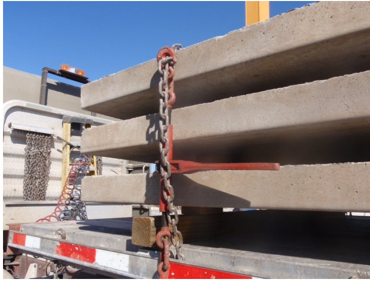
Figure 5.15 Panels strapped to flatbed truck, Plant B
