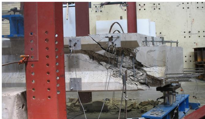
Figure 4-22: Failure of skewed end of BB-02 (Conventional Concrete).
