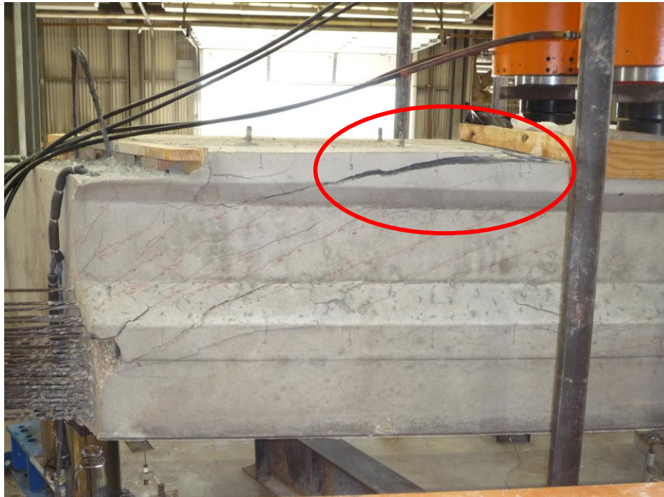
Figure 6-28: Shearing through top flange. Skewed end of 5B40-3 is shown.
