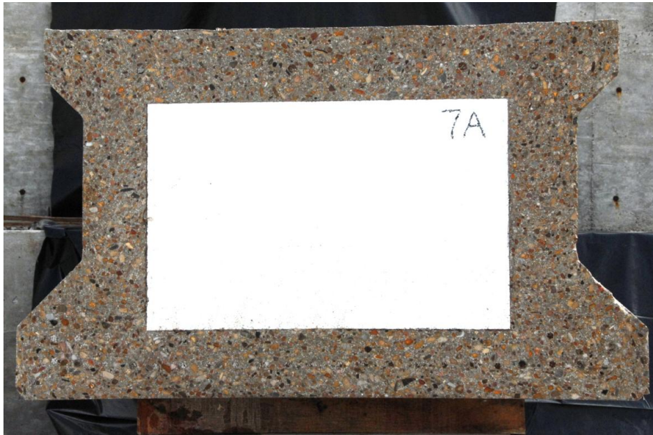
Figure 4-29: Cut section of beam fabricated with SCC and river gravel.
