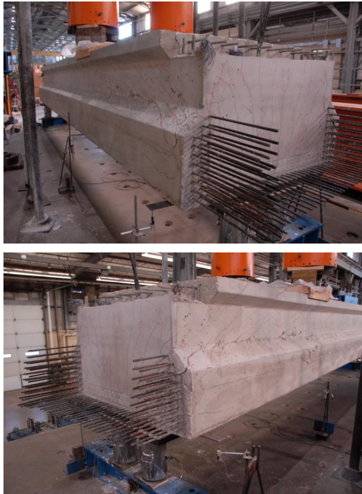
Figure 6-31: Symmetric failure of both webs in 5B40-4-Q
