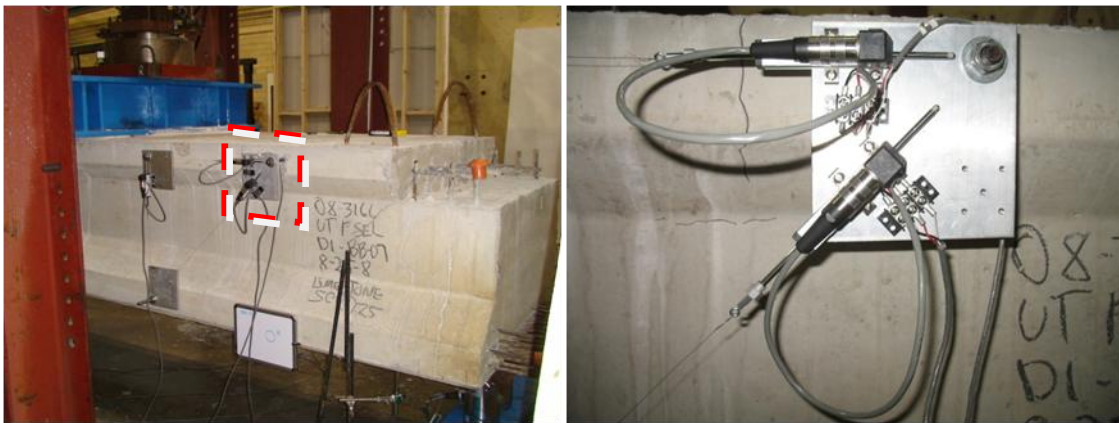
Figure 3-11: Shear deformation measurement instrumentation.
