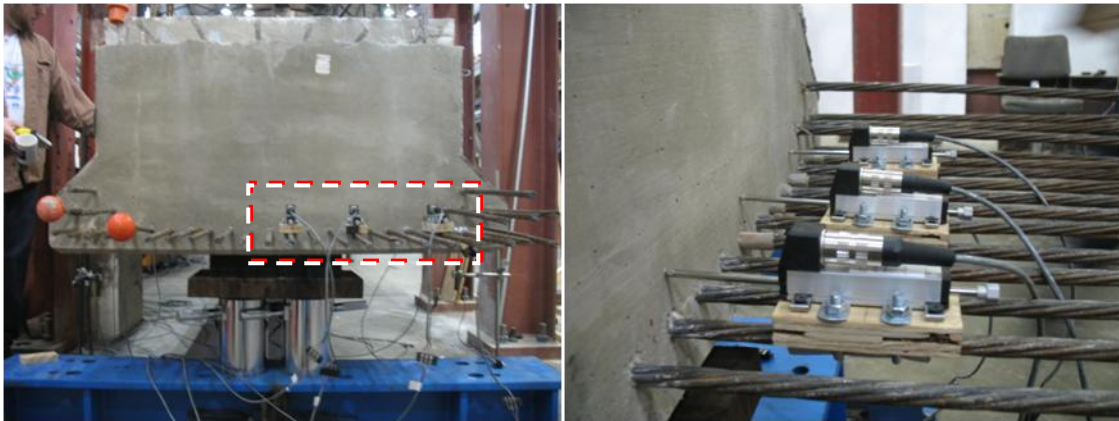
Figure 3-12: Strand slip instrumentation.
