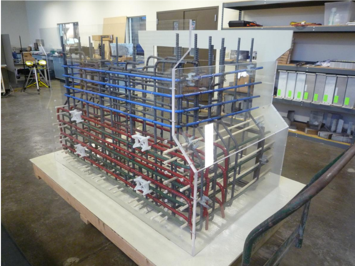
Figure 7-2: Full-scale model of the improved end-region reinforcement used in beam 5B40-4
