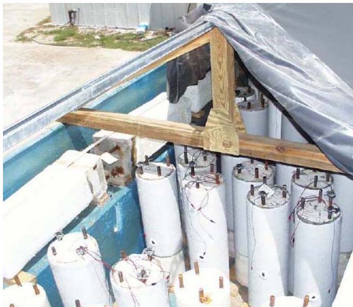
Figure 3.1 The corrosion monitoring tank and several specimens under observation for TxDOT Project 0-1774
